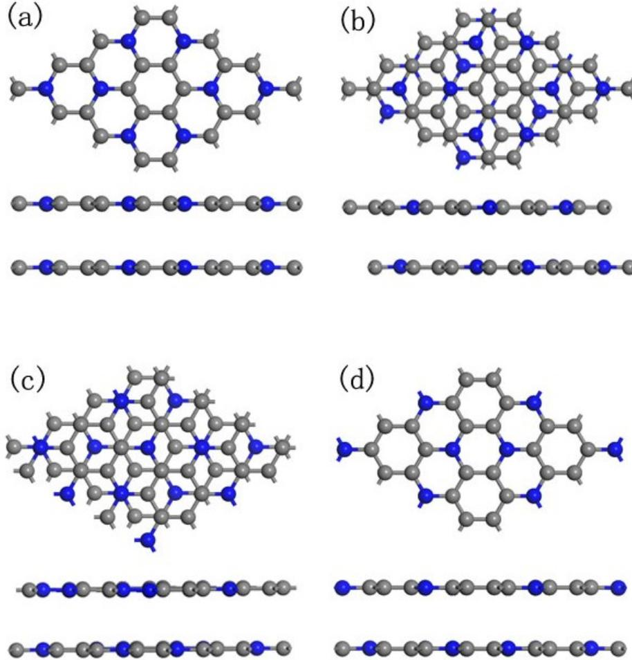
Fig. S2 Four stacking structures of C<sub>3</sub>N bilayer, (a)-(d) Top view and side view of AA-, AB-, AC-and AD-stacking, respectively. A 2×2 super cell is adopted for the view. Grey (blue) ball denotes carbon (nitrogen) atom.
