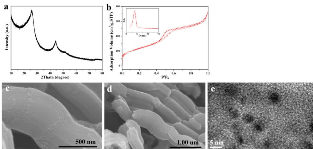
**Figure S11.** Wide-angle XRD pattern (a), N<sub>2</sub> sorption isotherms (b), SEM (c, d) and HRTEM (d) images of the representative catalyst CoN<sub>x</sub>-OMC-800 after 7 runs of catalytic reaction.
