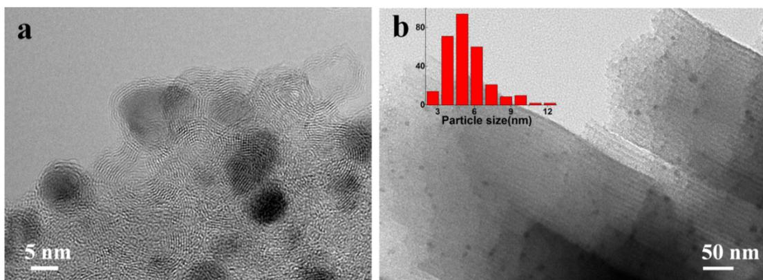
**Figure S4.** HRTEM (a) and TEM (b) images of the representative catalyst  $\text{CoN}_x\text{-OMC-800}$ . Inset (b) is the nanoparticle size distribution histogram.
