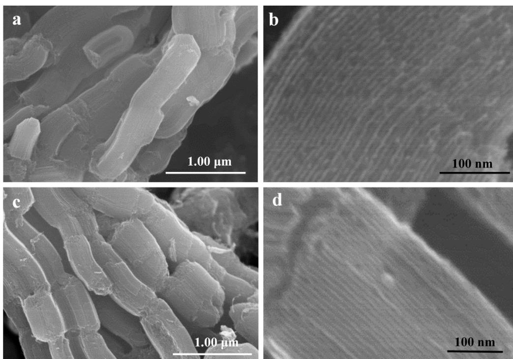
**Figure S7.** SEM (a, c) and HRSEM (b, d) images of the samples CoN<sub>x</sub>-OMC-700 (a, b) and CoN<sub>x</sub>-OMC-900 (c, d), respectively.
