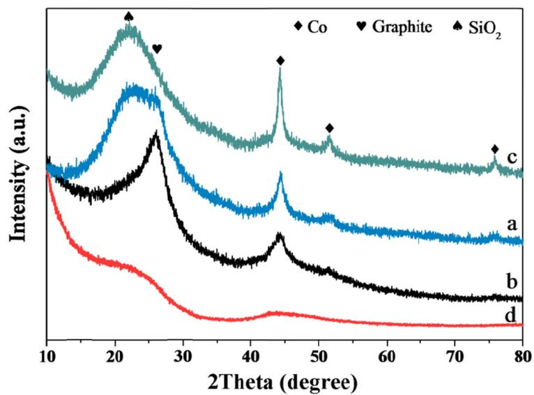
**Figure S3.** Wide-angle XRD patterns of the representative catalyst CoN<sub>x</sub>-OMC-800 (b) and the control sample Co-OMC-800 (d), and their corresponding carbonized composites before the HF acid treatment (a, c), respectively.
