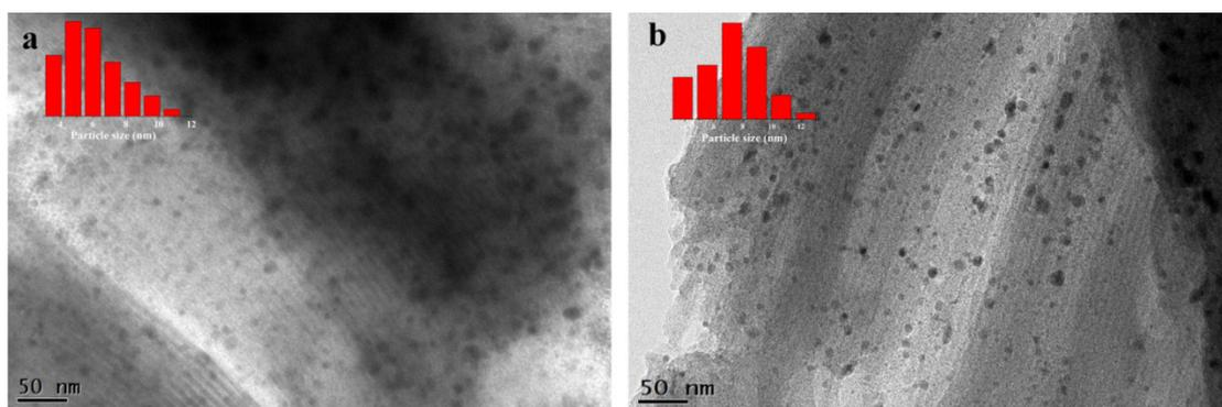
**Figure S8.** TEM images of the samples Co<sub>N<sub>x</sub></sub>-OMC-700 (a) and Co<sub>N<sub>x</sub></sub>-OMC-900 (b). Insets (a, b) are the corresponding nanoparticle size distribution histogram.
