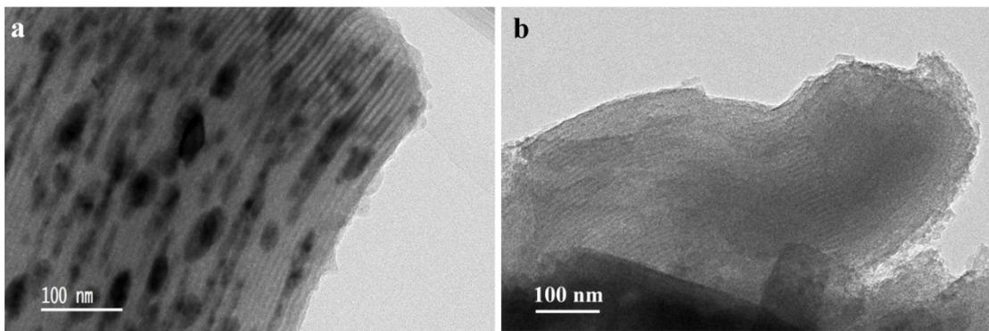
**Figure S5.** TEM images of the control sample Co-OMC-800 before (a) and (b) after the HF acid treatment.
