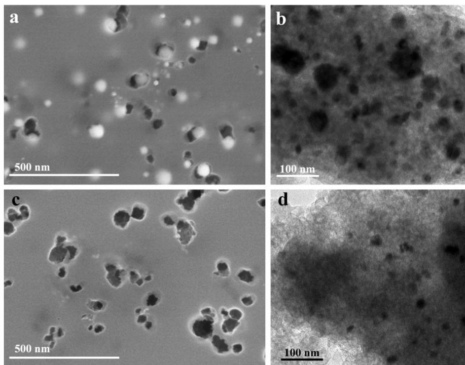
**Figure S10.** SEM (a, c) and TEM (b, d) images of the control sample  $\text{CoN}_x\text{-C-800}$  before (a, b) and after (c, d) the HF acid treatment.
