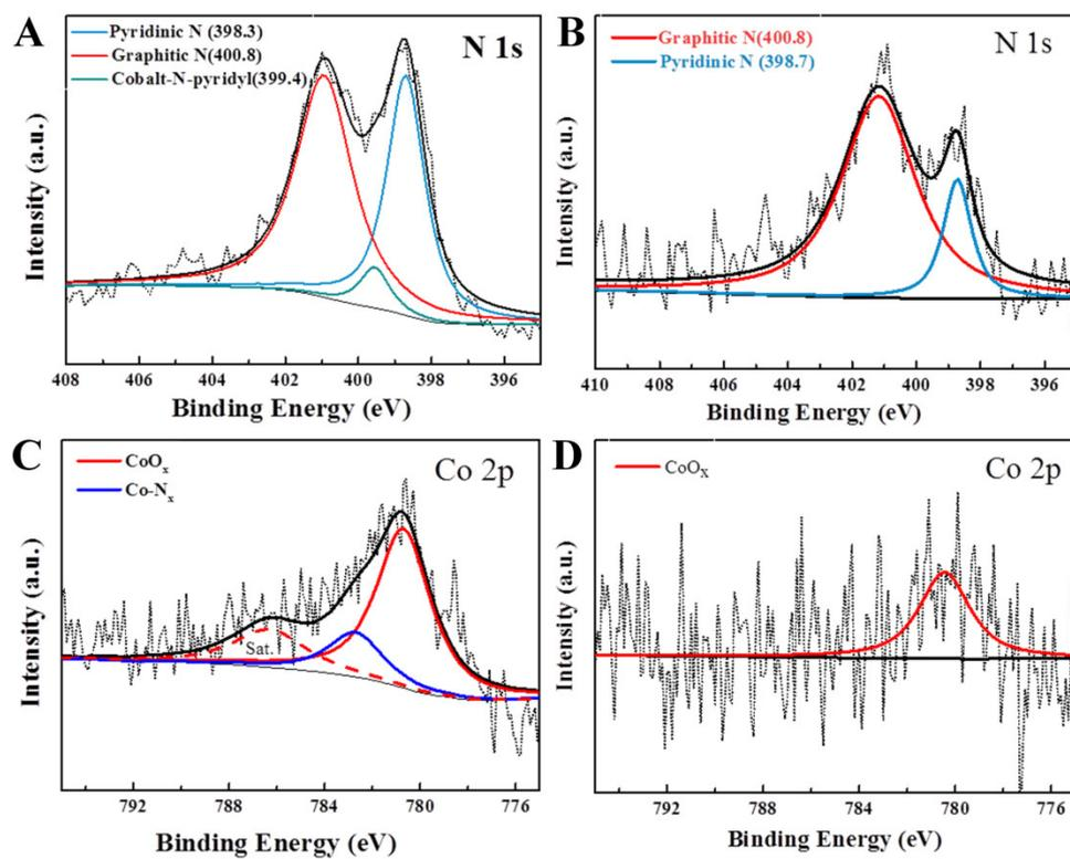
**Figure S9.** N 1s (A, B) and Co 2p (C, D) XPS spectra of the samples Co<sub>N<sub>x</sub></sub>-OMC-700 (A, C) and Co<sub>N<sub>x</sub></sub>-OMC-900 (B, D), respectively.
