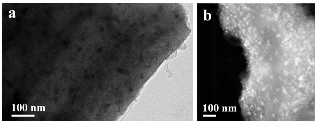
**Figure S2.** TEM (a) and STEM (b) images of the carbonized  $\text{CoN}_x\text{-OMC-800@SBA-15}$  composite before the HF treatment.
