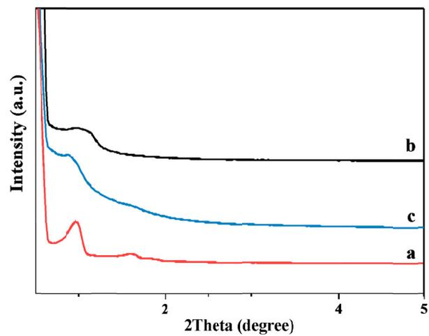
**Figure S1.** Small-angle XRD patterns of the ordered mesoporous silica SBA-15 template (a), the representative catalyst  $\text{CoN}_x\text{-OMC-800}$  (b), and the control sample  $\text{Co-OMC-800}$  (c), respectively.
