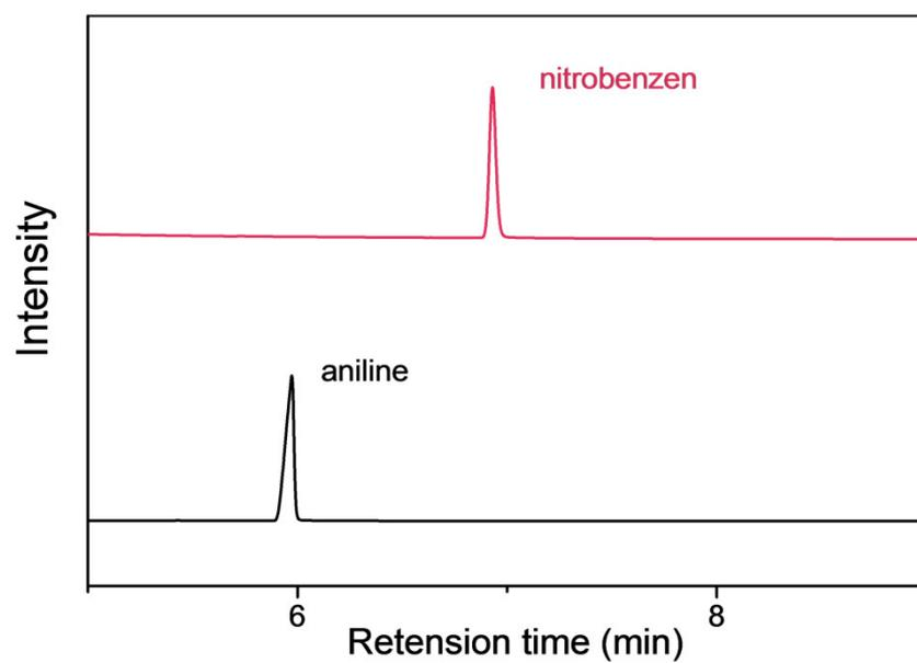
Figure S6. GC spectra of the nitrobenzene starting nitrobenzene solution (top curve) and the product (bottom curve) after the hydrogenation of nitrobenzene over the  $\text{CoN}_x$ -OMC-800 catalyst.
