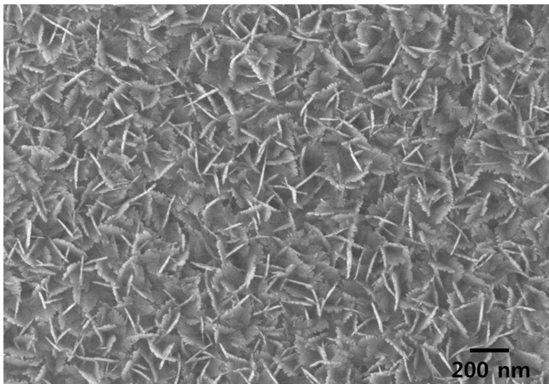
**Fig. S1.** FE-SEM top view of the aluminum hydroxide nanostructure.
