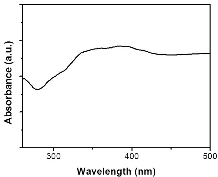
**Fig. S3.** Absorbance spectrum of the aluminum hydroxide nanostructure in the visible wavelength range, showing a small absorbance hump around 350 - 400 nm.
