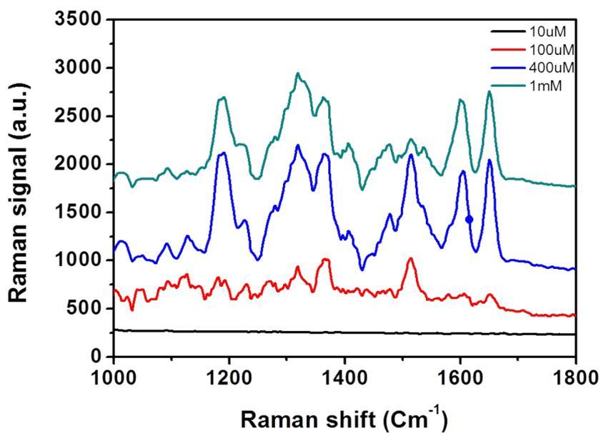
Fig. S7. SERS spectra of R6G molecules on the sample at  $t_{Ag} = 40$  nm.
