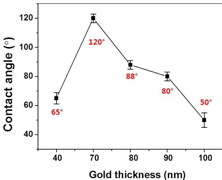
**Fig. S2.** Contact angle of gold-coated aluminum hydroxide nanostructures with respect to deposited gold thickness.
