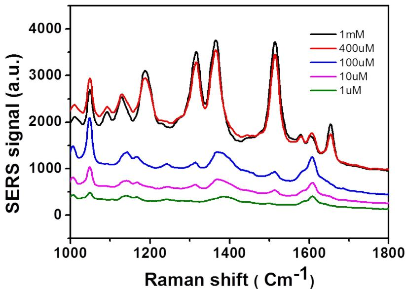
Fig. S9. SERS spectra of R6G molecules on the sample at  $t_{Ag} = 100$  nm.
