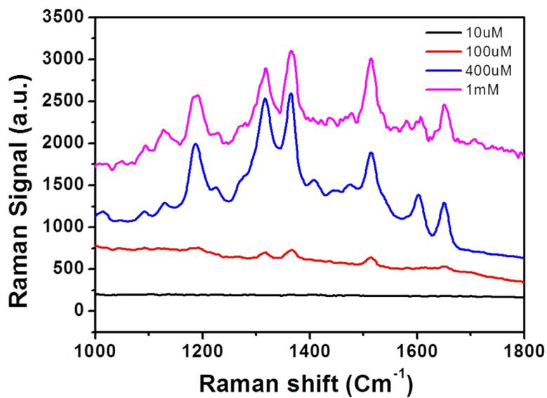
Fig. S6. SERS spectra of R6G molecules on the sample at  $t_{Ag} = 20$  nm.
