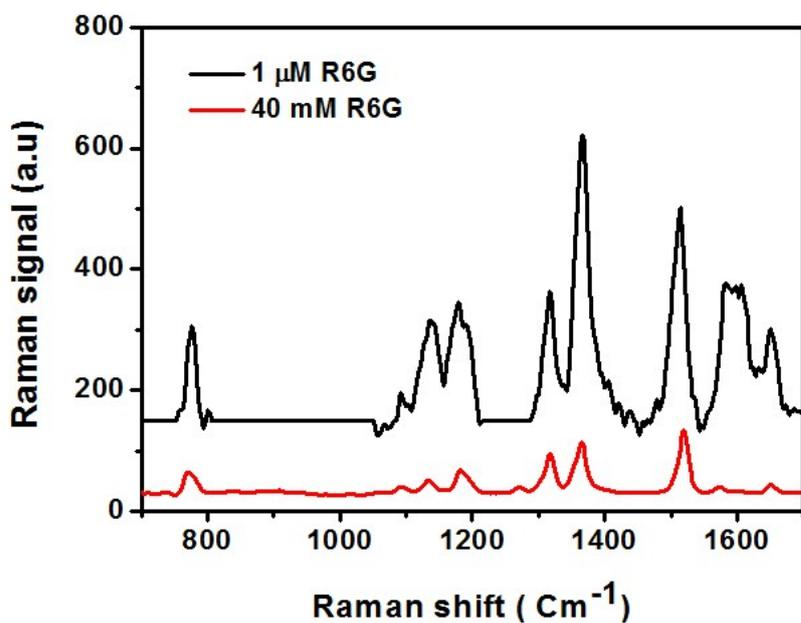
**Fig. S4.** SERS signal on our nanostructure for 1  $\mu\text{M}$  R6G and Raman signal on glass for 40 mM R6G.
