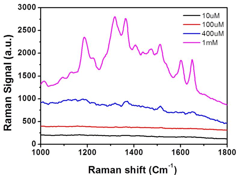
**Fig. S5.** SERS spectra of R6G molecules on the sample at  $t_{\text{Ag}} = 10$  nm.
