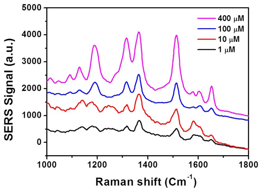
Fig. S8. SERS spectra of R6G molecules on the sample at  $t_{Ag} = 60$  nm.
