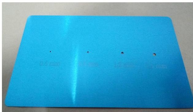
**Fig. S11.** The template used to precisely control the size of the ink dots, which was obtained by laser processing (the diameters were 0.6 mm, 0.9 mm 1.2mm and 1.5 mm, respectively).
