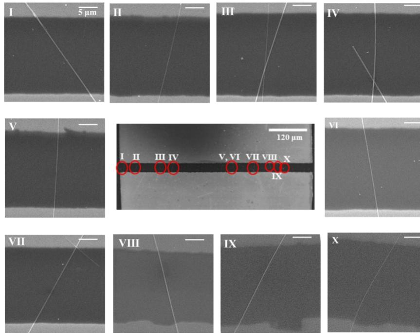
**Fig. S3.** SEM images of the 10 PSi NWs spanning the Al electrodes.
