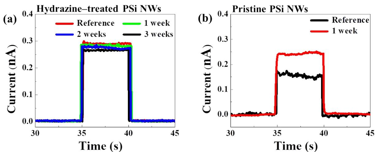
**Fig. S7.** Environmental stability test of the photo-sensing device composed of (a) hydrazine-treated PSi NWs and (b) pristine PSi NWs as reflected in the changes in the photocurrent upon exposure to ambient air up to three weeks (with illumination of visible lights of the wavelengths of 424 nm).
