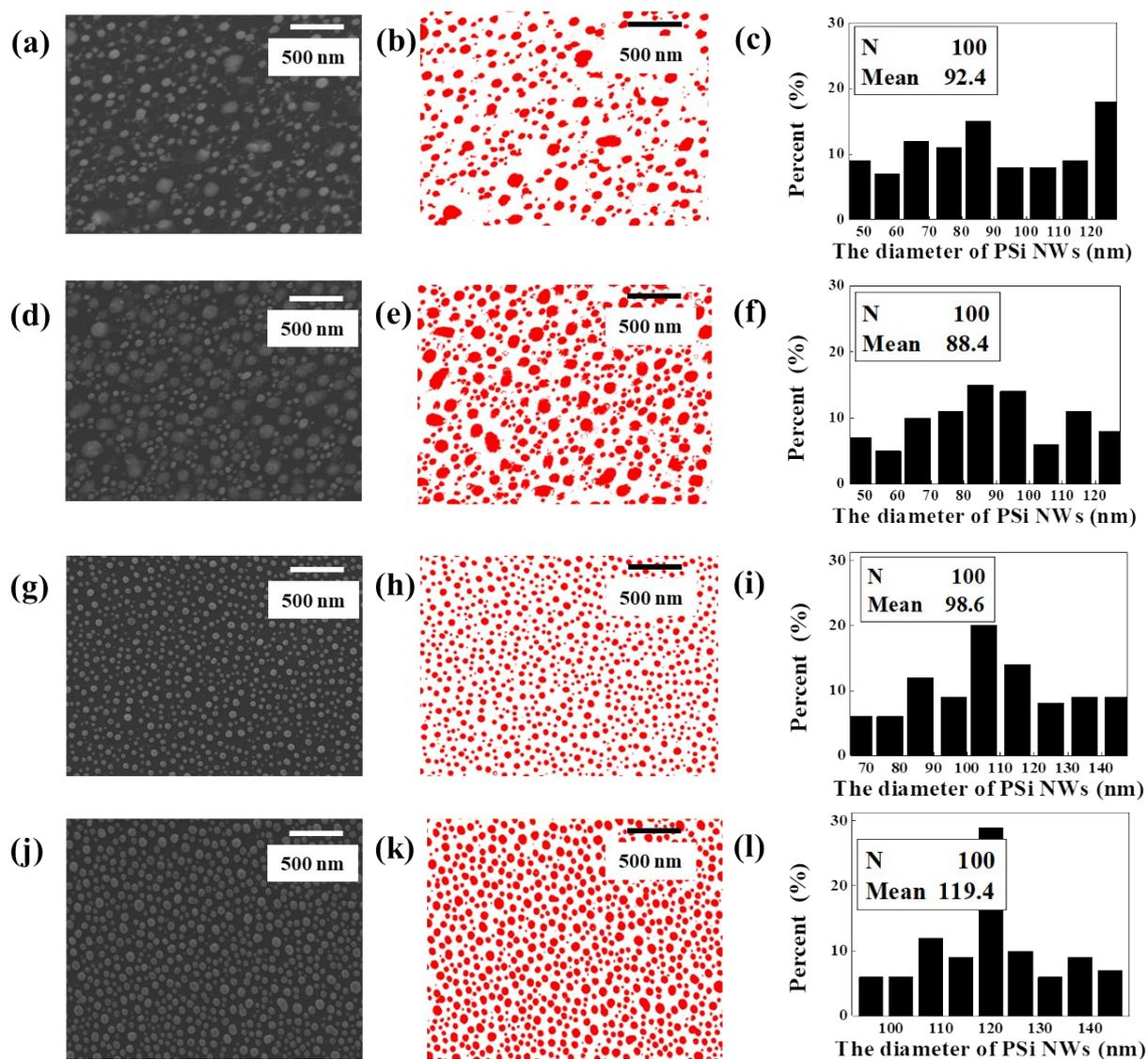
**Fig. S2.** SEM images of the Ag mesh generated by RTA with (a) 4, (d) 6, (g) 8, and (j) 10 nm thick Ag films; corresponding image analysis patterns with (b) 4, (e) 6, (h) 8, and (k) 10 nm thick Ag films; and size distributions of the Ag NPs generated by RTA with (c) 4, (f) 6, (i) 8, and (l) 10 nm thick Ag films.
