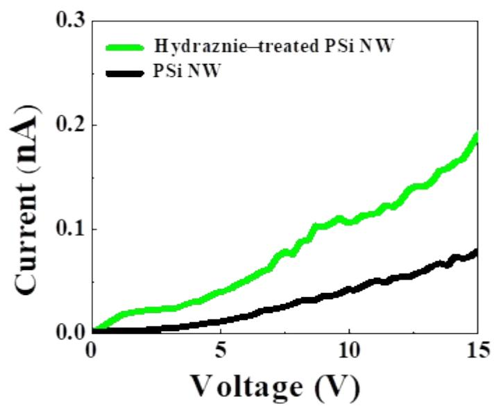
**Fig. S5.** *I-V* behaviors of pristine PSi NW and hydrazine-treated PSi NW.
