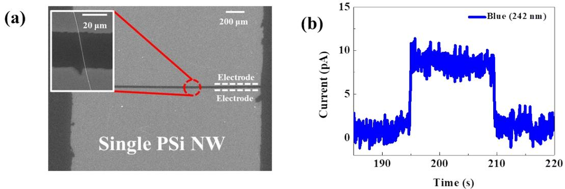
**Fig. S6.** (a) SEM image of the single PSi NW spanning the Al electrodes. (b) Photocurrent through the photo-sensing device composed of single PSi NW with illumination of visible light of the wavelength of 424 nm (blue).
