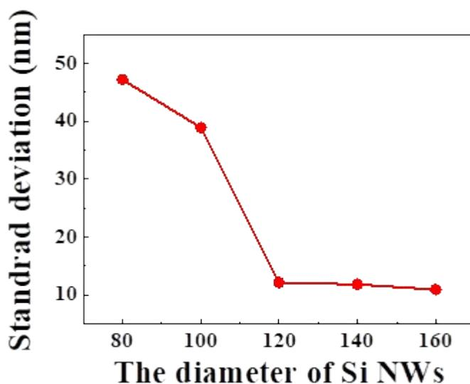
**Fig. S1.** Standard deviation of Si NWs' diameter.
