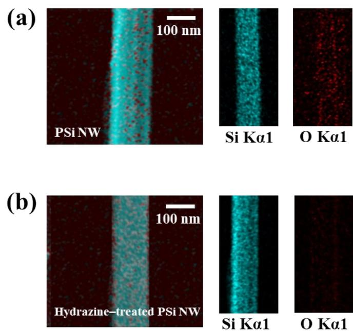
**Fig. S4.** TEM-EDS element mapping images of (a) pristine PSi NW and (b) hydrazine-treated PSi NW.
