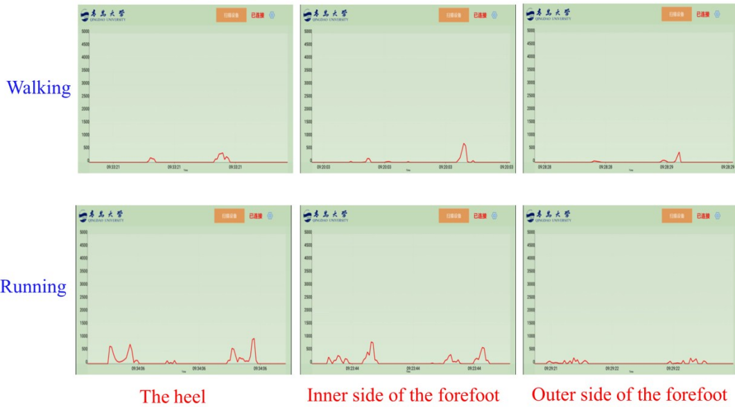
Fig. S7 Piezoelectric signals of volunteer No. 2. The part where the habitual abrasion occurs of their shoes is under inner side of the forefoot.
