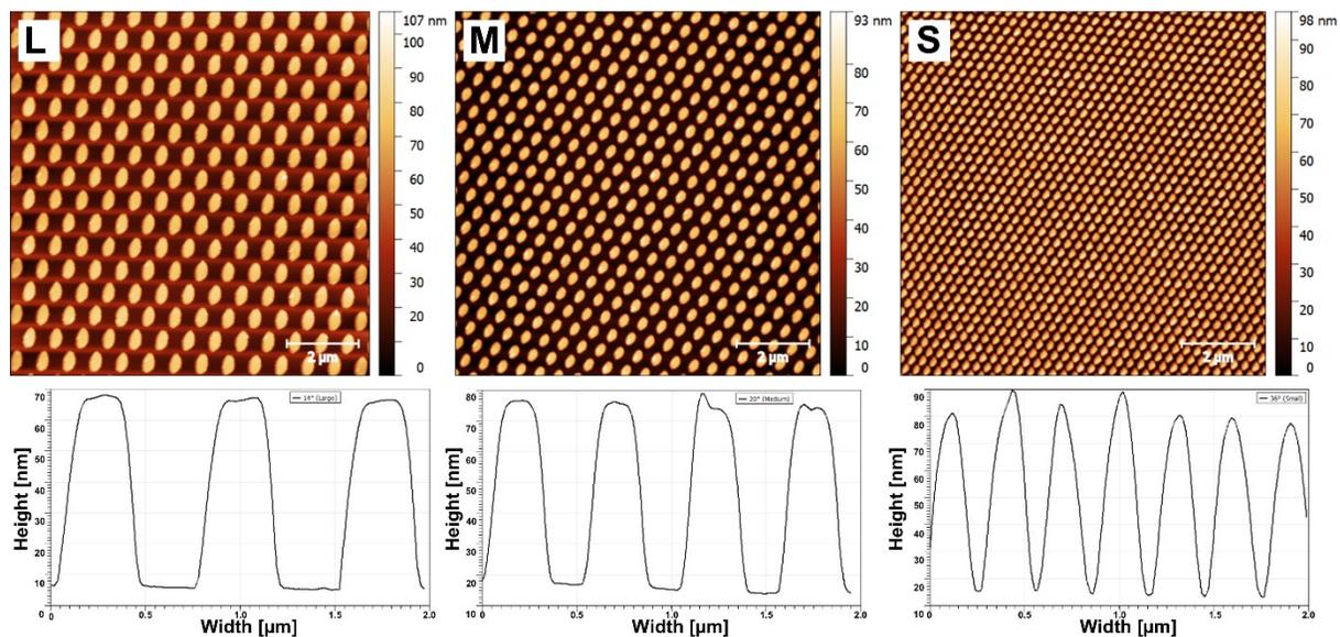
**Figure S1.** AFM analysis of hexagonally arranged, unmodified nanostructures of different feature dimensions obtained using three-beam laser interference lithography (LIL) at different angles of incidence (large (L) = 14°, medium (M) = 20°, and small (S) = 36°). The height profiles show the progression of structures in lateral dimension. [Scale: 2 μm]
