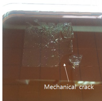
PMMA /graphene layer on copper etchant
