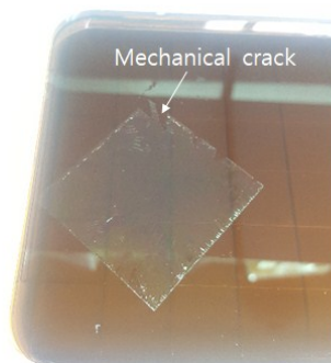
PS /graphene layer on copper etchant
