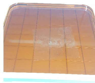
PS+DIPB /graphene layer on copper etchant
