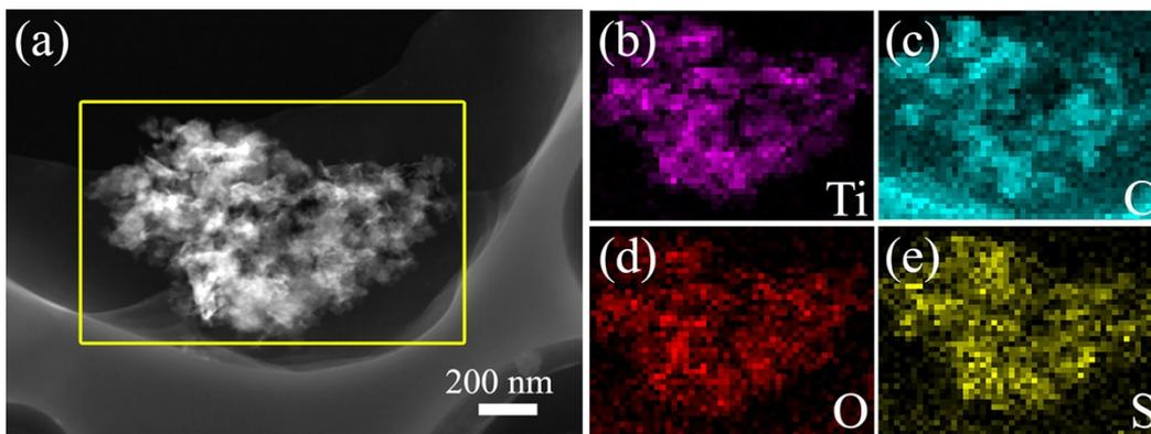
**Fig. S2** (a) TEM image of a S/Ti<sub>3</sub>C<sub>2</sub>T<sub>x</sub> nanoflake composite, and (b-e) the corresponding elemental mapping images of Ti, C, O, and S, respectively.
