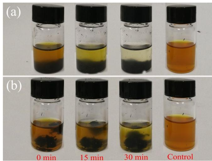
**Fig. S5** Digital Photos of (a) the  $\text{Ti}_3\text{C}_2\text{T}_x$  powder and (b) the SWCNT powder soaked in  $\text{Li}_2\text{S}_6$  (0.02 M) solution, respectively.
