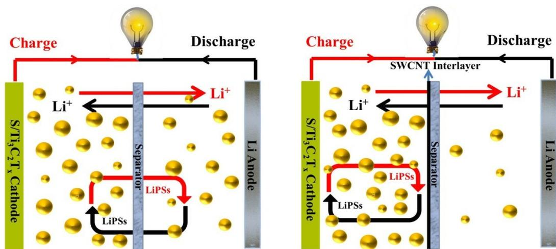
Fig. S6 Schematic configuration of the S/Ti<sub>3</sub>C<sub>2</sub>T<sub>x</sub> and S/Ti<sub>3</sub>C<sub>2</sub>T<sub>x</sub>-I cells.
