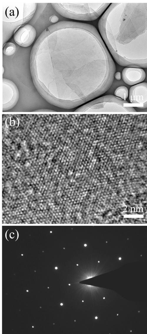
**Fig.S1** (a)TEM image take from the as-synthesized  $\text{Ti}_3\text{C}_2\text{T}_x$  nanoflake. (b) HRTEM image of a  $\text{Ti}_3\text{C}_2\text{T}_x$  nanoflake. (c) SAED pattern of the  $\text{Ti}_3\text{C}_2\text{T}_x$  nanoflake.
