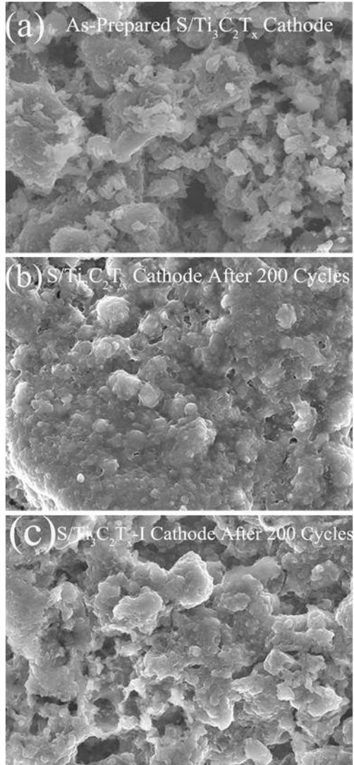
**Fig. S4** SEM images of (a) the as-prepared S/Ti<sub>3</sub>C<sub>2</sub>T<sub>x</sub> electrode, (b) the S/Ti<sub>3</sub>C<sub>2</sub>T<sub>x</sub>, and (c) the S/Ti<sub>3</sub>C<sub>2</sub>T<sub>x</sub>-I electrodes at fully charged state at 0.5 A g<sup>-1</sup> after 200 cycles.
