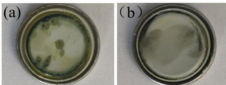
**Fig. S3** Digital photos of the separator surfaces closing to the anode for (a) the  $S/Ti_3C_2T_x$  and (b) the  $S/Ti_3C_2T_x-I$  cells.
