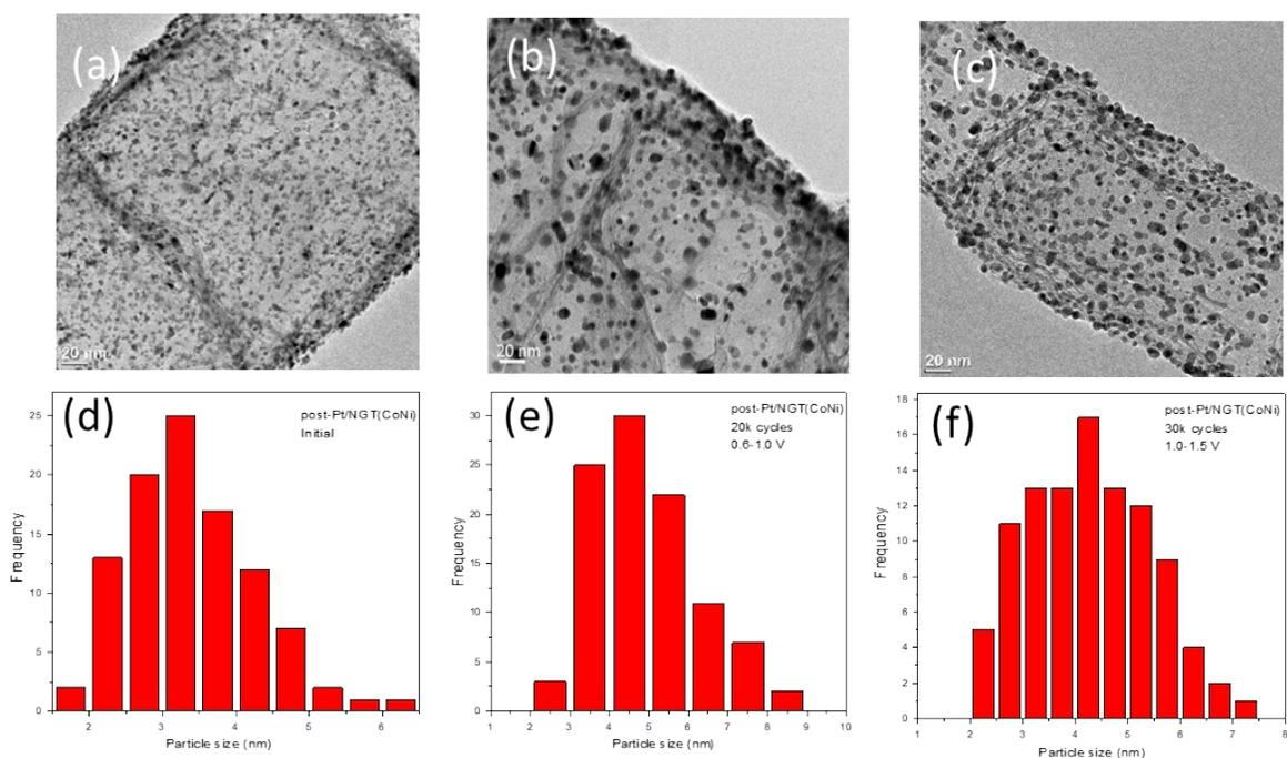
**Figure S16.** TEM images of (a) fresh post-Pt/NGT(CoNi), (b) post-Pt/NGT(CoNi) after 20k cycles from 0.6-1.0 V vs RHE, and (c) post-Pt/NGT(CoNi) after 30k cycles from 1.0-1.5 V vs RHE. Particle size distribution of (d) fresh post-Pt/NGT(CoNi), (e) post-Pt/NGT(CoNi) after 20k cycles from 0.6-1.0 V vs. RHE, and (f) post-Pt/NGT(CoNi) after 30k cycles from 1.0-1.5 V vs RHE.
