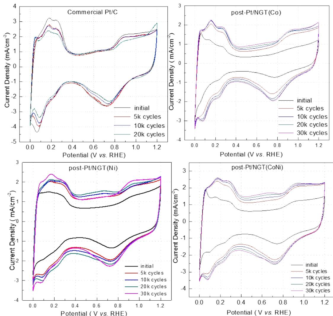
**Figure S6.** Cyclic voltammetry plots for different Pt cathode catalysts during ASTs. Potential cycling range from 1.0 to 1.5 V at a scan rate of 500 mV/s in 0.1 M HClO<sub>4</sub> at room temperature.
