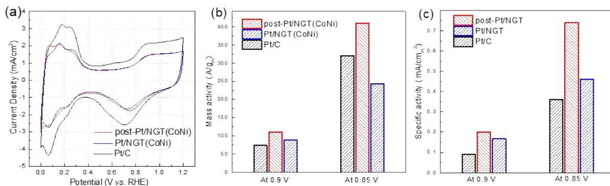
**Figure S14.** (a) cyclic voltammetry recorded in N<sub>2</sub> for commercial Pt/C, Pt/NGT(CoNi), and post-Pt/NGT(CoNi) in N<sub>2</sub>-saturated 0.1 M HClO<sub>4</sub> at room temperature. (b) Comparison of mass activities for commercial Pt/C, Pt/NGT(CoNi), and post-Pt/NGT(CoNi) at 0.85 and 0.9 V. (d) Comparison of specific activities for commercial Pt/C, Pt/NGT(CoNi), and post-Pt/NGT(CoNi) at 0.85 and 0.9 V.
