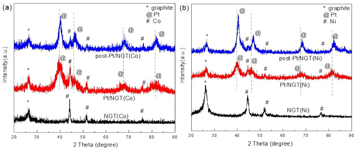
**Figure S9.** XRD spectra of (a) Co-derived NGT or catalysts and (b) Ni-derived NGT or catalysts.
