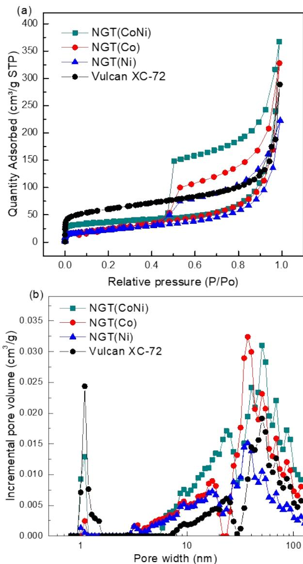
**Figure S1.** N<sub>2</sub> adsorption/desorption plots (a) and pore size distribution (b) of different carbon supports.
