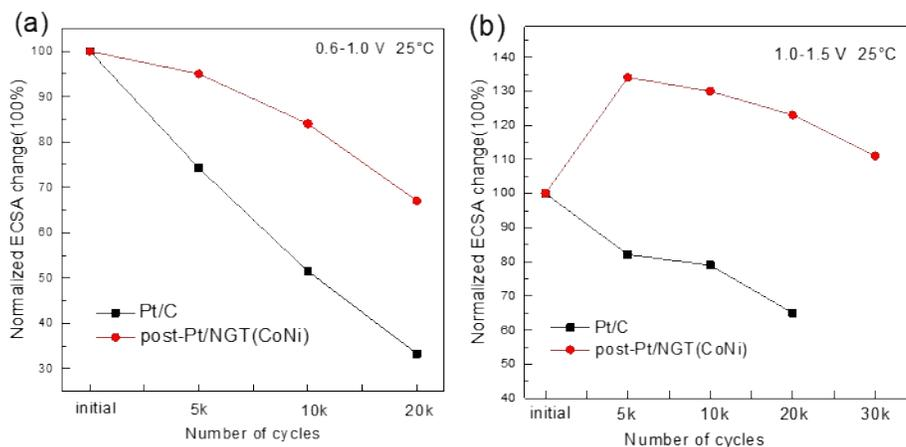
**Figure S18.** Comparison of normalized ECSA plot as a function of the AST cycling numbers between commercial Pt/C and post-Pt/NGT(CoNi).
