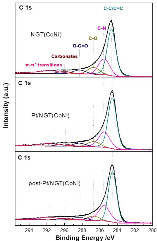
**Figure S10.** High resolution C 1s XPS spectra of NGT(CoNi), Pt/NGT(CoNi), and post-Pt/NGT(CoNi).
