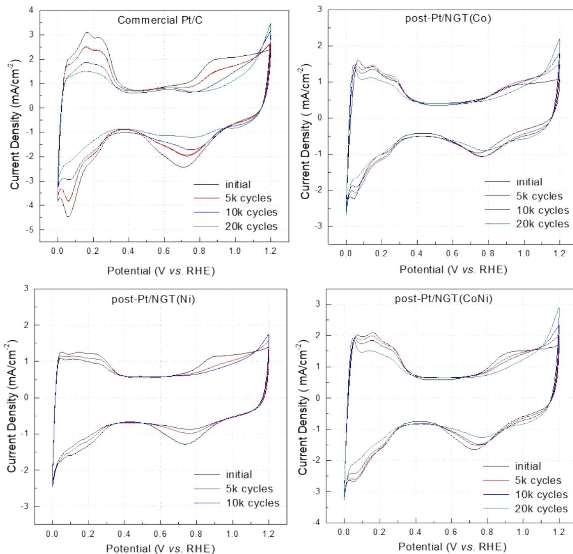
**Figure S5.** Cyclic voltammetry plots for different Pt cathode catalysts during ASTs. Potential cycling range from 0.6 to 1.0 V at a scan rate of 100 mV/s in 0.1 M HClO<sub>4</sub> at room temperature.
