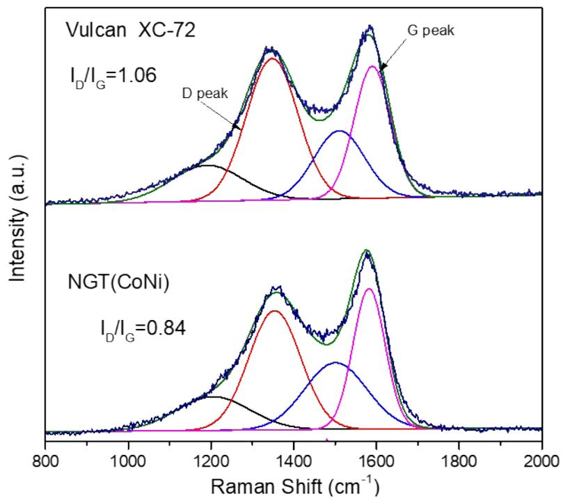
**Figure S20.** Raman patterns of Vulcan XC-72 and NGT(CoNi) supports.
