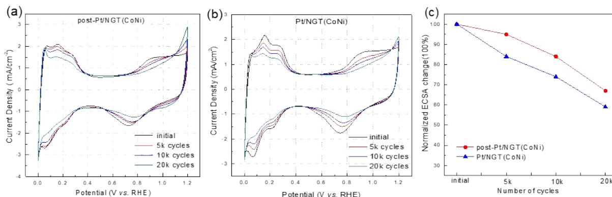
**Figure S15.** Cyclic voltammetry plots for (a) Pt/NGT(CoNi) and (b) post-Pt/NGT(CoNi) during AST test. Potential cycling range from 0.6 to 1.0 V at a scan rate of 100 mV/s in 0.1 M HClO<sub>4</sub> at room temperature. (c) Corresponding normalized ECSA plot as a function of the AST cycling numbers.
