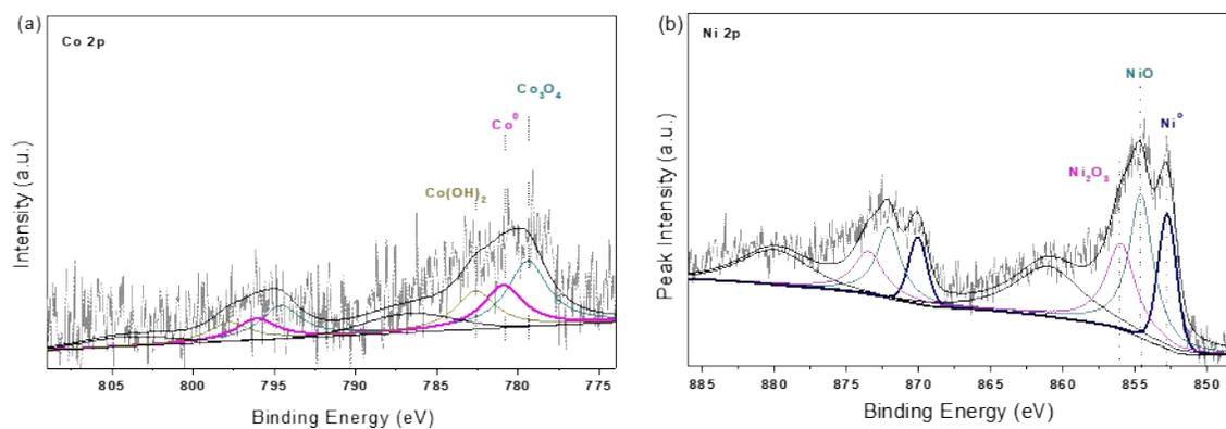
**Figure S11.** High resolution (a) Co 2p and (b) Ni 2p XPS spectra of post-Pt/NGT(CoNi).
