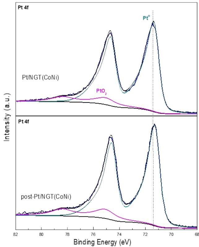
**Figure S8.** Pt 4f XPS spectra of Pt/NGT(CoNi) and post-Pt/NGT(CoNi).
