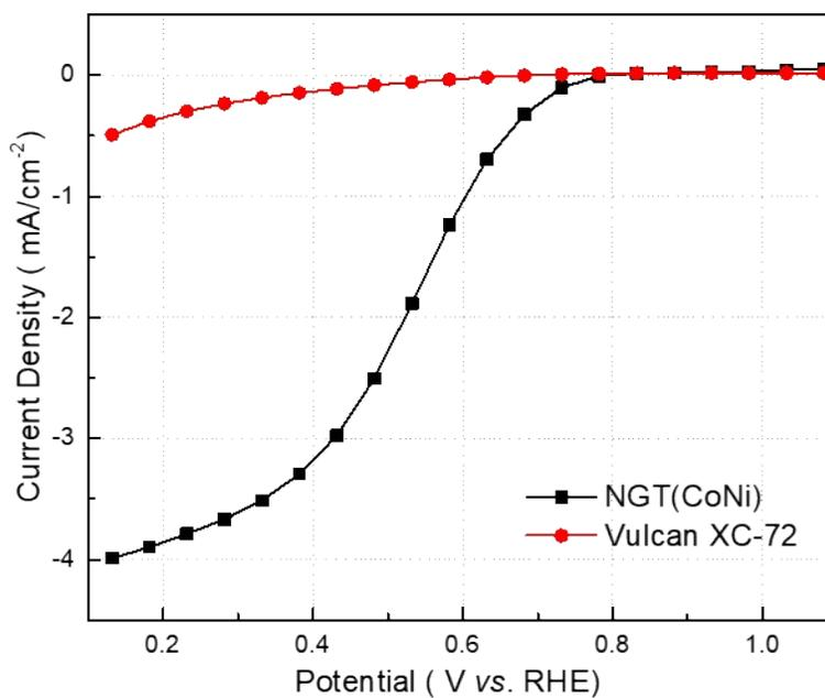
**Figure S13.** Steady-state polarization plots for NGT(CoNi) and Vulcan XC-72 in 0.1 M  $\text{HClO}_4$ .
