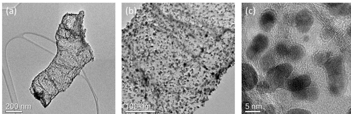
**Figure S19.** TEM images (a, b) and HR-TEM image (c) of post-Pt/NGT(CoNi) after 10,000 cycles from 1.0-1.5 V vs RHE at 60 °C.
