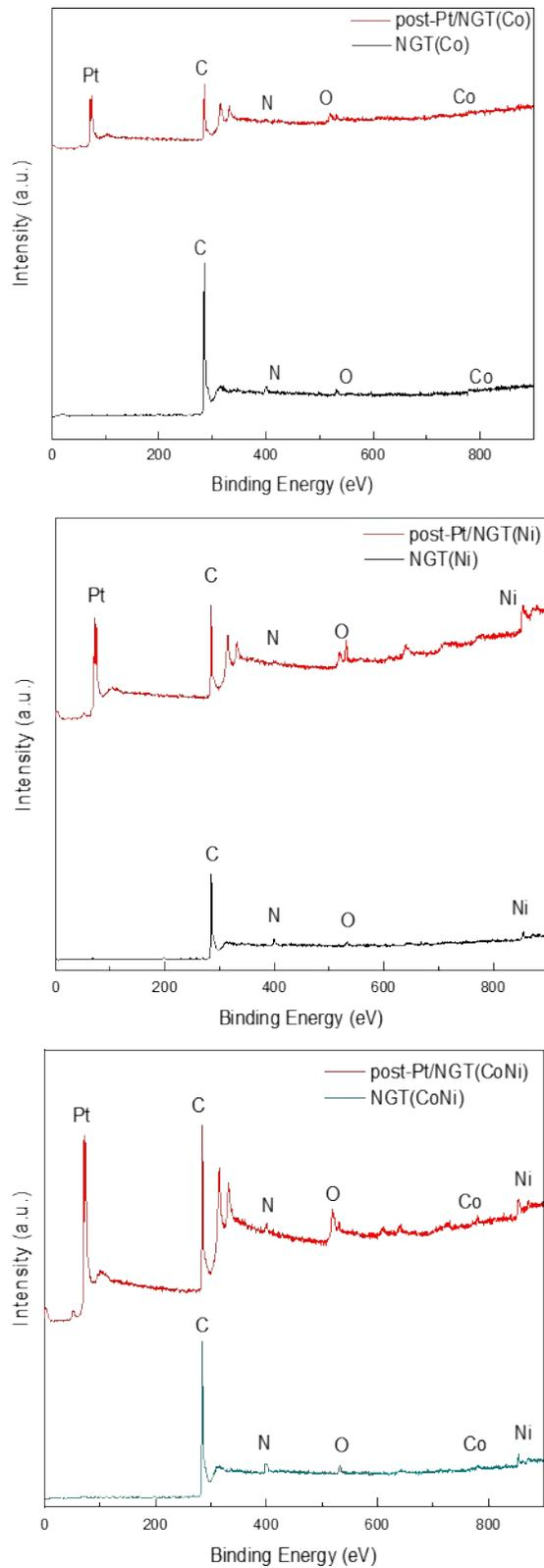
**Figure S3.** XPS survey spectra for different NGT supports and post-Pt/NGTs.
