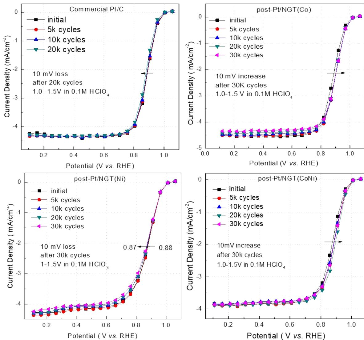
**Figure S7.** Steady-state polarization plots for different Pt cathode catalysts with rotation rate of 900 rpm during ASTs. Potential cycling range from 1.0 to 1.5 V at a scan rate of 500 mV/s in 0.1 M HClO<sub>4</sub> at room temperature.
