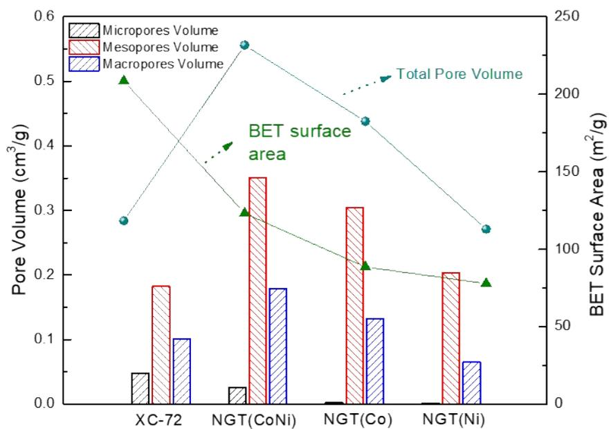
**Figure S2.** Comprehensive comparison of BET surface areas and porosity for various carbon supports.
