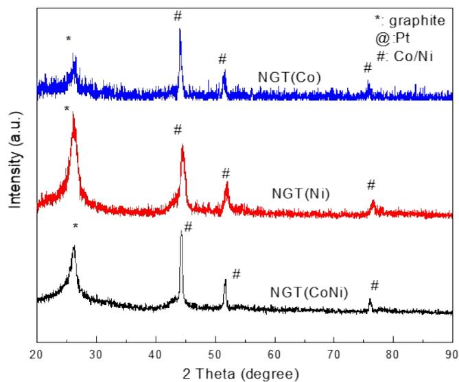
**Figure S4.** XRD patterns for various graphene tube supports.
