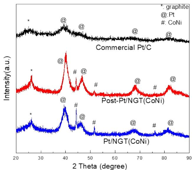
**Figure S17.** XRD spectra of different Pt cathode catalysts.
