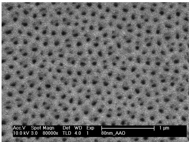
Figure 3 SEM image of the bare AAO membrane
