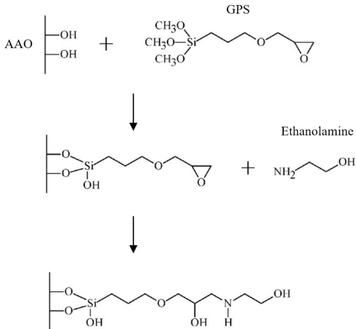
Figure 8 Immobilization of ethanolamine onto the AAO with 3-glycidoxypropyl-trimethoxysilane (GPS)
