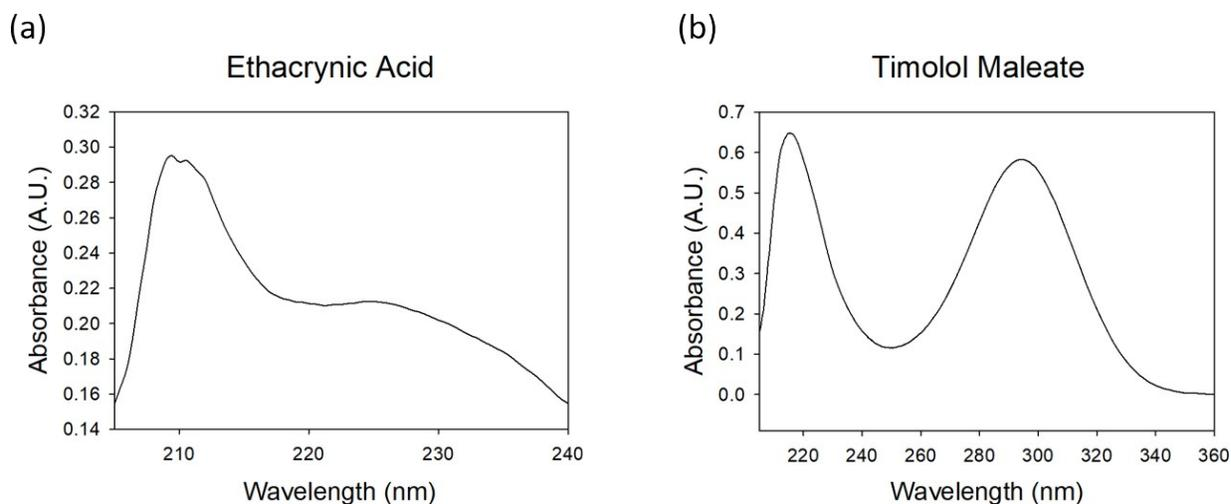
Figure 2 UV absorbance spectrum of (a) Ethacrynic acid (0.015mg/mL) and (b) Timolol maleate (0.1mg/mL) in 0.01x PBS solution
