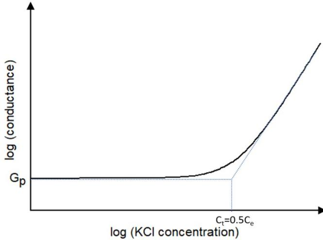
Figure 6 Schematic behavior of the nanochannel conductance as a function of the KCl concentration.
