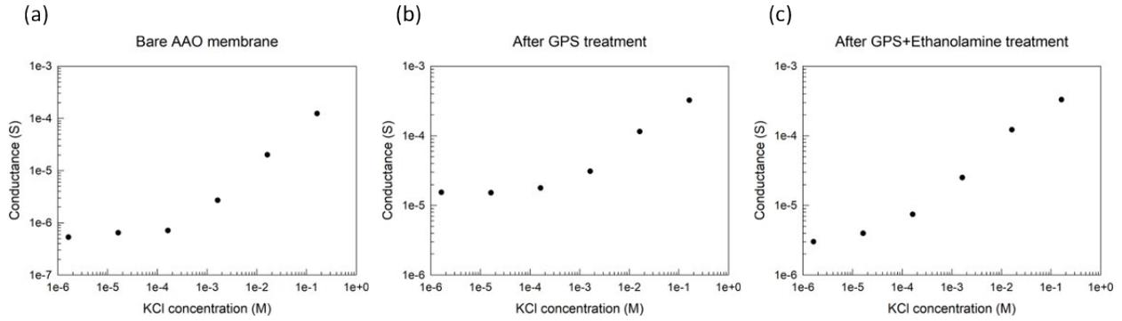
Figure 7 Measured conductance through the nanoporous membrane. (a) Bare membrane (b) After treating the membrane with a 2% solution of 3-glycidoxypropyl trimethoxysilane(GPS) in ethanol for 1 hour (c) After treating the membrane with a 2% solution of GPS in ethanol for 1 hour followed by 50mM ethanolamine in DI water for 30 minutes. Note that the active area of each membrane was different.
