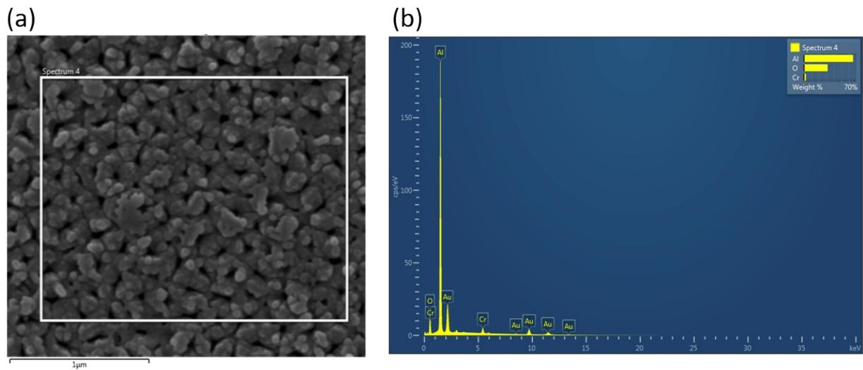
Figure 5. Surface characterization with energy-dispersive spectroscopy (EDS). (a) SEM image of the surface acquired with a FEI Quanta-600 scanning electron microscope. Surface marked with the white square was analyzed (b) EDS spectrum acquired with EDS. Al, O, Cr, Au peaks are observed.
