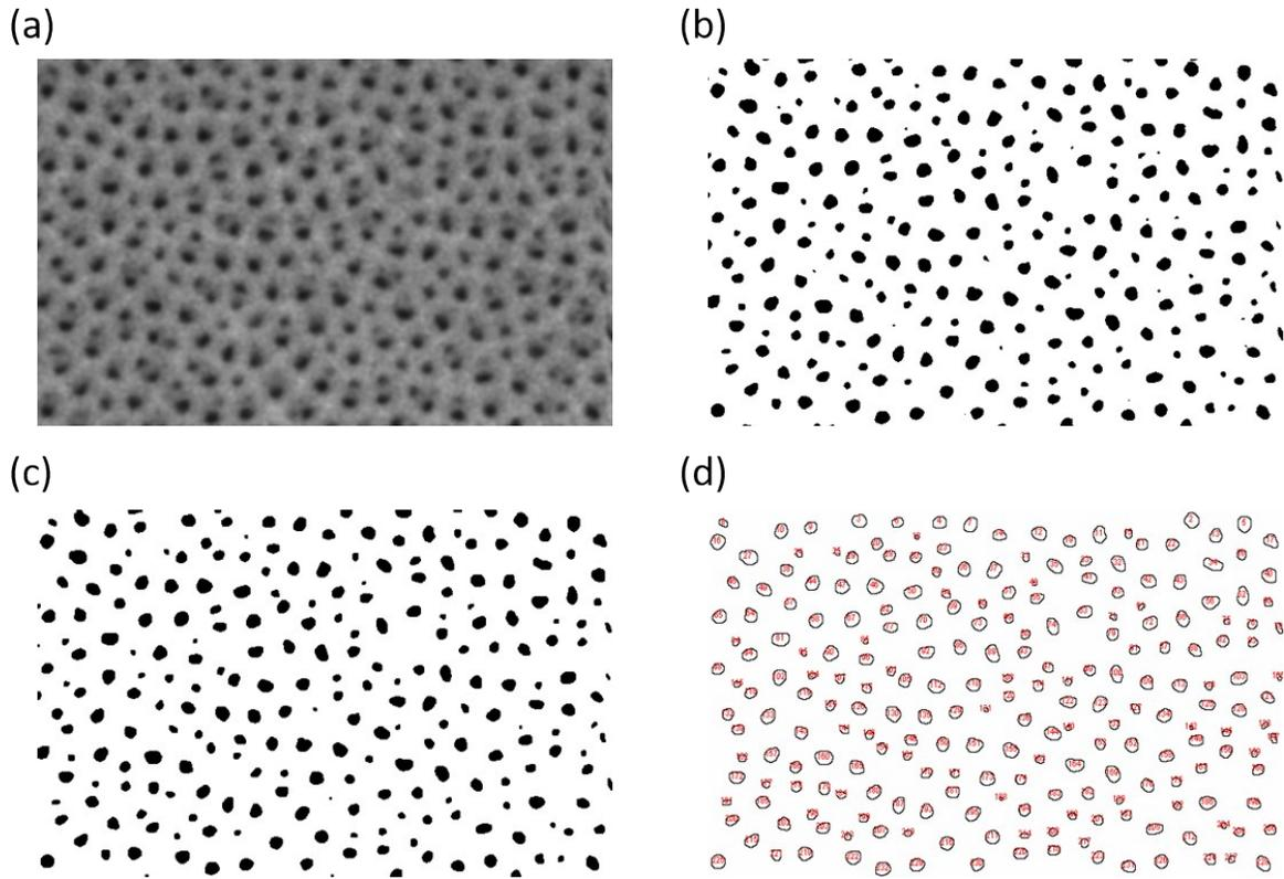
Figure 4 Image processing for the characterization of the nanoporous membrane. All processes were done with ImageJ. (a) Gaussian blurred image for the noise reduction (b) Converted to black and white image by setting the threshold value (c) Image after the smoothing process with erode and dilate (d) Particle analysis result
