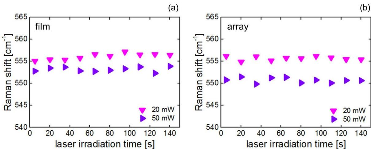
**Figure S5.** Time dependent Raman shift for (a) the TiN film on the sapphire substrate and (b) TiN array on the sapphire substrate where the superstrates are water.
