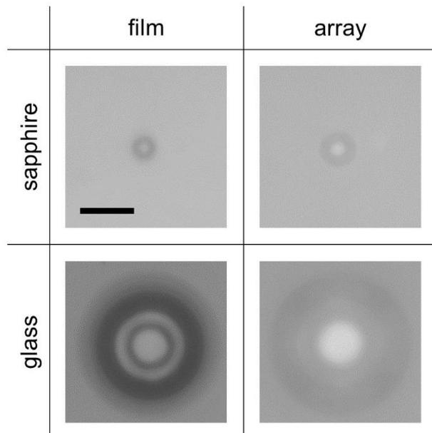
**Figure S6.** Optical images of the bubbles of the four different samples with water superstrates; TiN film on sapphire substrate, TiN array on sapphire substrate, TiN film on glass substrate, and TiN array on glass substrate. All the images were taken at the same magnification and the scale bar shows 20  $\mu\text{m}$ .
