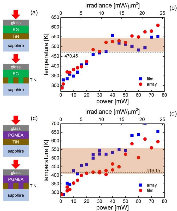
**Figure S9.** (a) Schematics of the samples with sapphire substrates where the superstrates are ethylene glycol (EG) layers. (b) Laser power dependent temperature increase of the samples with EG as superstrate. (c) Schematics of the samples with sapphire substrates where the superstrates are 2-Acetoxy-1-methoxypropane (PGMEA) layers. (d) Laser power dependent temperature
