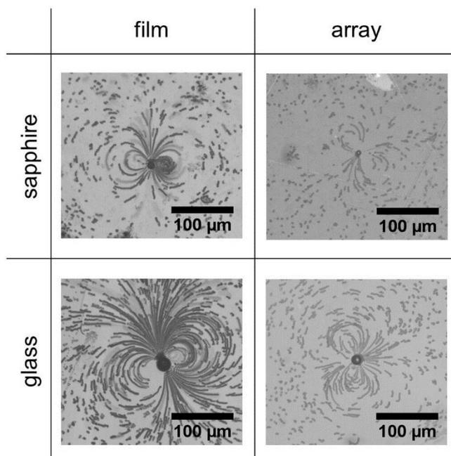
**Figure S7.** Visualized Marangoni flows of four different samples with water superstrates; TiN on sapphire substrate, TiN array on sapphire substrate, TiN film on glass substrate, and TiN array on glass substrate. To visualize Marangoni flows, polystyrene spheres were dispersed in water before the measurements.
