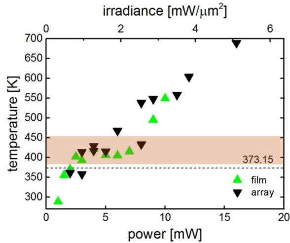
Figure S8. Experimentally recorded laser power dependent temperature of the samples with the glass substrates and water superstrates. The data are identical to Figure 4(d) in the main text but plotted with a different x-axis range. The top x-axis was calculated from the bottom x-axis using the beam area.
