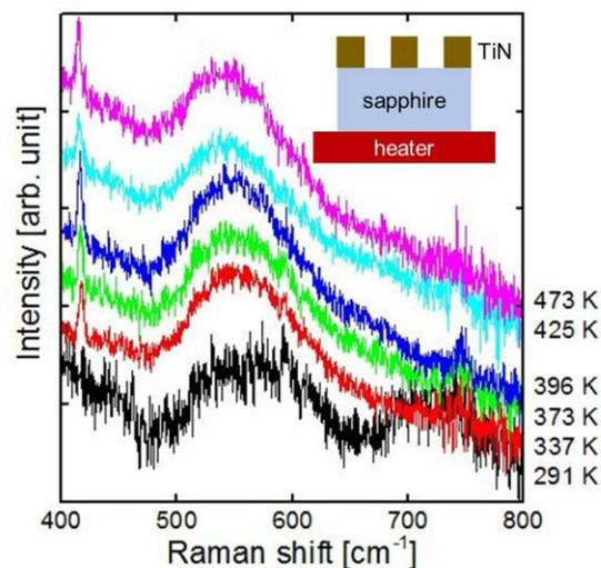
**Figure S3.** Stokes peaks of the array on the sapphire substrate recorded at various temperatures. The sample was heated by a sample heater and the temperature was monitored on the surface of the sample. The sharp peak at  $\sim 410 \text{ cm}^{-1}$  was from the sapphire substrate. The excitation was a He-Ne laser at  $\sim 3 \text{ mW}$ .
