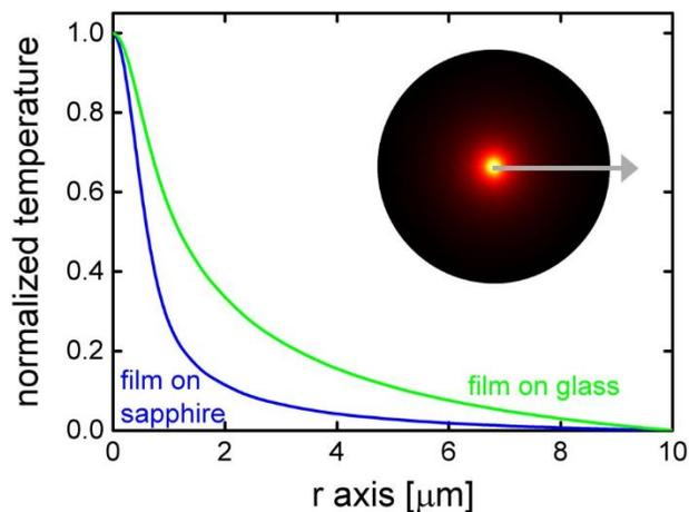
**Figure S4.** Simulated temperature profiles of the TiN films on the sapphire and glass substrates where the superstrates are air. The inset shows the normalized temperature map of the TiN film on the sapphire substrate. The size of the color map is 10  $\mu\text{m}$  in radius.
