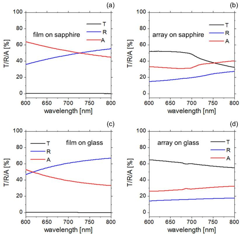
**Figure S2.** Transmittance (T), reflectance (R) and absorptance (A) of the four samples where the superstrates were air. (a) Film on the sapphire substrate, (b) array on the sapphire substrate, (c) film on the glass substrate and (d) array on the glass substrate.
