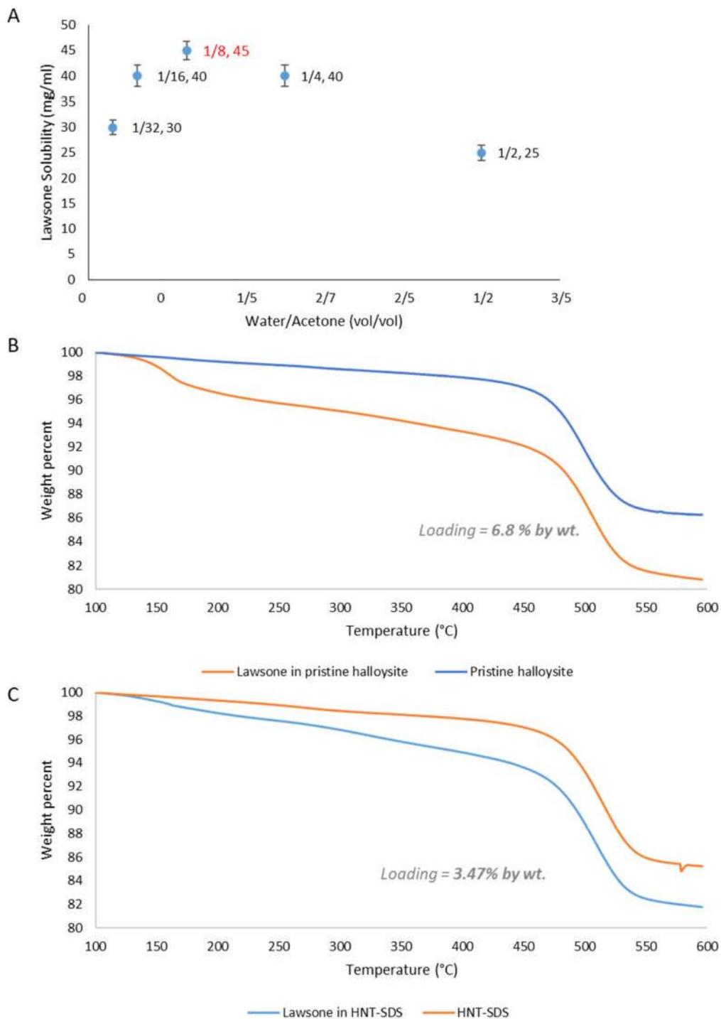
Figure S7: Optimisation of lawsone solubility (A). Lawsone was found to have increased solubility in a mixture of water to acetone, with the 1:8 mixture bearing solubility 2.25 times over pure acetone. TGA spectra of lawsone loaded in pristine (B) and HNT-SDS(C).
