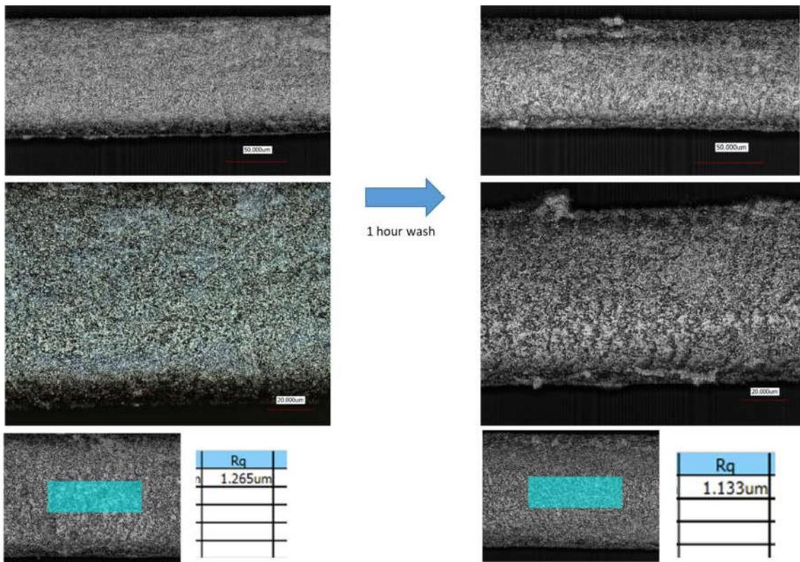
Figure S4. Coating of ODTMS-halloysite CA 57° on hair (left) is intact after 1-hour rigorous wash (right) as indicated by optical pictures and roughness measurement (Rq is root mean square roughness in inset)
