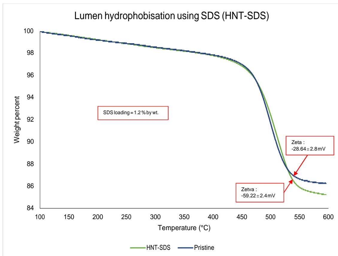
Figure S8: TGA spectra of HNT-SDS against pristine halloysite with zeta potential measurement labels showing increased negative charge on modified halloysite.
