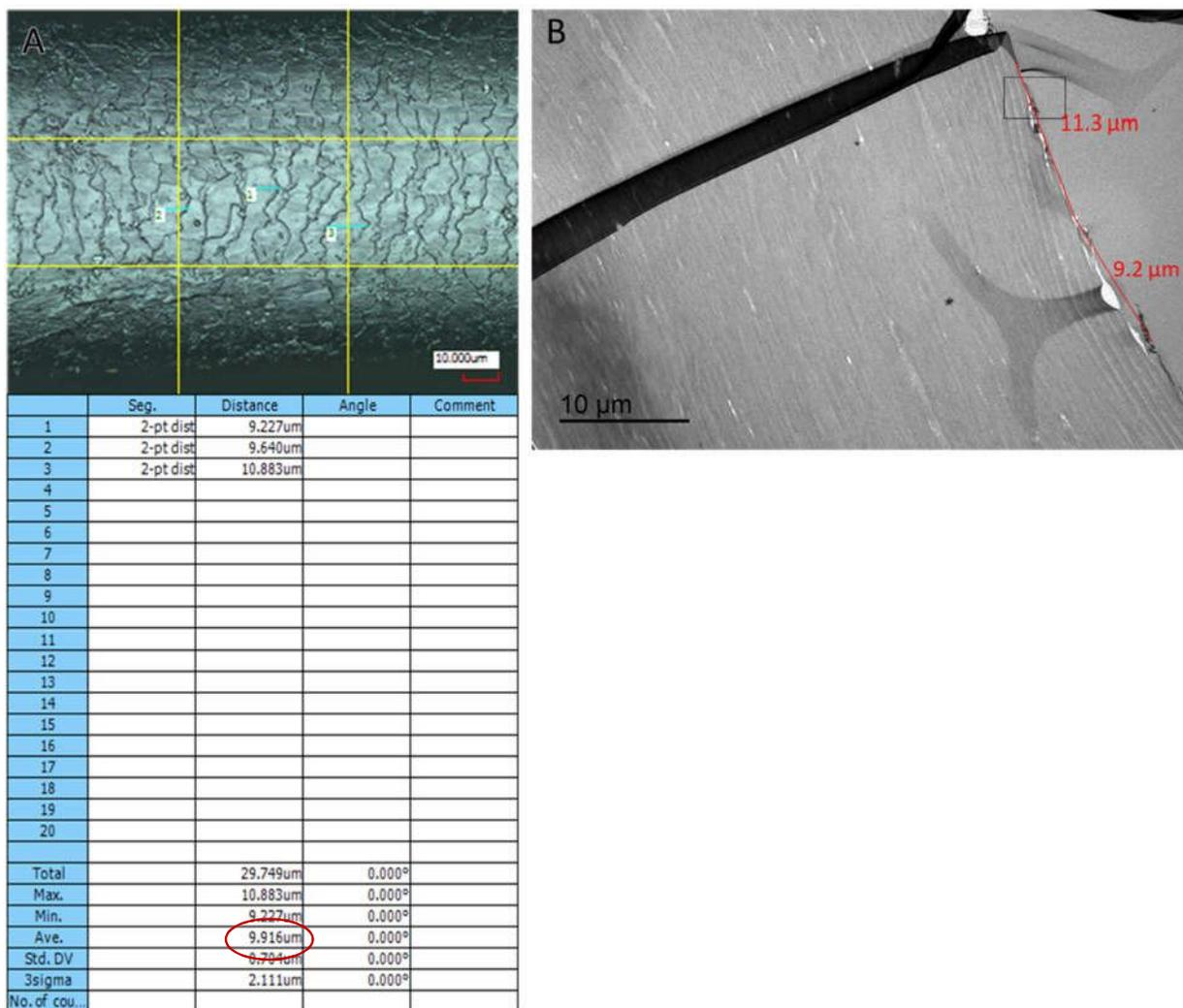
Figure S2: Profilmetry measurements of pristine hair show cuticles are spaced out at an interval of ca. 10  $\mu\text{m}$  away from each other (A). The TEM image (B) of longitudinal section of halloysite coated hair show dark clay deposits at a similar interval indicating the cuticle ends as sites for initiation of assembly of halloysite tubes.
