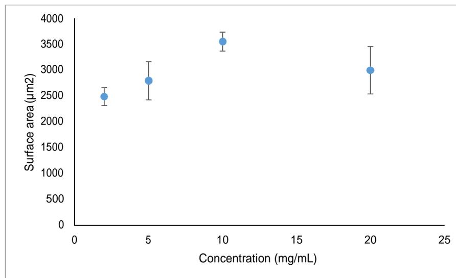
Figure S6: Profilometry surface area measurements of coated hair samples varying with dispersion concentration.
