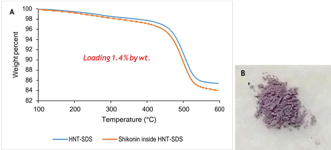
Figure S14. TGA spectra (A) and image of shikonin from extract of Alkanet root encapsulated in pristine halloysite (B)
