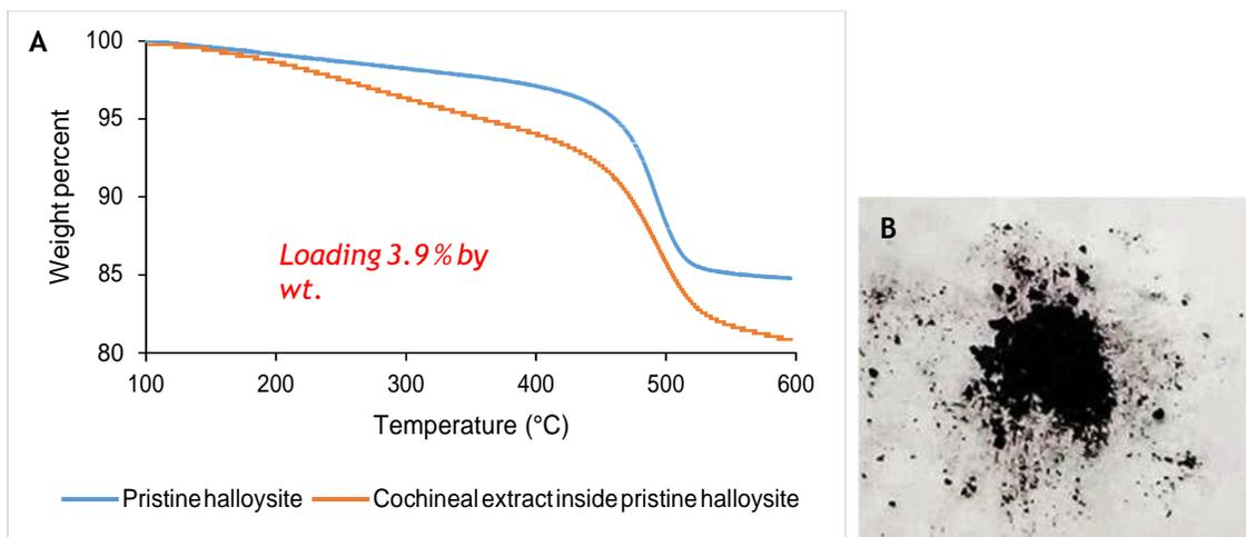
Figure S13. TGA spectra (A) and image of cochneal extract (carmine) in pristine halloysite (B)
