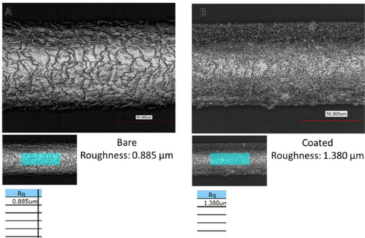
Figure S1. Visual and roughness measurement of bare (A) and coated (B) hair with the root mean square roughness (Rq) enlarged in inset.
