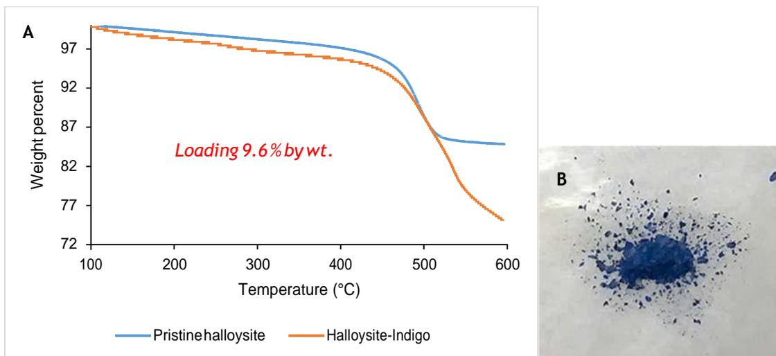
Figure S12. TGA spectra (A) and image of HNT-Indigo halloysite (B)
