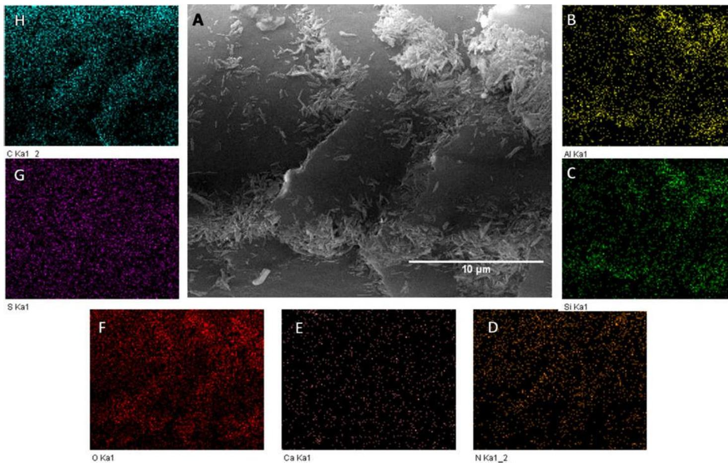
Figure S3: EDX spectra elemental maps of hair coated by pristine halloysite tubes. Original image (A) and corresponding Aluminium (B), Silica (C), Nitrogen (D), Calcium (E), Oxygen (F), Sulphur (G) and Carbon (H) maps. The Si and Al maps (B & C) are imprints of the halloysite deposit sites on the hair surface.
