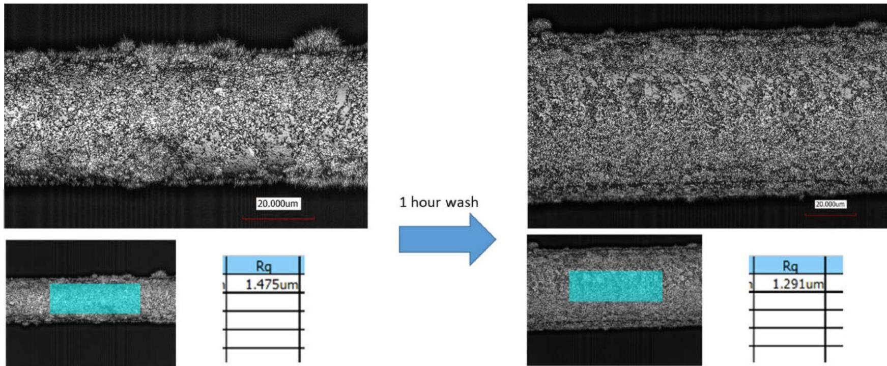
Figure S5. Coating of ODTMS-halloysite CA 116° on hair (left) is intact after 1-hour rigorous wash (right) as indicated by optical pictures and roughness measurement (Rq is root mean square roughness in inset)
