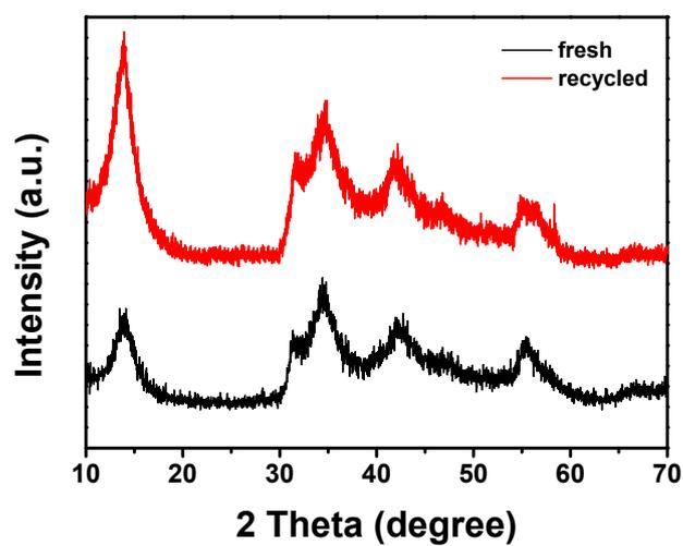
**Fig. S7.** The XRD patterns of WSe<sub>2</sub> nanosheets before and after undergoing 5 recycles.
