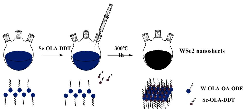
**Fig. S2.** Schematic illustration of the colloidal synthesis procedure of WSe<sub>2</sub> nanosheets
