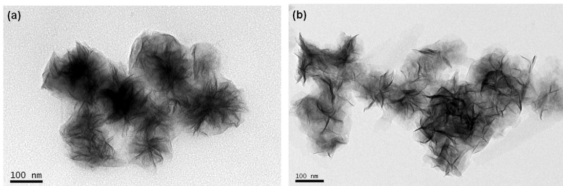
**Fig. S8.** The TEM images of WSe<sub>2</sub> nanosheets before (a) and after (b) undergoing 5 cycles.
