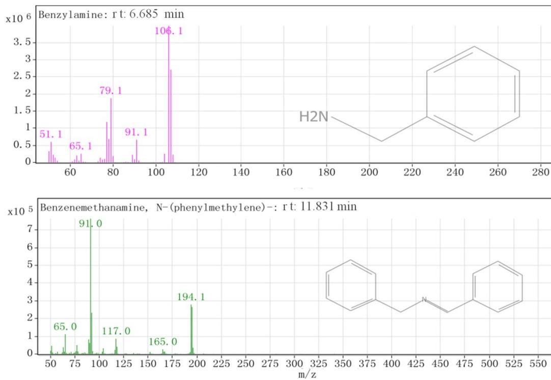
**Fig. S6.** GC-MS of the photochemical oxidation of benzylamine for 10 hours.
