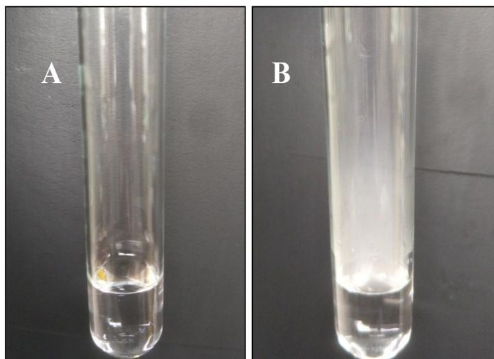
**Fig. S5.** NH<sub>3</sub> qualitative detection: (A) reaction solution before adding the glass rod and (B) the formation of white fumes of ammonium chloride.
