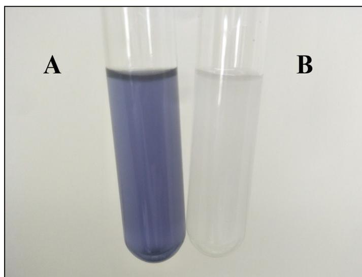
**Fig. S4.** H<sub>2</sub>O<sub>2</sub> qualitative detection: (A) reaction solution and (B) pure benzylamine solution reacts with potassium iodide for a period of time and then uses starch as an indicator.
