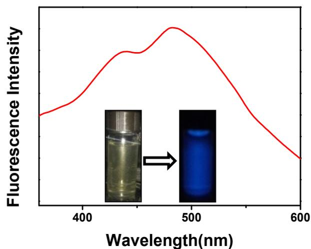
**Fig. S3.** fluorescence emission spectra of the WSe<sub>2</sub> nanosheets dispersed in solvent NMP excited by 380 nm, the inset shows photo pictures of WSe<sub>2</sub> solution without and with light irradiation.
