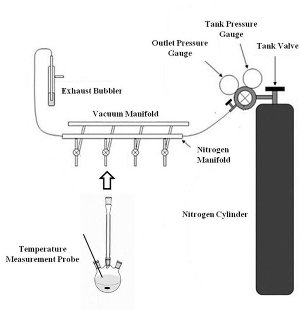
**Fig. S1.** Schematic diagram of the reaction device.
