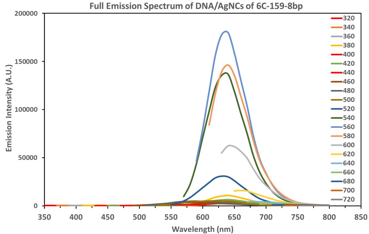
Supplementary figure 3. Emission spectra of 6C-159-8bp (3.75  $\mu\text{M}$ ). The spectra were recorded by exciting from 300-720 nm in 20 nm steps. The spectral homogeneity in emission maximum indicates the presence of single type of AgNCs.
