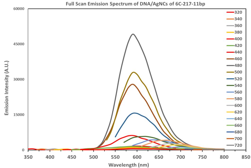
Supplementary figure 2. Emission spectra of 6C-217-11bp (3.75  $\mu\text{M}$ ). The spectra were recorded by exciting from 300-720 nm in 20 nm steps. The spectral heterogeneity in emission maximum indicates the presence of one type of AgNCs, with one being the dominant at Ex/Em 480/590 nm.
