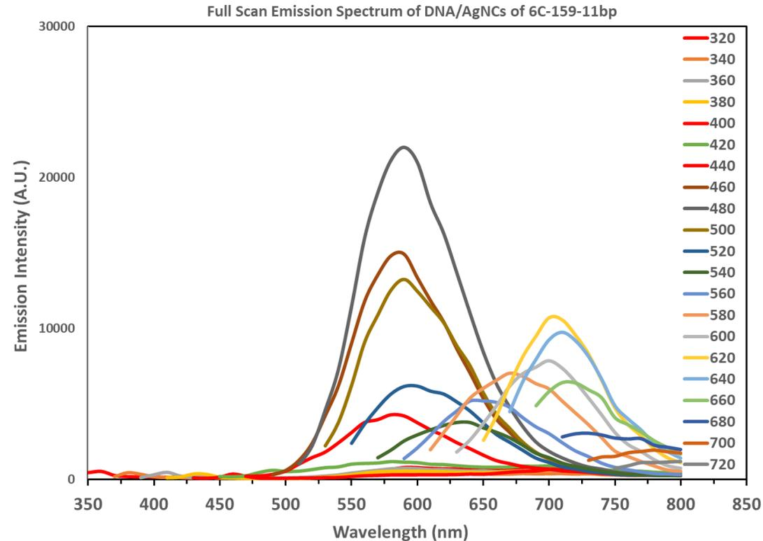
Supplementary Figure 4. Emission spectra of 6C-159-11bp (3.75  $\mu\text{M}$ ). The spectra were recorded by exciting from 300-720 nm in 20 nm steps. The spectral heterogeneity in emission maximum indicates the presence of at least two types of AgNCs, with one being dominant at Ex/Em 480/590 nm. The second emission peak with Ex/Em at 580/660 nm can also be seen. Another peak appears at Near Infrared emission at Ex/Em 620/710 nm but this could not be visualized on the gel.
