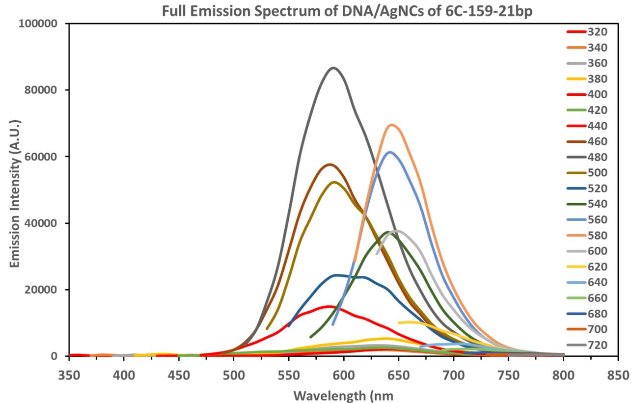
Supplementary Figure 6. Emission spectra of 6C-159-21bp (3.75  $\mu\text{M}$ ). The spectra were recorded by exciting from 300-720 nm in 20 nm steps. The spectral heterogeneity in emission maximum indicates the presence of at-least two types of AgNCs, with one being the dominant at Ex/Em 480/590 nm. The second emission peak corresponds to Ex/Em 580/660 nm.
