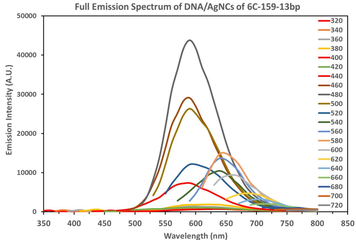
Supplementary Figure 5. Emission spectra of 6C-159-13bp (3.75  $\mu\text{M}$ ). The spectra were recorded by exciting from 300-720 nm in 20 nm steps. The spectral heterogeneity in emission maximum indicates the presence of at least two types of AgNCs, with one being the dominant at Ex/Em 480/590 nm. The second emission peak with Ex/Em at 580/660 nm can also be seen.
