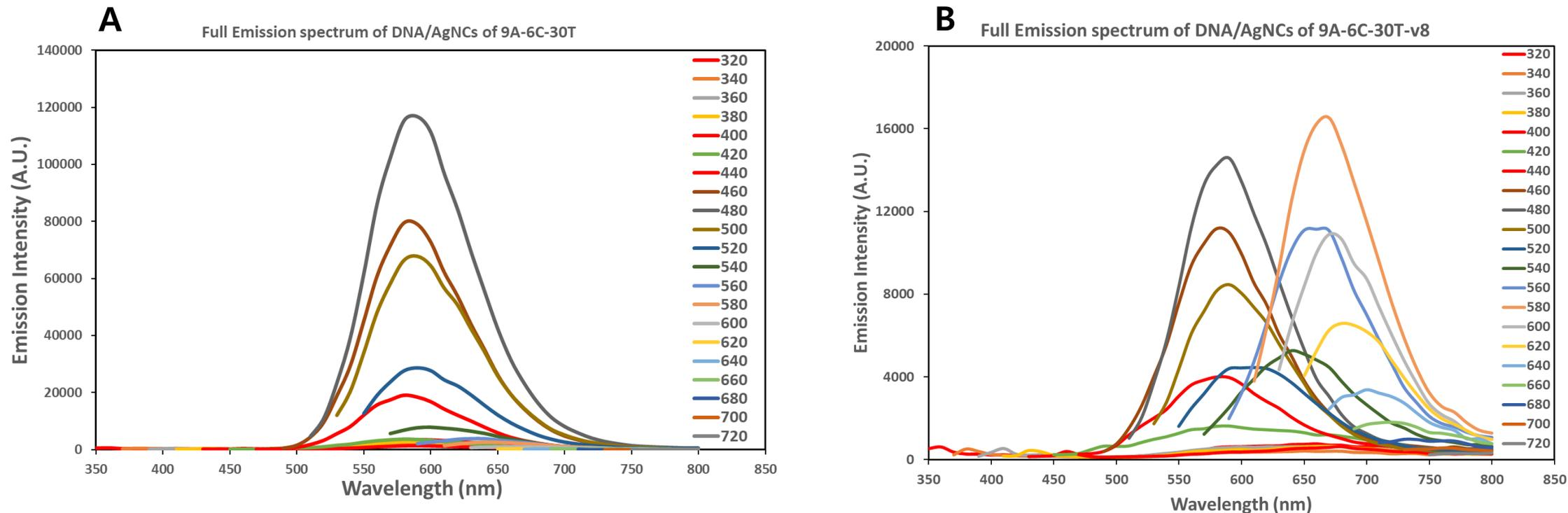
Supplementary Figure 7. A) Emission spectra of 9A-6C-30T (3.75  $\mu$ M). The spectra were recorded by exciting from 300-720 nm in 20 nm steps. The dominant AgNC emits at Ex/Em 480/590 nm. B) Emission spectra of 9A-6C-30T-v8 (3.75  $\mu$ M). The spectra were recorded by exciting from 300-720 nm in 20nm steps. The spectral heterogeneity in emission maximum indicates the presence of two types of AgNCs, with one being the dominant at Ex/Em 480/590 nm and second one with Ex/Em at 580/660 nm.
