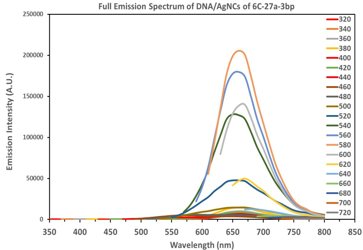
Supplementary figure 1. Emission spectra of 6C-27a-3bp (3.75  $\mu\text{M}$ ). The spectra were recorded by exciting from 300-720 nm in 20 nm steps. The spectral homogeneity in emission maximum indicates the presence of single type of AgNCs.
