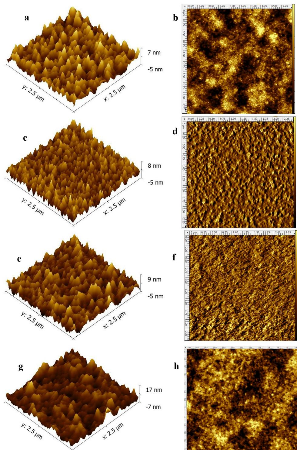
**Figure S4.** 3D and phase images of AFM images of the binary and ternary thin films.
