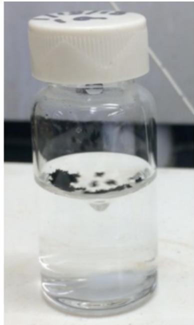
**Fig. S3.** Photographs of raw SWCNTs before electrolysis in DI water.
