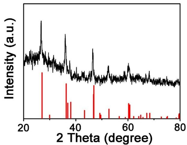
**Fig. S5** XRD pattern of the PVP-Fe<sub>3</sub>S<sub>4</sub> tetragonal nanosheets after H<sub>2</sub>O<sub>2</sub> treatment.
