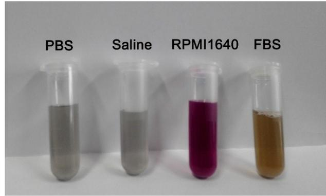
**Fig. S3** A camera image of the PVP-Fe<sub>3</sub>S<sub>4</sub> tetragonal nanosheets dispersed in PBS, Saline, RPMI1640, and FBS, respectively, for two days.
