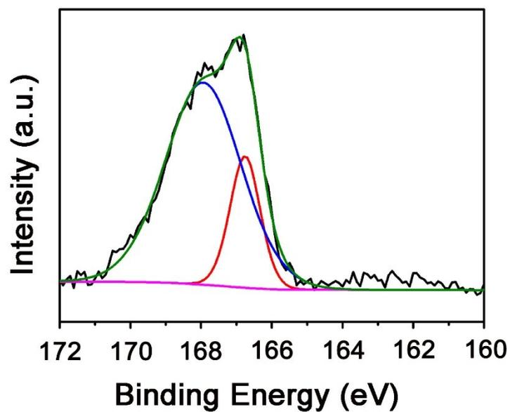
**Fig. S6** S 2p regions for the PVP-Fe<sub>3</sub>S<sub>4</sub> tetragonal nanosheets after H<sub>2</sub>O<sub>2</sub> treatment.
