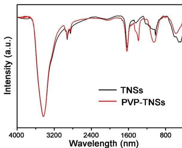
**Fig. S2** FTIR spectra of the  $\text{Fe}_3\text{S}_4$  tetragonal nanosheets and PVP- $\text{Fe}_3\text{S}_4$  tetragonal nanosheets. The bands at 2850-2950  $\text{cm}^{-1}$  are corresponded to asymmetric and symmetric stretching vibrations of methylene ( $\text{CH}_2$ ) of the long alkyl chain in OLA. The bands at 2850-2950  $\text{cm}^{-1}$  are due to the C-H stretching vibration in PVP and the band around 1400  $\text{cm}^{-1}$  is assigned to the C-H deformation vibration in PVP.
