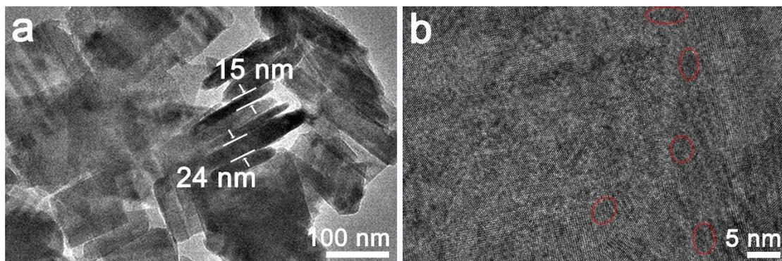
**Fig. S1** (a) TEM and (b) HRTEM images of the  $\text{Fe}_3\text{S}_4$  tetragonal nanosheets.
