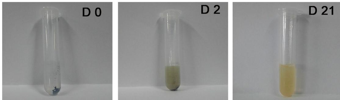
**Fig. S4** The camera images of the PVP-Fe<sub>3</sub>S<sub>4</sub> tetragonal nanosheets dispersed in PBS for different days under a magnet nearby.
