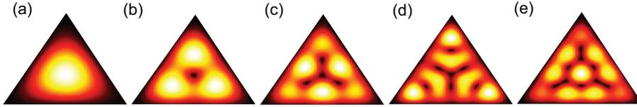
FIG. S2: The lowest five optical mode distribution  $E_z(x, y)$  in a triangle cavity. The side length of the cavity is 1083 nm.
