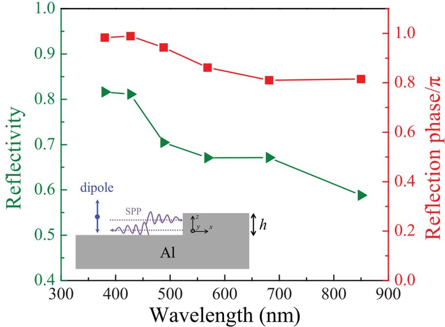
FIG. S1: Simulated reflectivity and reflection phase shift of the out-of-plane component of SPPs for the cavity reflectors. The height of the reflector is 136 nm.
