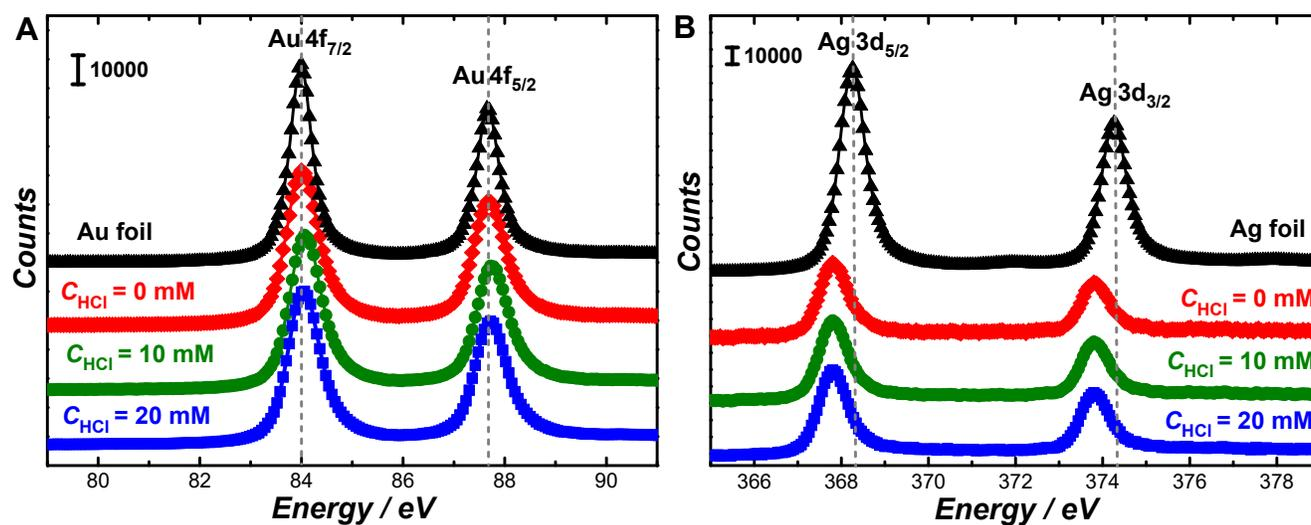
**Figure S2.** XPS spectra of (A) Au 4f and (B) Ag 3d regions of nanoparticles synthesized after 16 h in 100 mM CTAC, 50  $\mu\text{M}$   $\text{AgNO}_3$ , 500  $\mu\text{M}$   $\text{HAuCl}_4$ , and 1.2 mM AA in the presence of 0, 10, and 20 mM HCl. The spectra of a bulk Au foil and Ag foil were also shown for comparison. The spectra were offset for clarity.
