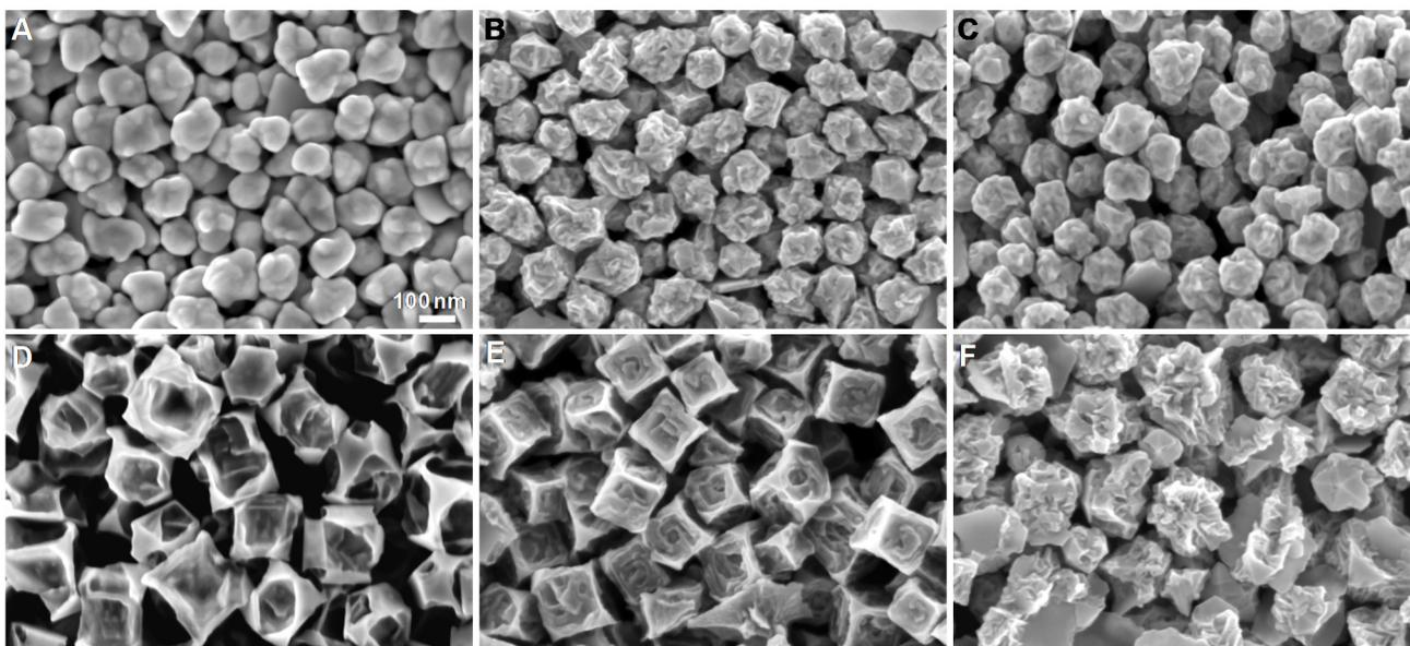
**Figure S9.** Effects of AA. SEM images of nanoparticles synthesized after 16 h in growth solutions containing 100 mM CTAC, 50  $\mu\text{M}$   $\text{AgNO}_3$ , 500  $\mu\text{M}$   $\text{HAuCl}_4$ , and various concentrations of AA and HCl: (A) 0.5 mM AA, 2 mM HCl; (B) 1 mM AA, 2 mM HCl; (C) 5 mM AA, 2 mM HCl; (D) 1 mM AA, 20 mL HCl; (E) 2.5 mM AA, 20 mL; (F) 5 mM AA, 20 mM HCl. All SEM images share the same scale bar in panel A.
