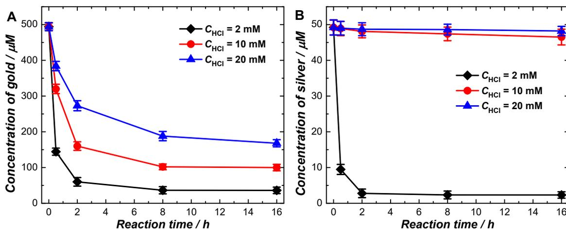
**Figure S7.** Total amounts of (A) gold and (B) silver remaining in the supernatant at various reaction times quantified by ICP-MS. The growth solutions contained 100 mM CTAC, 50  $\mu\text{M}$   $\text{AgNO}_3$ , 500  $\mu\text{M}$   $\text{HAuCl}_4$ , 1.2 mM AA, and 2, 10, or 20 mM HCl.
