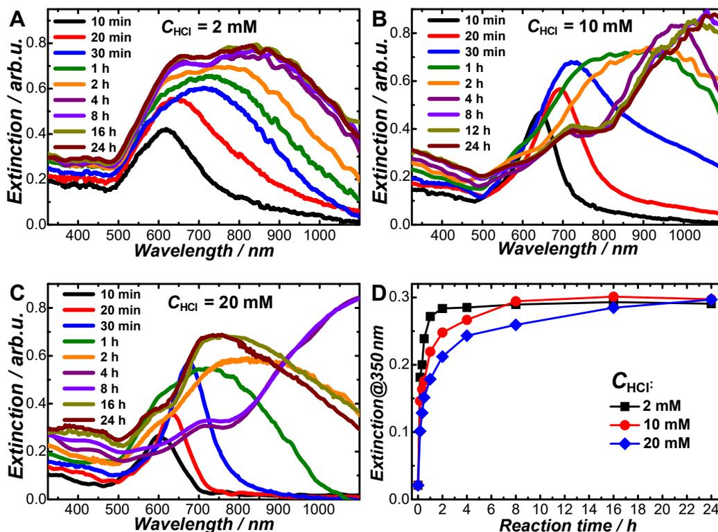
**Figure S8.** Temporal evolution of optical extinction spectra during nanocrystal growth in 100 mM CTAC, 50  $\mu\text{M}$   $\text{AgNO}_3$ , 500  $\mu\text{M}$   $\text{HAuCl}_4$ , 1.2 mM AA, and (A) 2 mM, (B) 10 mM, and (C) 20 mM HCl. (D) Temporal evolution of optical extinction at 350 nm.
