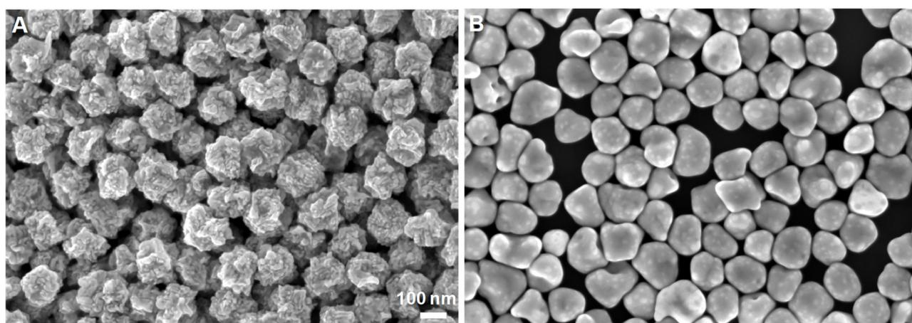
**Figure S14.** (A) SEM image of Au nanoparticles synthesized after 16 h in a growth solution containing 100 mM CTAC, 500  $\mu\text{M}$   $\text{HAuCl}_4$ , and 1.2 mM AA. (B) SEM image of the nanoparticles obtained after exposing the nanoparticles shown in panel A to an etching solution containing 100 mM CTAC and 10 mM HCl for 16 h. Both SEM images share the same scale bar in panel A.
