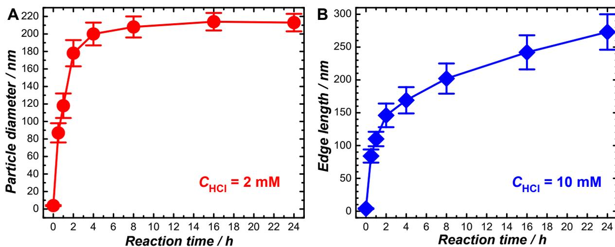
**Figure S5.** Temporal evolution of particle sizes during the seed-mediated nanocrystal growth in growth solutions containing 100 mM CTAC, 50  $\mu\text{M}$   $\text{AgNO}_3$ , 500  $\mu\text{M}$   $\text{HAuCl}_4$ , 1.2 mM AA, and (A) 2 and (B) 10 mM HCl. The average particle sizes and standard deviations were obtained from 100 particles in the SEM images for each sample. The Au seeds were  $3.9 \pm 0.6$  nm in diameter.
