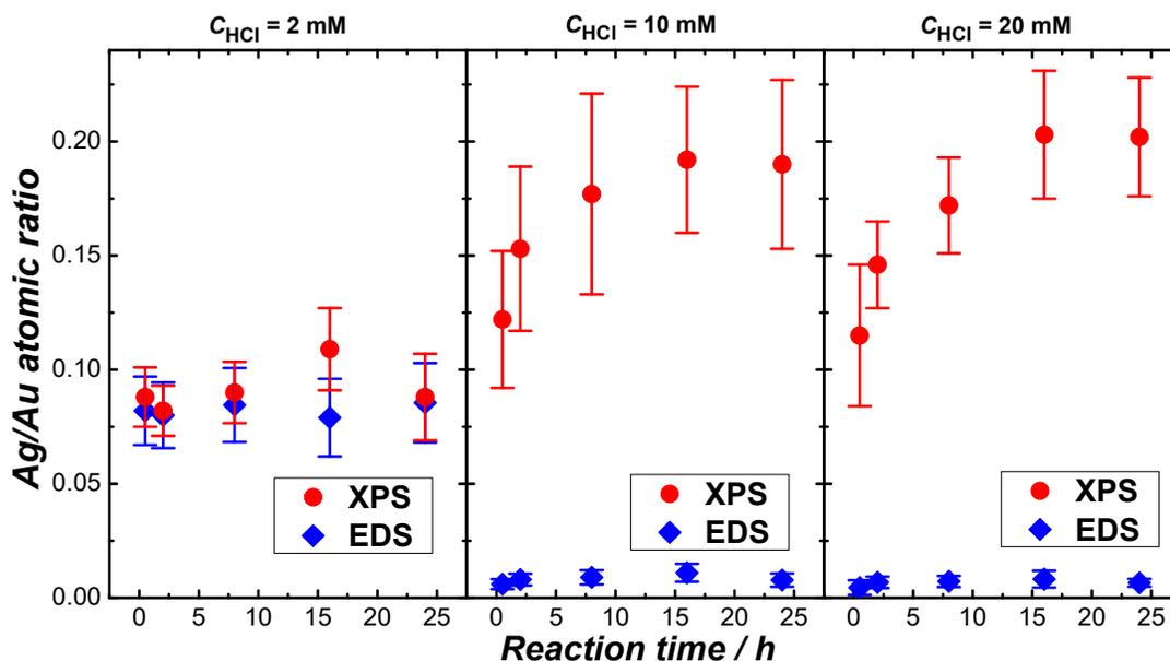
**Figure S6.** Temporal evolution of surface Ag/Au atomic ratio (quantified by XPS) and bulk Ag/Au atomic ratio (quantified by EDS) during seed-mediated nanocrystal growth in growth solutions containing 100 mM CTAC, 50  $\mu\text{M}$   $\text{AgNO}_3$ , 500  $\mu\text{M}$   $\text{HAuCl}_4$ , 1.2 mM AA, and (left panel) 2, (middle panel) 10, and (right panel) 20 mM HCl. The error bars represent the standard deviations obtained from 3 samples synthesized under identical conditions.
