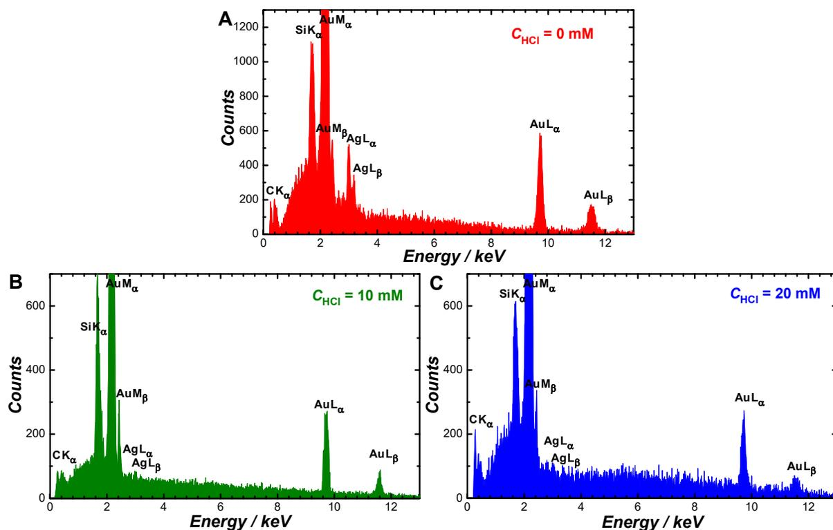
**Figure S3.** EDS spectra of nanoparticles synthesized after 16 h in 100 mM CTAC, 50  $\mu\text{M}$   $\text{AgNO}_3$ , 500  $\mu\text{M}$   $\text{HAuCl}_4$ , 1.2 mM AA, and (A) 0, (B) 10, and (C) 20 mM HCl. The Si signals were from the Si substrates.
