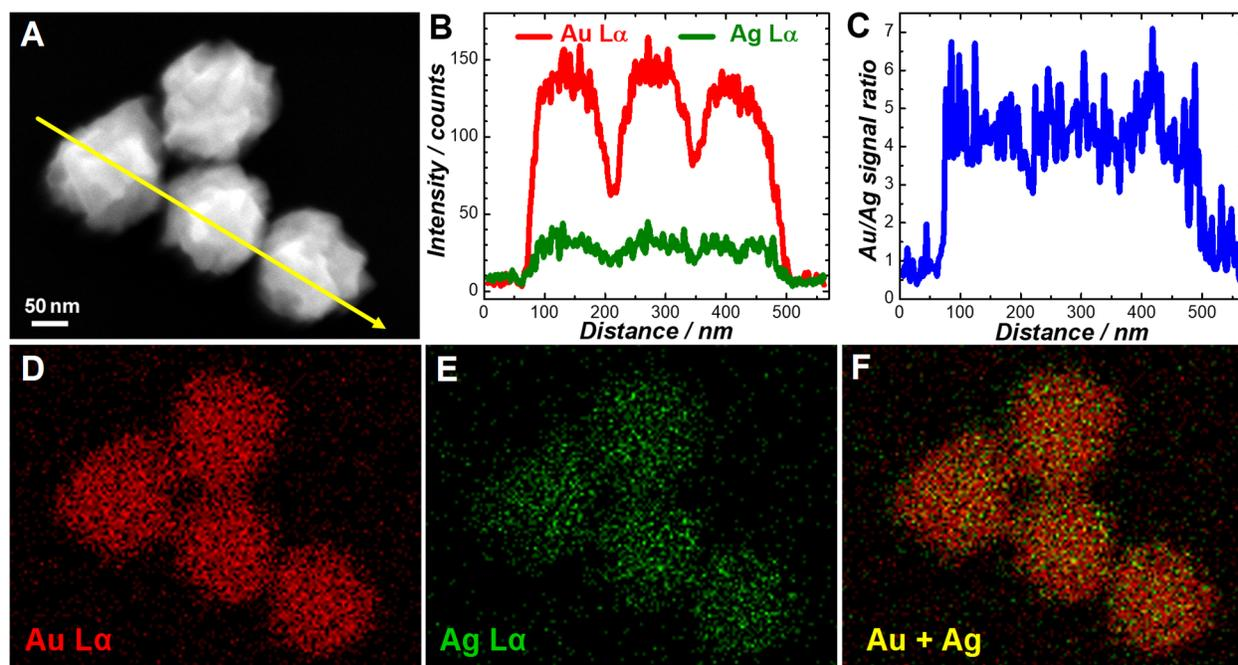
**Figure S4.** (A) SEM image of Au-Ag alloy surface-textured quasi-spherical nanoparticles synthesized after 16 h in a growth solution containing 100 mM CTAC, 50  $\mu\text{M}$   $\text{AgNO}_3$ , 500  $\mu\text{M}$   $\text{HAuCl}_4$ , and 1.2 mM AA. (B) Line-profiles of EDS intensities of Au L $\alpha$  and Ag L $\alpha$ , and (C) line-profile of Au/Ag signal ratios across the yellow line in panel A. EDS elemental maps of (D) Au, (E) Ag, and (F) overlay of Au + Ag.
