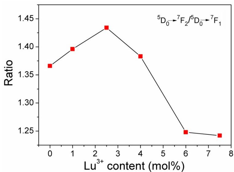
**Fig. S4** The dependence of the ratio of intensity ( $^5D_0 \rightarrow ^7F_2/^5D_0 \rightarrow ^7F_1$ ) on  $\text{Lu}^{3+}$  doping content in  $\beta\text{-NaGdF}_4:1\%\text{Eu}$  NPs doped with different concentrations of  $\text{Lu}^{3+}$  ions.
