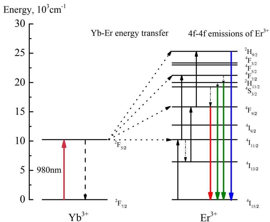
**Fig. S3** The energy level diagram for the  $4f$  electronic configurations of  $\text{Yb}^{3+}$  and  $\text{Er}^{3+}$  ions and the upconversion luminescence mechanism of  $\text{Yb}^{3+}/\text{Er}^{3+}$ -codoped materials with the excitation of 980 nm.
