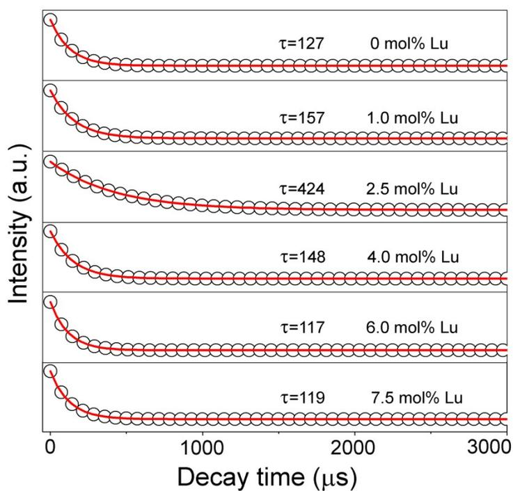
**Fig. S5** Temporal evolution of UCL from the  $^4F_{9/2}$  level of  $\text{Er}^{3+}$  in the  $\beta\text{-NaGdF}_4\text{:Yb,Er,X\%Lu}$  NPs ( $X = 0, 1, 2.5, 4, 6$  and  $7.5$ ) under the excitation of a 980 nm pulsed Raman shift laser: experimental data (black circles) and fitting by single-exponential function ( $I = I_0 \exp(-t/\tau)$ ) (red solid line).
