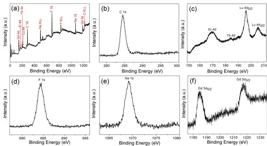
**Fig. S1** (a) XPS survey spectrum and (b) C 1s, (c) Yb 4d, Er 4d, Lu 4d<sub>5/2</sub>, and Lu 4d<sub>3/2</sub>, respectively, (d) F 1s, (e) Na 1s, (f) Gd 3d<sub>5/2</sub> and Gd 3d<sub>3/2</sub> spectra of NaGdF<sub>4</sub>:18%Yb,2%Er,2.5%Lu NPs.
