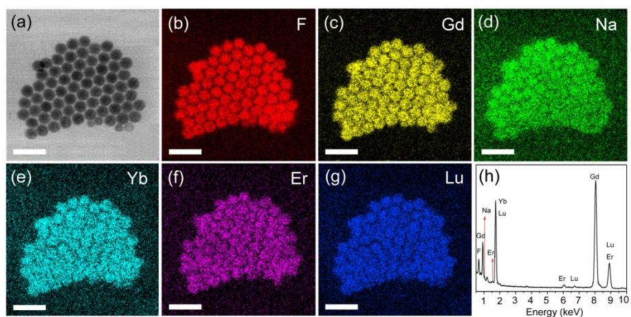
**Fig. S2** (a) STEM image (b-g) EDX elemental mapping of  $\text{NaGdF}_4:18\%\text{Yb},2\%\text{Er},2.5\%\text{Lu}$  NPs and line-profile analysis of  $\text{NaGdF}_4:18\%\text{Yb},2\%\text{Er},2.5\%\text{Lu}$  NPs with different elements (F, Gd, Na, Yb, Er and Lu), (h) EDX spectrum of  $\text{NaGdF}_4:18\%\text{Yb},2\%\text{Er},2.5\%\text{Lu}$  NPs. The scale bar is 25 nm.
