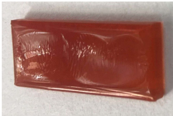
Figure S2. Photograph of the \alpha -Fe 2 O 3 nanostructured array synthesized at pH 1.7 and annealed at 800 °C.
