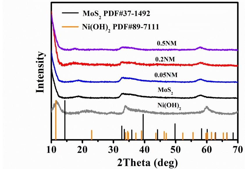
**Fig. S4** XRD patterns of  $\text{Ni(OH)}_2$ ,  $\text{MoS}_2$ , and  $\text{Ni(OH)}_2/\text{MoS}_2$  heterostructures
