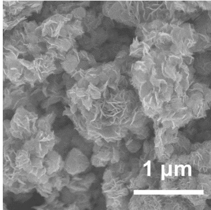
**Fig. S2** SEM image of the pure MoS<sub>2</sub>.
