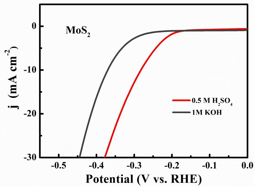
**Fig. S6** LSV curves of the pure  $\text{MoS}_2$  in  $0.5\text{M H}_2\text{SO}_4$  and  $1\text{M KOH}$ .
