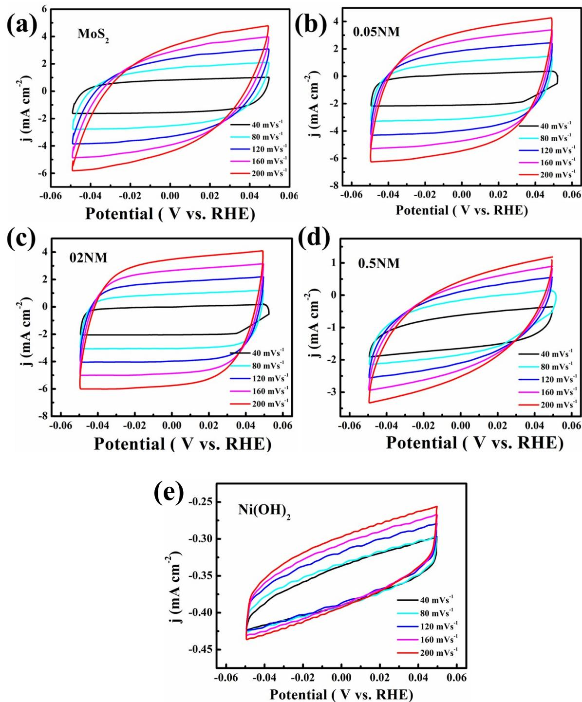
**Fig. S8** CV curves of (a) MoS<sub>2</sub>, (b) 0.05NM, (c) 0.2NM, (d) 0.5NM, and (e) Ni(OH)<sub>2</sub> at various scan rates
