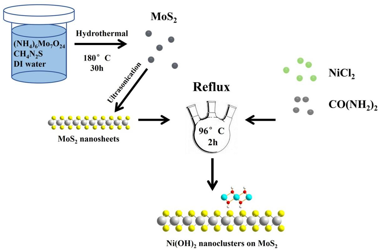
**Fig. S1** Illustration scheme for materials synthesizing procedures.
