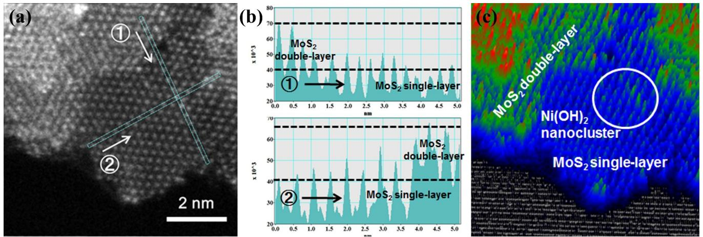
**Fig. S3** (a) HAADF-STEM image of 0.2NM, the arrows indicate the direction of the intensity profiles. (b) the corresponding intensity profiles, showing a nanodomain with an average intensity between single-layer MoS<sub>2</sub> and double-layer MoS<sub>2</sub>. (c) the corresponding surface plot image, illustrating Ni(OH)<sub>2</sub> nanocluster on the surface of single-layer MoS<sub>2</sub>.
