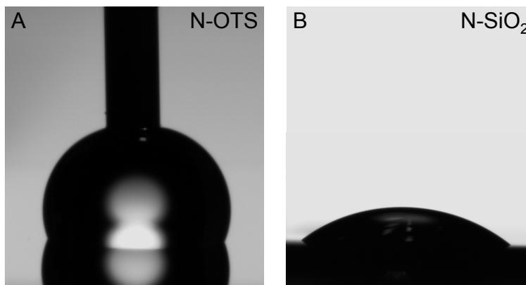
**Figure S1** Water contact angle measurements, exemplary shown for the N-wafer A: with and B: without silanization (after piranha cleaning).
