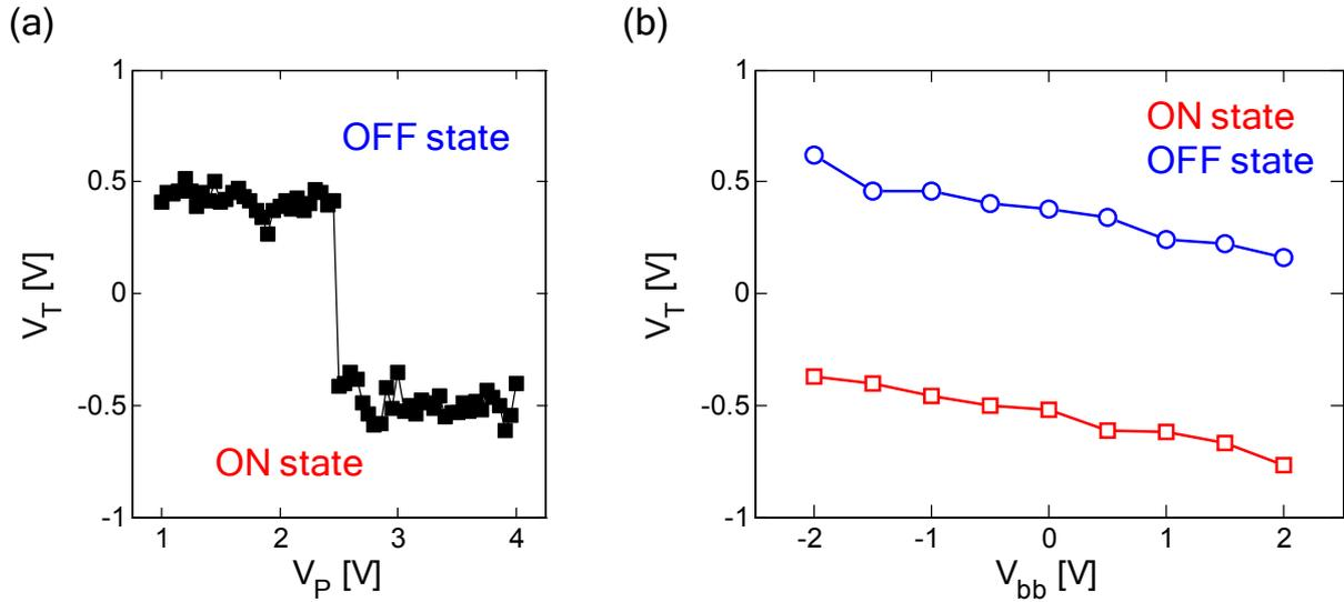
Figure S3 | Ferroelectric switching in FDSOI FeFETs. (a) Voltage dependent switching (b) Effect of the back-bias voltage  $V_{bb}$  on the threshold voltage for the two stored states.
