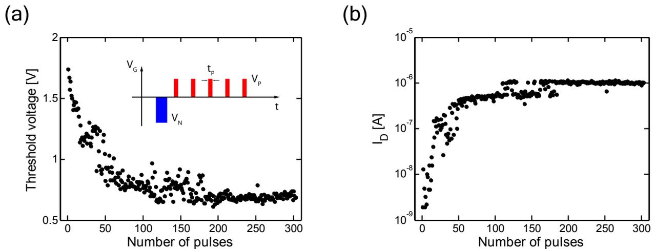
Figure S2 | Gradual accumulative switching in large-area FeFETs. (a) Threshold voltage and (b) drain current evolution upon a train of identical pulses ( $V_p = 3\text{V}$ ,  $t_p = 1\mu\text{s}$ ). Threshold voltage is extracted at  $I_D = 0.1\mu\text{A} * W/L$ .
