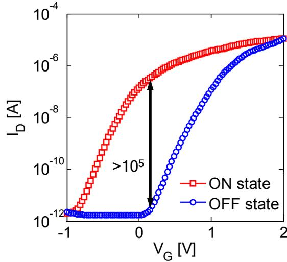
Figure S1 | Long-integration measurement of  $I_D$ - $V_G$  curves for the two polarization states.
