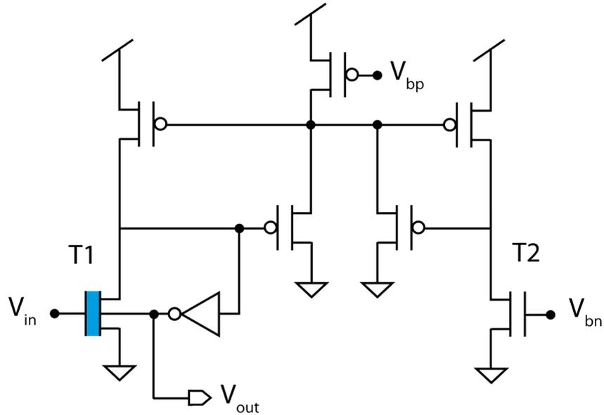
Fig. S4 A possible implementation a FeFET based neuron circuit. T1 is a FeFET, whereas T2 is a conventional transistor without a ferroelectric layer in the gate stack.
