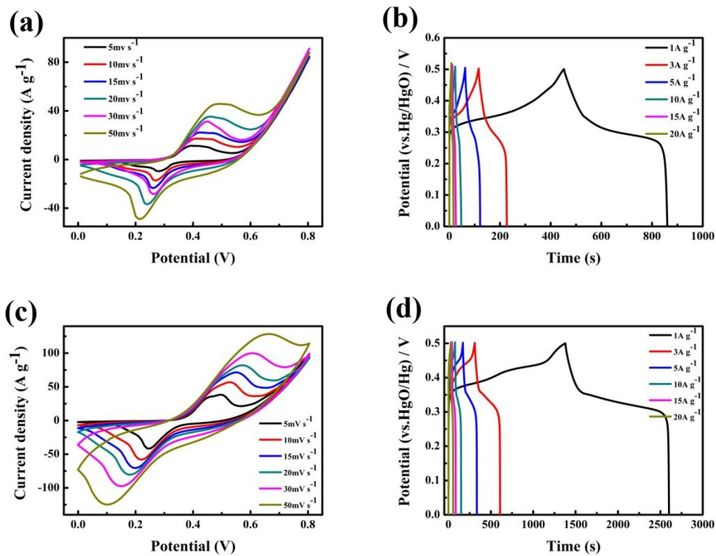
Figure S4. CV curves and GCD curves of the typical Co-Ni-DH (a-b) and Co-Ni-S (c-d).
