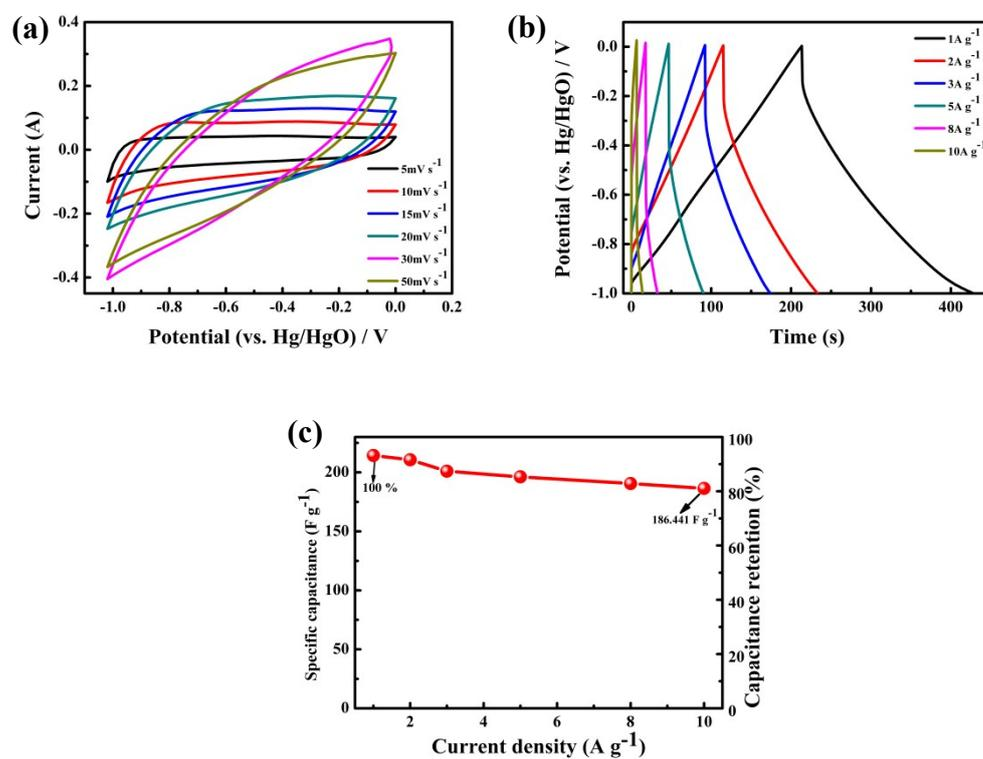
**Figure S7.** (a) the CV measurements of AC electrode at different scan rates from 5 to 50  $\text{mV s}^{-1}$ ; (b) GCD curves of AC electrode at the current densities of 1, 2, 3, 5, 8 and 10  $\text{A g}^{-1}$ ; (c) specific capacitance of AC electrode.
