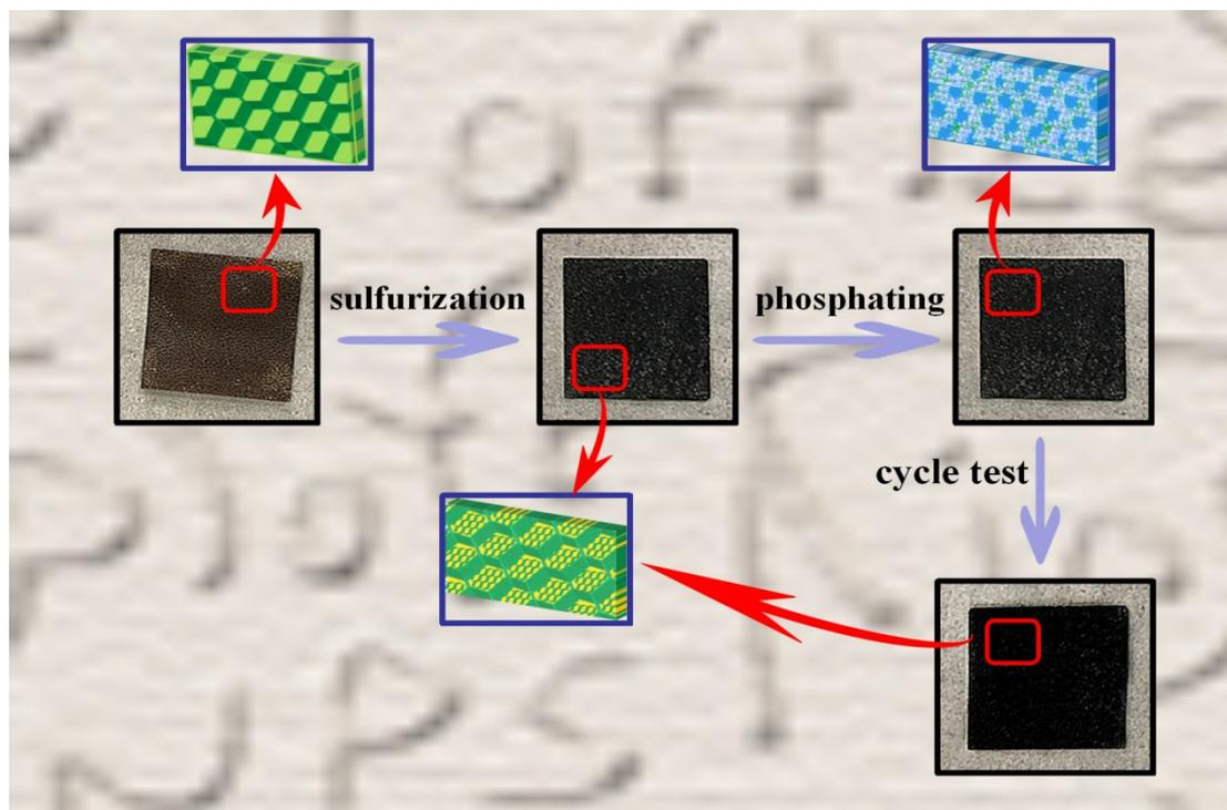
**Figure S1.** Photographs of the as-prepared different electrode materials.
