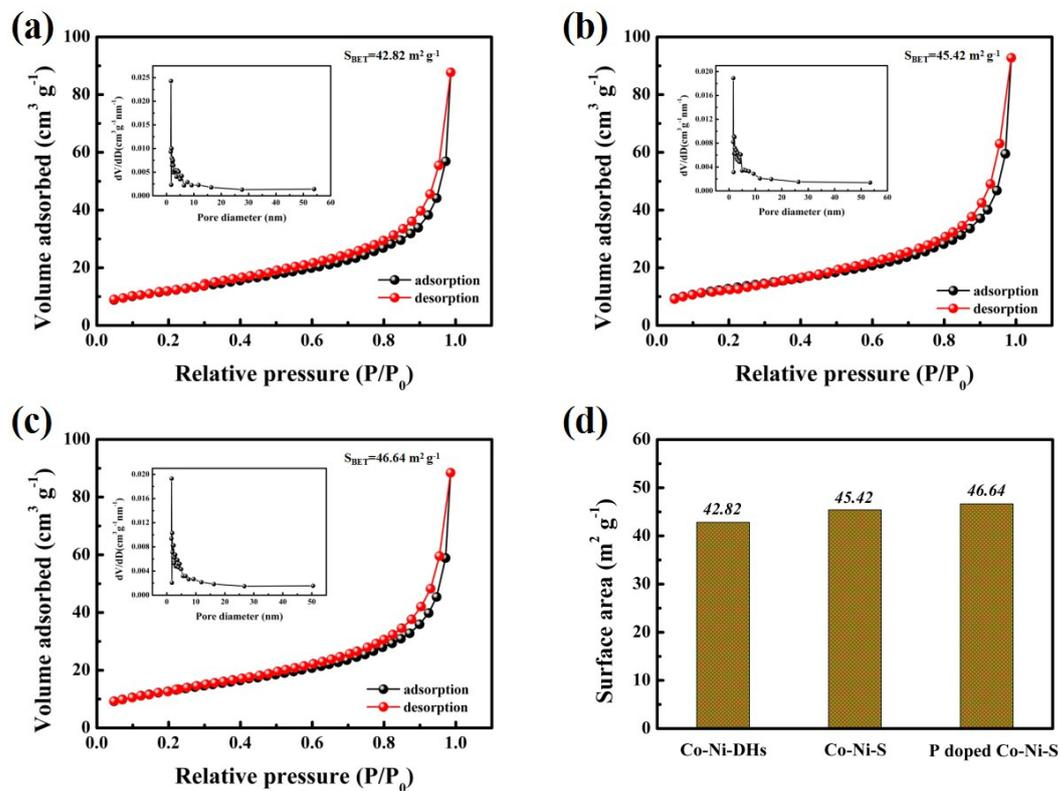
**Figure S3.**  $N_2$  adsorption–desorption analysis of (a) Co-Ni-DHs (b) Co-Ni-S and (c) P doped Co-Ni-S. Insets show the corresponding pore size distribution profiles, (d) the surface area contrast of as-prepared materials.
