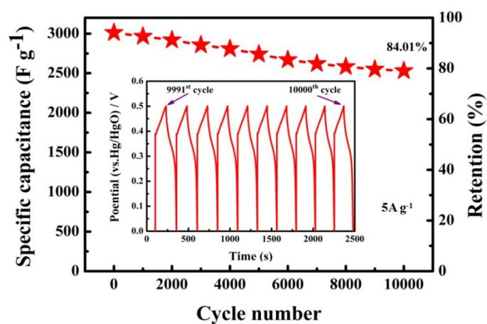
**Figure S6.** The cycling performance of P doped Co-Ni-S electrode at a constant current density of 5 A g<sup>-1</sup>.
