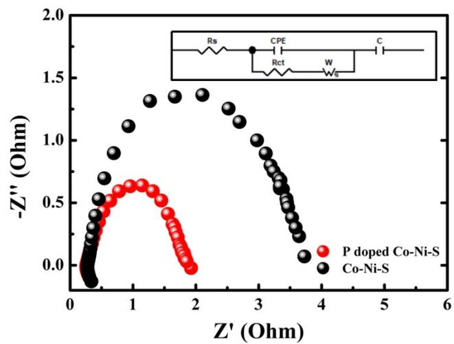
**Figure S5.** EIS in the frequency of 0.01Hz~100KHz and the equivalent circuit model for the EIS plot of Ni-Co-S and P doped Co-Ni-S.
