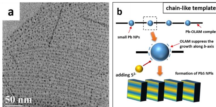
**Figure S6.** (a) TEM image of Pb-OLAM complex. (b) A schematic illustration of template-assistant growth of PbS NPs.
