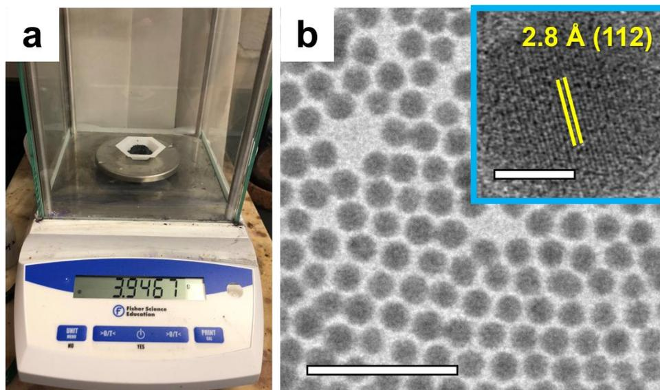
**Figure S1.** (a) Photograph of Ag<sub>2</sub>S NP powders produced by large-scale synthesis in a single batch. Based on ICP-OES results, the yield of the product Ag<sub>2</sub>S is 95.1% relative to the amount of Ag precursor provided. (b) TEM image of Ag<sub>2</sub>S NPs from scaled up synthesis. The inset shows an HRTEM image of a single Ag<sub>2</sub>S NP. The scale bars in the main panel and inset are 50 nm and 5 nm, respectively.
