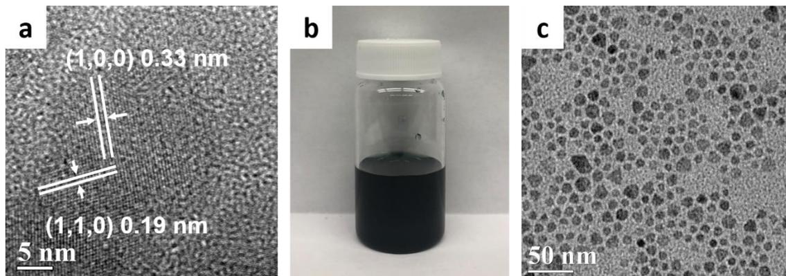
**Figure S5.** (a) HRTEM image of top view CuS NPIs. (b) Photograph of Cu-OAm precursor produced using CuCl. The dark green color of the solution indicates formation of Cu(II) species. (c) TEM image of CuS NPIs synthesized using CuCl.
