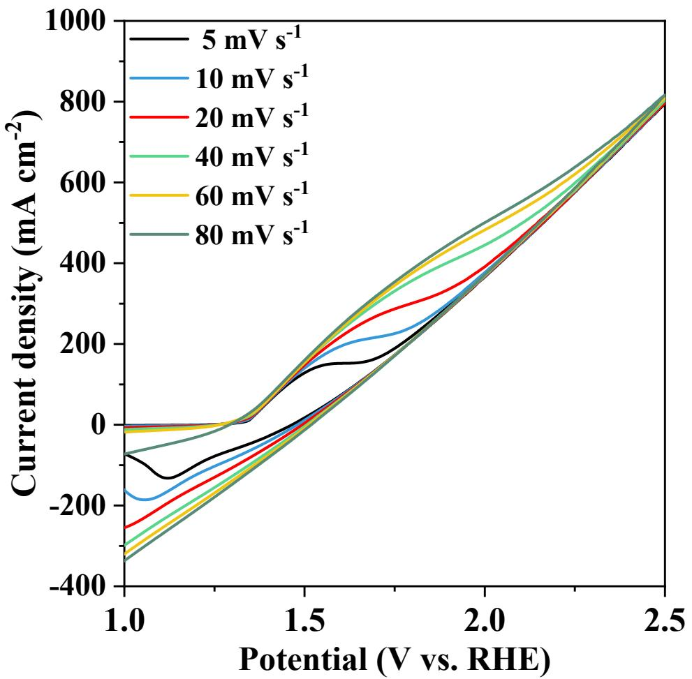
Figure S15. OER performance of  $\text{Ni}(\text{PO}_3)_2\text{-MoO}_3/\text{NF}$  in different scan rates.
