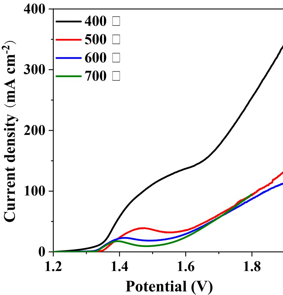
Figure S7. Polarization curves for OER of  $\text{Ni}(\text{PO}_3)_2\text{-MoO}_3/\text{NF}$  from different phosphating temperature.
