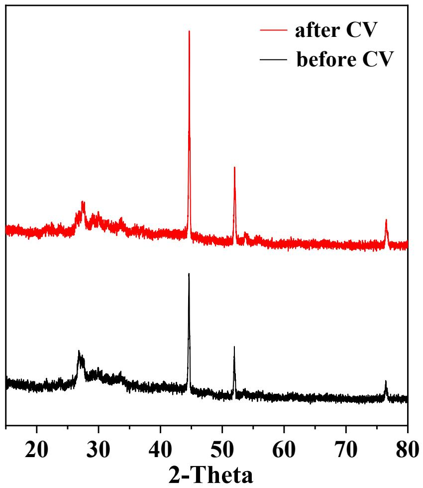
Figure S11. XRD patterns of  $\text{Ni}(\text{PO}_3)_2\text{-MoO}_3/\text{NF}$  before and after stability test.
