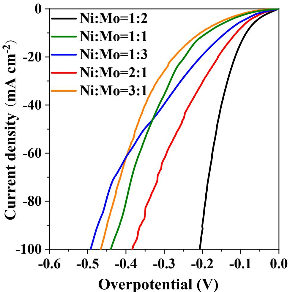
Figure S6. Polarization curves for HER of  $\text{Ni}(\text{PO}_3)_2\text{-MoO}_3/\text{NF}$  from different proportion of Mo and Ni by adjusting synthesis quantity of metal precursor.
