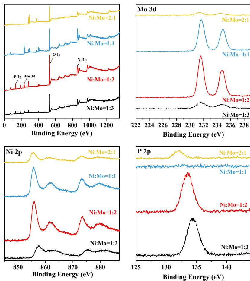
Figure S13. XPS spectrum of  $\text{Ni}(\text{PO}_3)_2\text{-MoO}_3/\text{NF}$  from different ratio of Ni:Mo.
