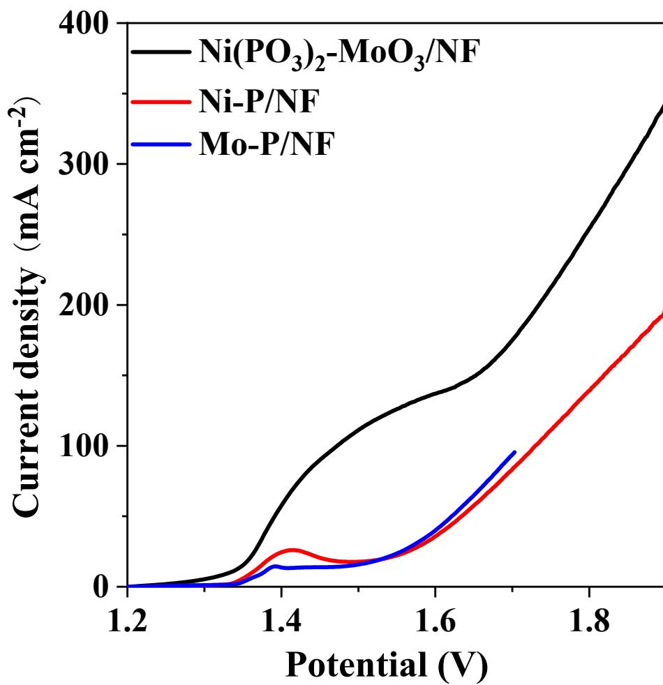
Figure S8. Polarization curves for OER of  $\text{Ni}(\text{PO}_3)_2\text{-MoO}_3/\text{NF}$ ,  $\text{Ni-P}/\text{NF}$  and  $\text{Mo-P}/\text{NF}$ .
