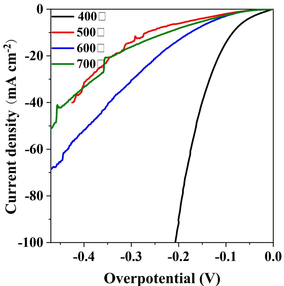
Figure S4. Polarization curves for HER of  $\text{Ni}(\text{PO}_3)_2\text{-MoO}_3/\text{NF}$  from different phosphating temperature.
