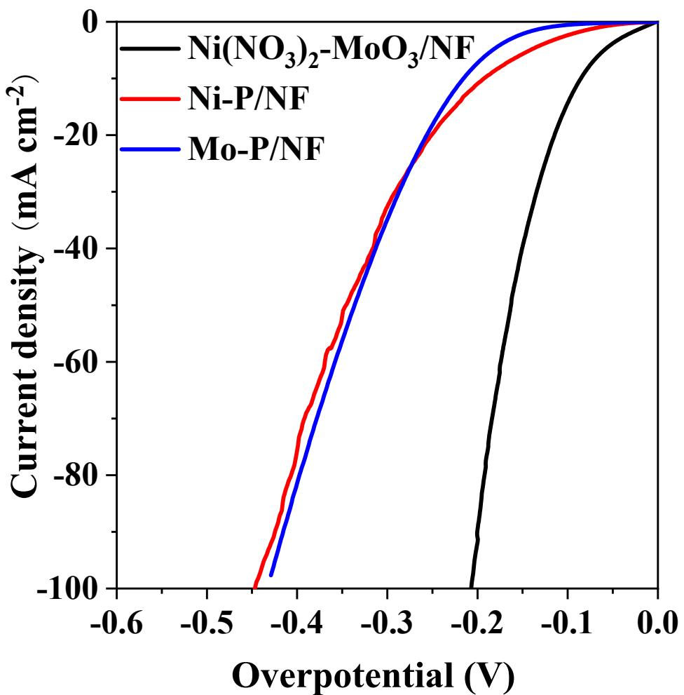
Figure S5. Polarization curves for HER of  $\text{Ni}(\text{PO}_3)_2\text{-MoO}_3/\text{NF}$ , Ni-P/NF and Mo-P/NF.
