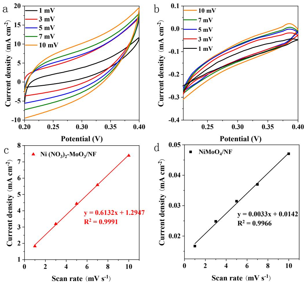
Figure S10. CV curves at different scan rates of (a)  $\text{Ni}(\text{PO}_3)_2\text{-MoO}_3/\text{NF}$  and (b)  $\text{NiMoO}_4/\text{NF}$ . The capacitive currents of (c)  $\text{Ni}(\text{PO}_3)_2\text{-MoO}_3/\text{NF}$  and (d)  $\text{NiMoO}_4/\text{NF}$  are measured at 0.30 V vs. RHE plotted as a function of scan rate.
