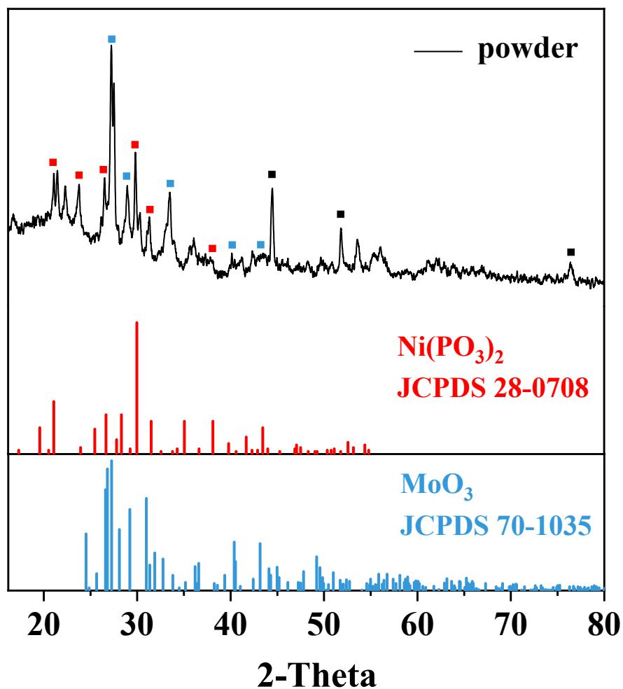
Figure S14. XRD patterns of  $\text{Ni}(\text{PO}_3)_2$ - $\text{MoO}_3$  powder.
