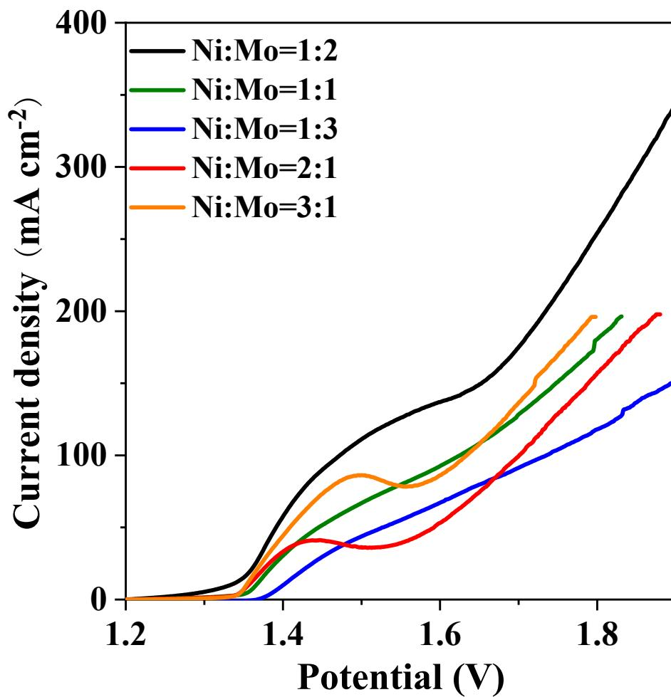
Figure S9. Polarization curves for OER of  $\text{Ni}(\text{PO}_3)_2\text{-MoO}_3/\text{NF}$  from different proportion of Mo and Ni by adjusting synthesis quantity of metal precursor.
