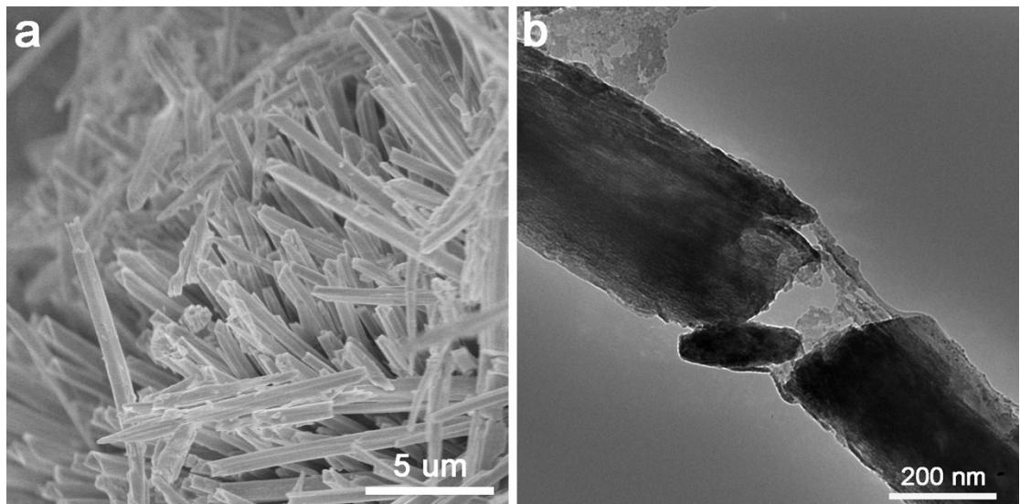
Figure S2. SEM image (a) and TEM images (b) of  $\text{Ni}(\text{PO}_3)_2\text{-MoO}_3/\text{NF}$ .
