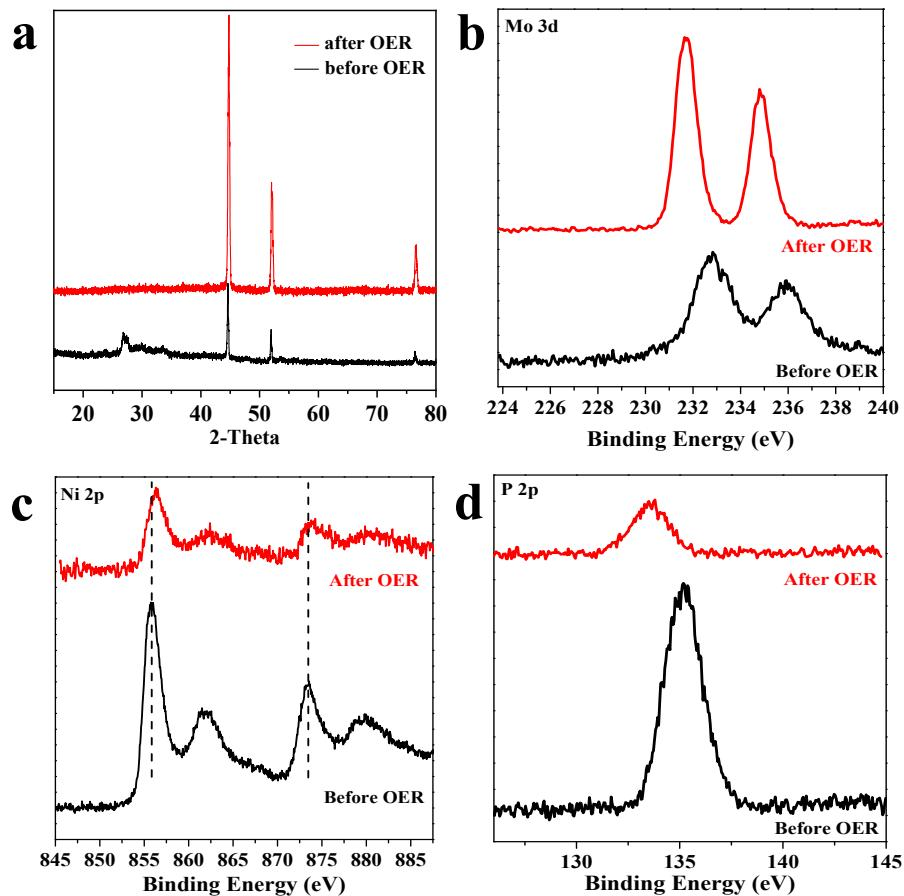
Figure S17. (a) XRD patterns and (b-d) XPS spectrum of  $\text{Ni}(\text{PO}_3)_2\text{-MoO}_3/\text{NF}$  after OER.
