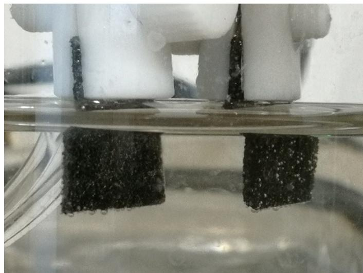
Figure S12. The photograph of bubbles during the water splitting tests.
