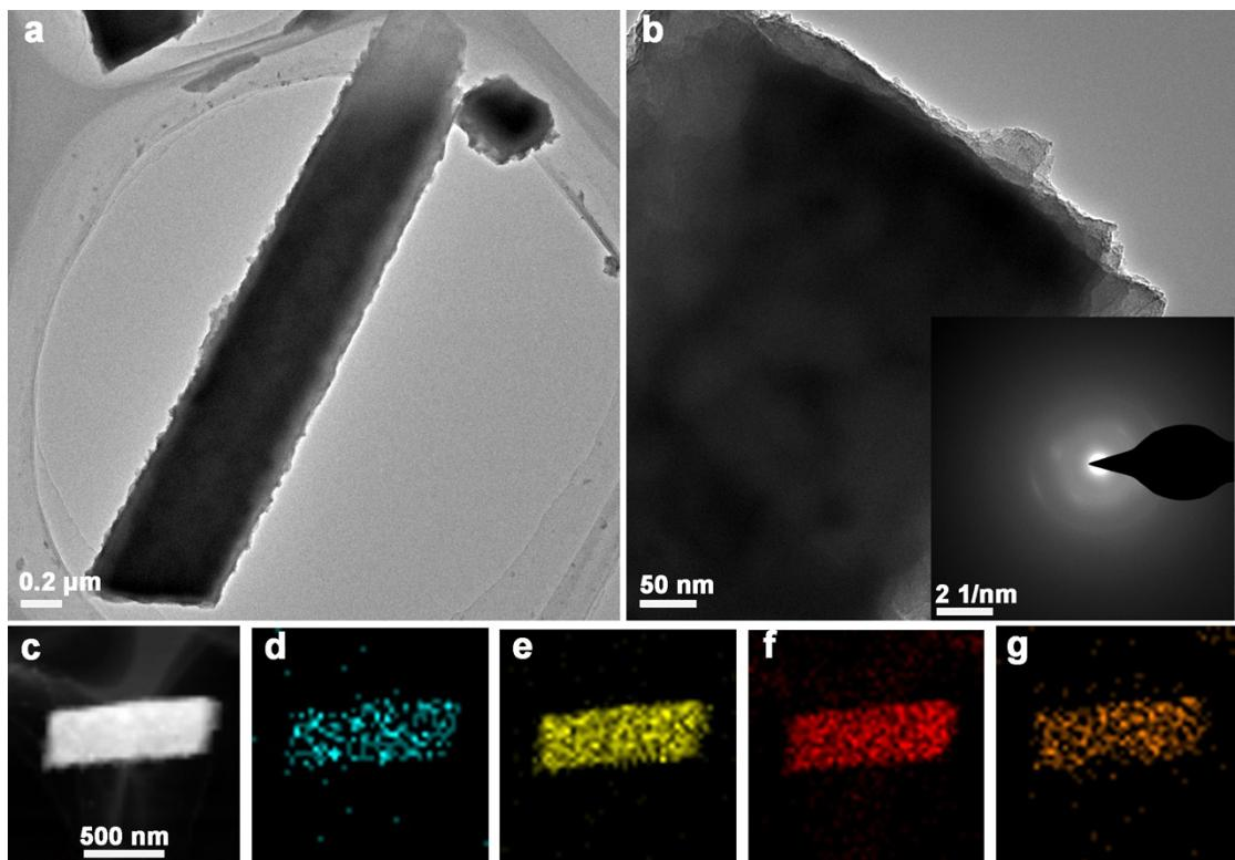
Figure S16. (a) TEM image, (b) HRTEM image and (c-g) STEM mapping images of  $\text{Ni}(\text{PO}_3)_2\text{-MoO}_3/\text{NF}$  after OER. The inset in (b) shows the corresponding SAED patterns.
