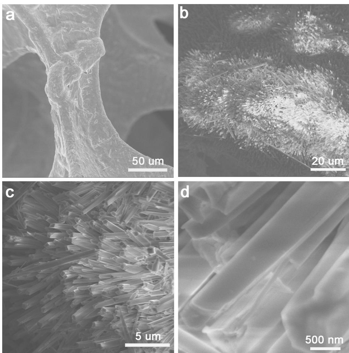
Figure S1. SEM images of (a) bare nickel foam and (b-d)  $\text{NiMoO}_4/\text{NF}$ .
