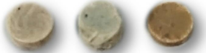
**S11** Image of ND pellets after first air etching (left), directly after irradiation (middle), after irradiation and post-treatment.
