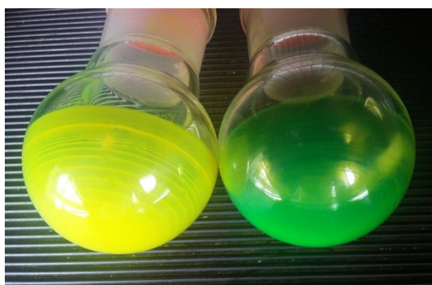
Figure S4. As-prepared (left) and purified (right) \text{CsPbBr}_3 NCs samples in the solid state after three weeks storage under ambient conditions and room light.
