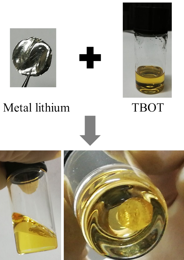
Fig. S3 Phenomenons of the chemical reactions between lithium and TBOT. Bubbles were hydrogen generated from the reaction between H_2O and lithium.
