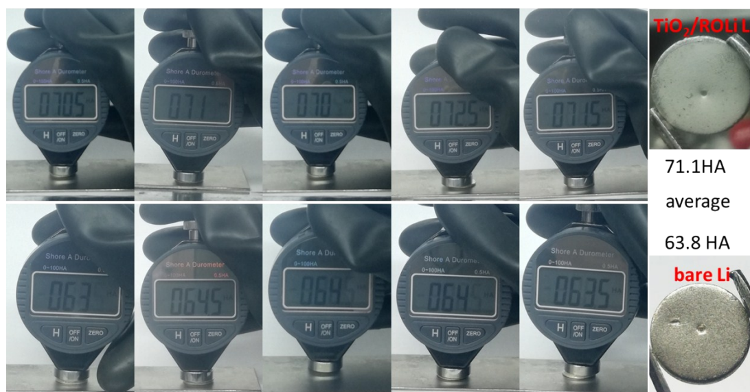
Fig. S4 Hardness measurement results of the TiO_2/ROLi-Li and bare Li electrode with a Shore A
