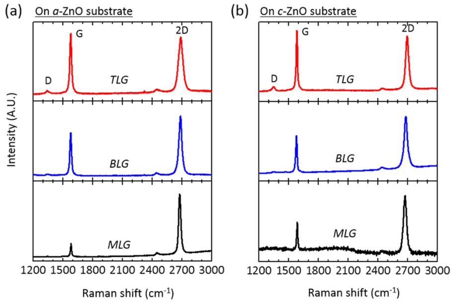
**Figure S1.** Raman spectra for MLG (bottom), BLG (middle), and TLG (top) layers coated on (a)  $\alpha$ -ZnO and (b)  $c$ -ZnO substrates after remote epitaxy of ZnO overlayer.
