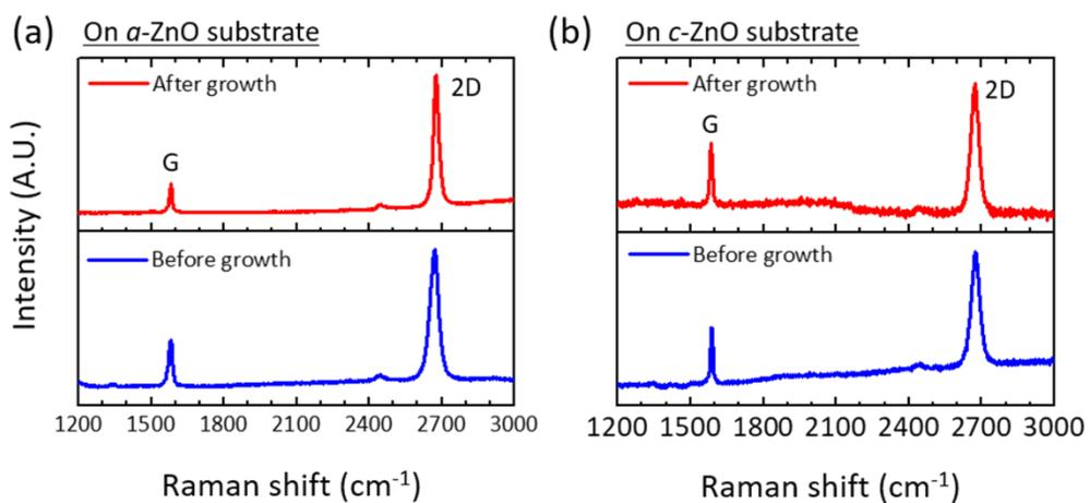
**Figure S2.** Raman spectra for MLG coated on (a)  $\alpha$ -ZnO and (b)  $c$ -ZnO substrates. Bottom blue lines are the spectra obtained before hydrothermal growth of ZnO MRs, and red ones are after hydrothermal growth of ZnO MRs.
