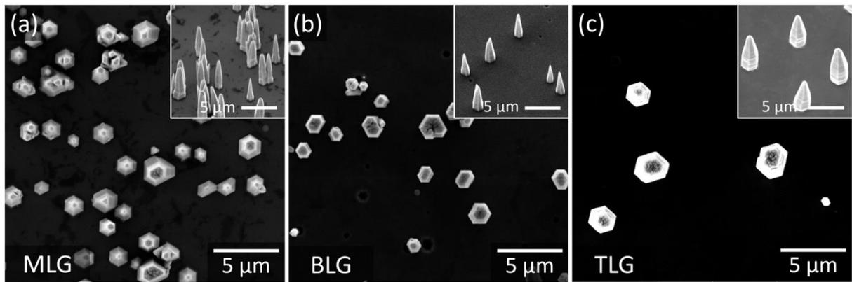
**Figure S6.** Regeneration of substrate for remote epitaxy of ZnO MRs. Plan-view FE-SEM images of ZnO MR arrays grown on (a) MLG-, (b) BLG-, and (c) TLG-coated *c*-ZnO substrates. Insets are tilt-view FE-SEM images.
