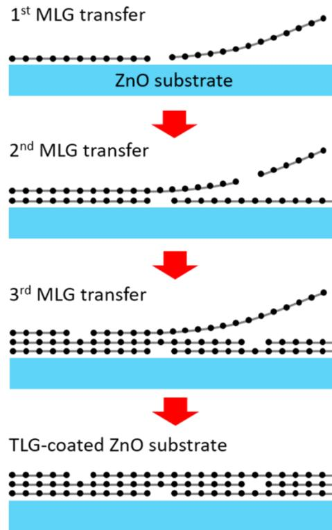
**Figure. S4.** Schematic illustrations for preparation of graphene-coated ZnO substrate. For BLG and TLG-coated substrates, the transfer of MLG was repeated with respect to the number of graphene layers. This substrate preparation method remarkably reduces the presence of small opening defect of graphene that may induce the homoepitaxial nucleation and growth of ZnO directly via the opening defects.
