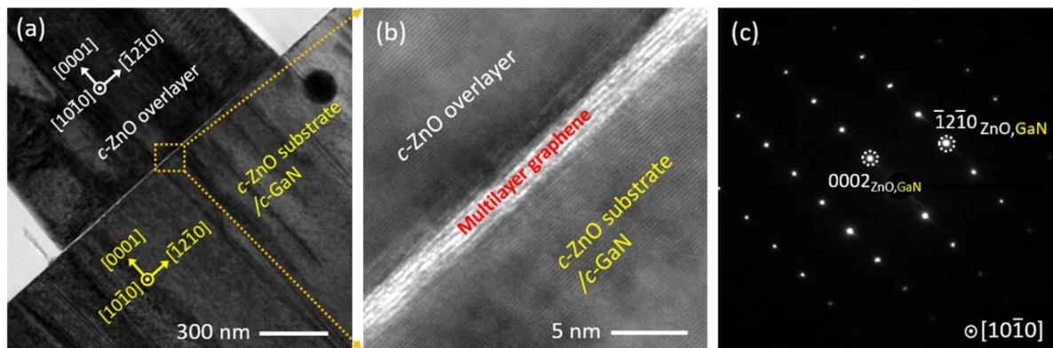
**Figure S3.** Cross-sectional TEM analyses for remote epitaxial *c*-ZnO/multilayer graphene/*c*-ZnO heterostructure. (a) Low-magnification TEM image and (b) the corresponding HR-TEM image enlarged from boxed area of (a). (c) Electron diffraction patterns of *c*-ZnO MR/graphene/*c*-ZnO substrate.
