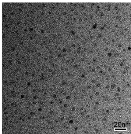
**Fig. S3.** Transmittance electron microscopy (TEM) images of the Den-Cy5.5/Pt.
