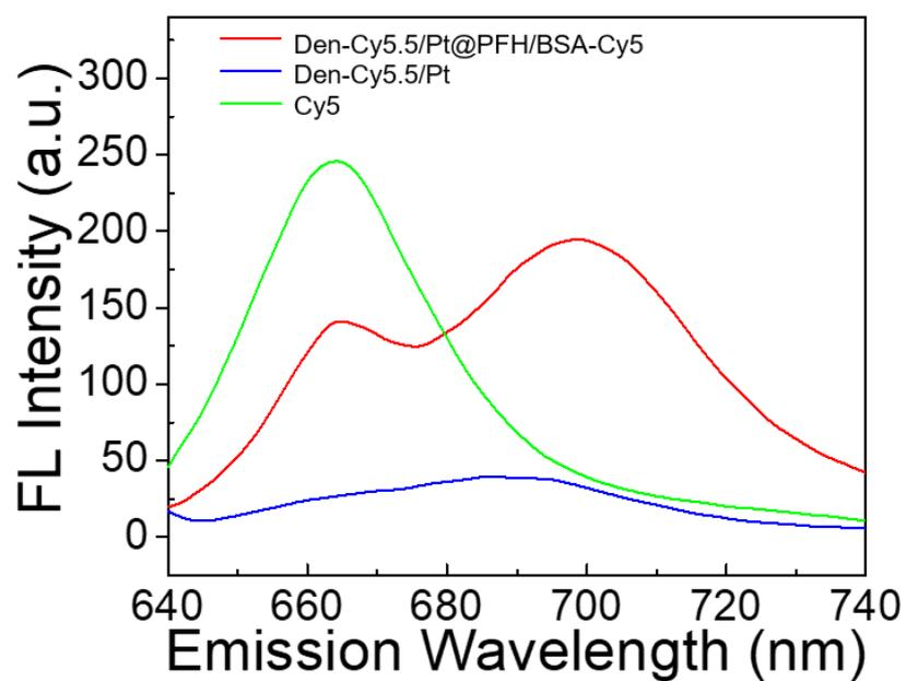
**Fig. S6.** The fluorescence spectra of Den-Cy5.5/Pt@PFH/BSA-Cy5 (red line), BSA-Cy5 (green line) and Den-Cy5.5/Pt (blue line). The excitation wavelength is 640 nm.
