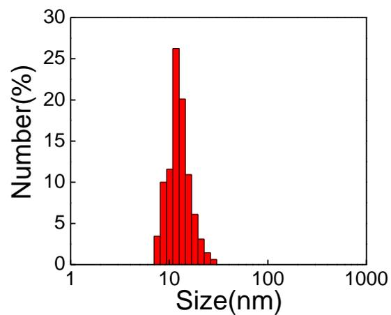
**Fig. S4.** Dynamic light scattering (DLS) measurements of the size and distribution of the Den-Cy5.5/Pt.
