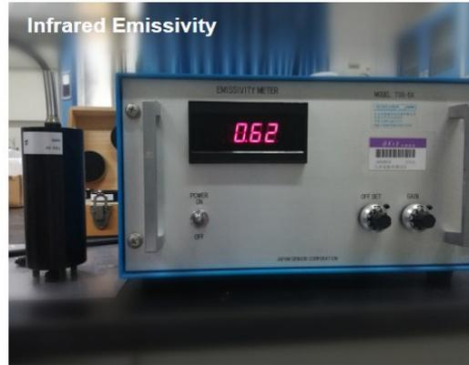
**Fig. S10.** Photograph of emissivity meter, exhibiting a low infrared emissivity of 0.62.
