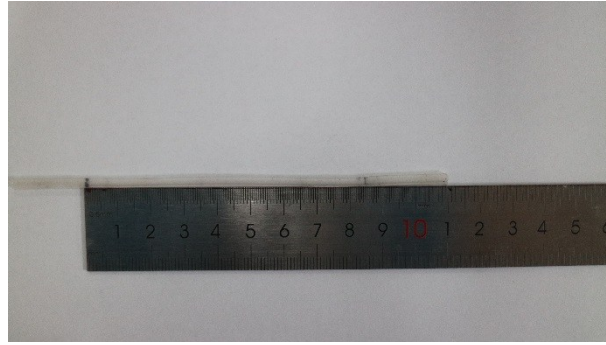
Fig. S2 Residual strain of the silicone tube after near 700% elongation test.
