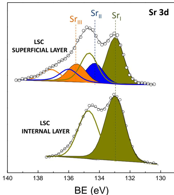
**Figure S2.** Sr 3d region of the photoelectron spectra for the superficial and internal LSC layer of the the 50nm-[LSC/CGO]<sub>N=2</sub> heterostructure (without CGO termination).
