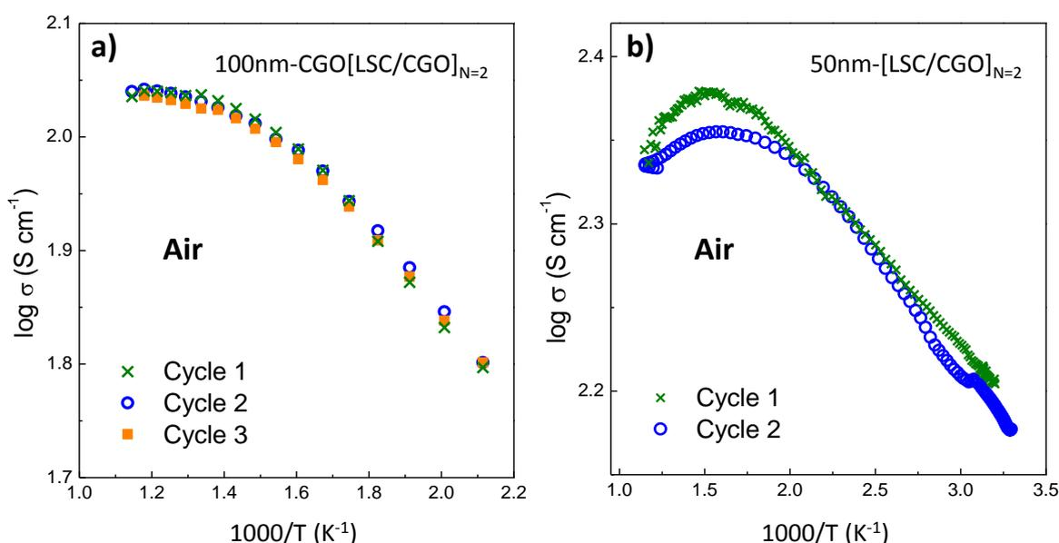
**Figure S1.** Arrhenius plot of (a) 100nm-CGO[LSC/CGO]<sub>N=2</sub> and (b) 50nm-CGO[LSC/CGO]<sub>N=2</sub> heterostructures measured in air after different thermal cycles of ca. 10 hours in the RT-600 °C temperature range.
