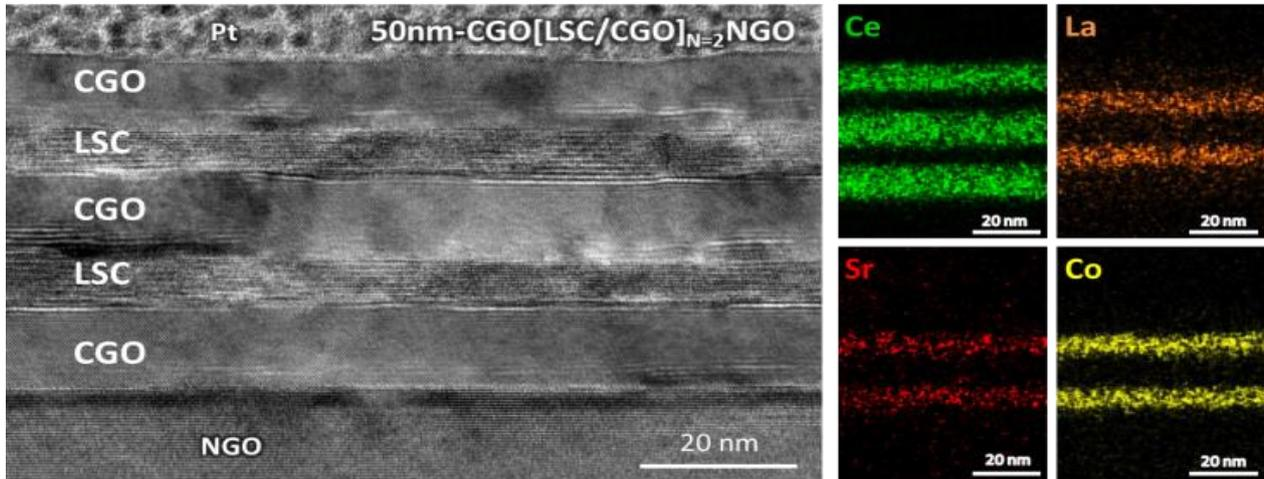
**Figure S3.** Cross section HR-TEM micrograph and EDS elemental mapping of the 50nm-CGO[LSC/CGO]<sub>N=2</sub>NGO heterostructure after thermal cycles (aged sample/post mortem). The Pt protective layer (top-layer in Figure) was deposited by focused ion beam (FIB) to the area of interest prior to ion beam milling in order to preserve the sample and avoid ion beam damage during lamella preparation.
