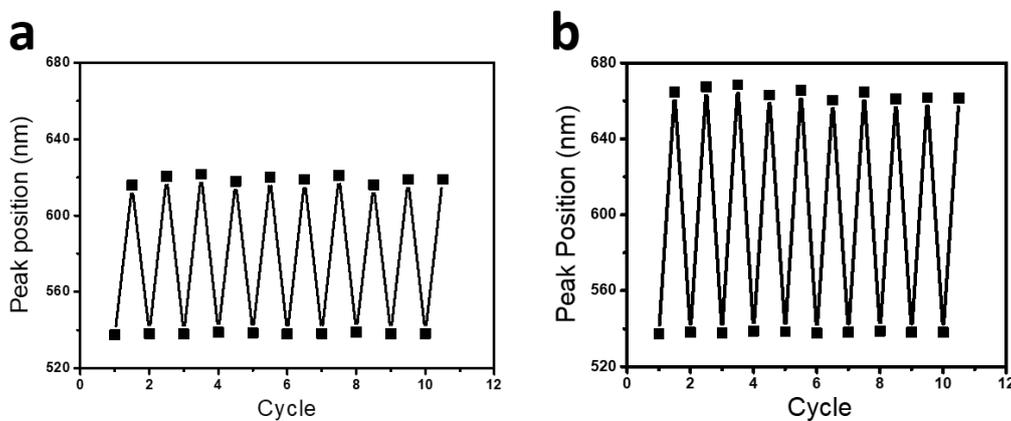
**Figure S4.** Reproducible ethanol/water vapor sensing with response time of a) 5 min and b) 15 min of the fiber optic sensor. The ethanol vapor sensor is fully reversible
