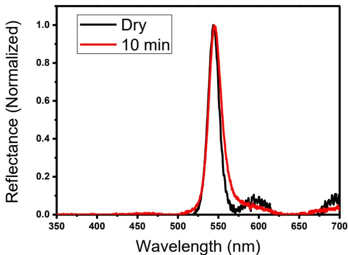
**Figure S5.** Reflection spectra of the PC film at normal incidence before and after being immersed in pure *n*-octane for 10 min.
