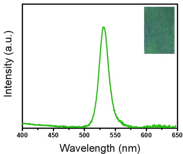
**Figure S6.** Reflection spectra and picture of the PC film which consisted of PS particles and styrene. The mass fraction of PS particles is 45%.
