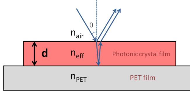
**Figure S1.** Schematic illustration of thin-film interference. Light reflected by the lower and upper boundaries interfere with one another.
