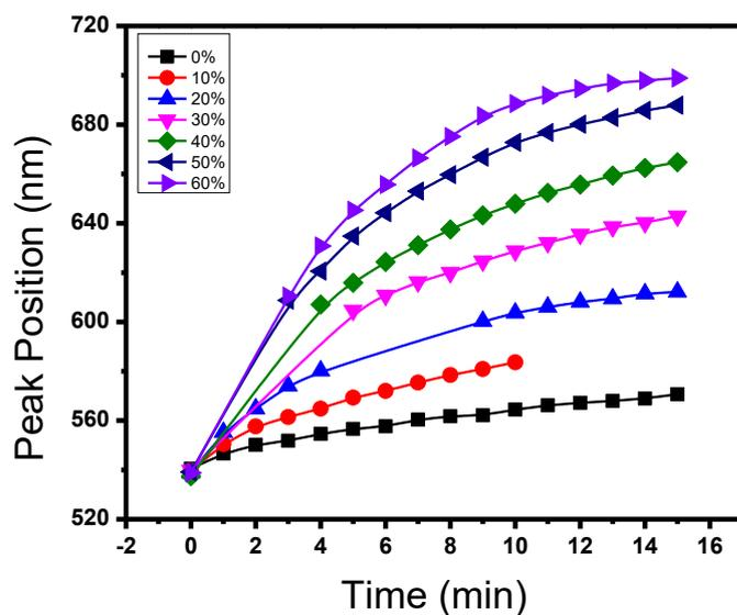
**Figure S3.** Correlation of the peak position of the reflection spectra and the response time with different ethanol concentrations which were detected by fiber optic sensor.
