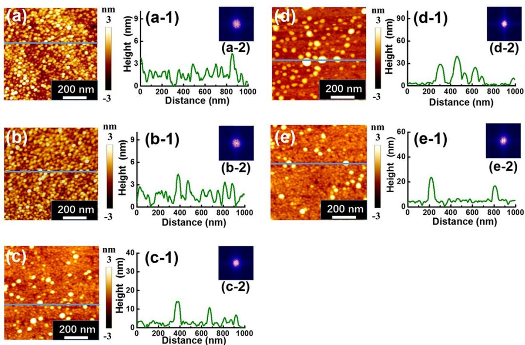
**Fig. S1** Annealing temperature effect on the fabrication of the self-assembled stalagmite-shaped Al nanoparticles (NPs) with an identical deposition thickness of 6 nm. (a) - (e) Atomic force microscope (AFM) top views of the samples with a size of  $1 \times 1 \mu\text{m}^2$ . (a-1) - (e-1) The cross-sectional line-profiles obtained from the blue lines drawn in AFM top-views. (a-2) - (e-2) 2D fast Fourier transform (FFT) spectra of the samples.
