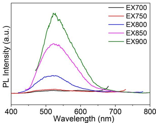
**Fig. S6** Up-conversion PL properties of the prepared NCDs at different excitation wavelength length.
