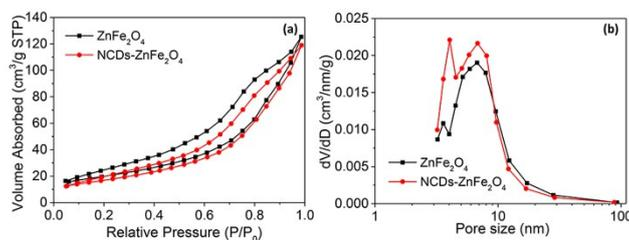
**Fig. S4** N<sub>2</sub> adsorption-desorption isotherms (a) and pore-size distribution (b) of ZnFe<sub>2</sub>O<sub>4</sub> yolk-shell and NCDs-ZnFe<sub>2</sub>O<sub>4</sub> yolk-shell structure.
