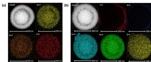
**Fig. S2** HAADF-STEM image and element mapping images of ZnFe<sub>2</sub>O<sub>4</sub> yolk-shell (a) and NCDs-ZnFe<sub>2</sub>O<sub>4</sub> yolk-shell photocatalysts (b).
