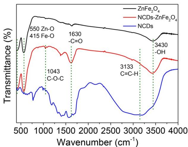
**Fig. S3** FTIR spectra of NCDs, ZnFe<sub>2</sub>O<sub>4</sub> and NCDs-ZnFe<sub>2</sub>O<sub>4</sub>.
