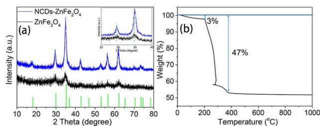
**Fig. S1** (a) XRD patterns of ZnFe<sub>2</sub>O<sub>4</sub> and CN-ZnFe<sub>2</sub>O<sub>4</sub>. Inset: high-resolution spectrum in range of 2θ from 25 to 40 °. (b) TGA profile of Zn-Fe glycerinate under air flow.
