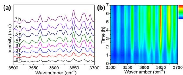
**Fig. S7** *In situ* FTIR spectra of gaseous *o*-DCB during photocatalytic process (a) and corresponding time-domain IR spectra (b) in the wavenumber region of 3500-3700  $\text{cm}^{-1}$ .
