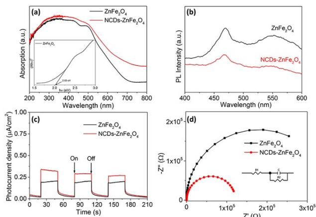
**Fig. S5** (a) UV-vis diffuse reflectance spectra (inset: estimated band gap of pure  $\text{ZnFe}_2\text{O}_4$ ) (b) photoluminescence emission spectra (excitation wavelength: 325 nm) (c) Photocurrent response under visible light and (d) EIS Nyquist plot of NCDs- $\text{ZnFe}_2\text{O}_4$  and  $\text{ZnFe}_2\text{O}_4$ .
