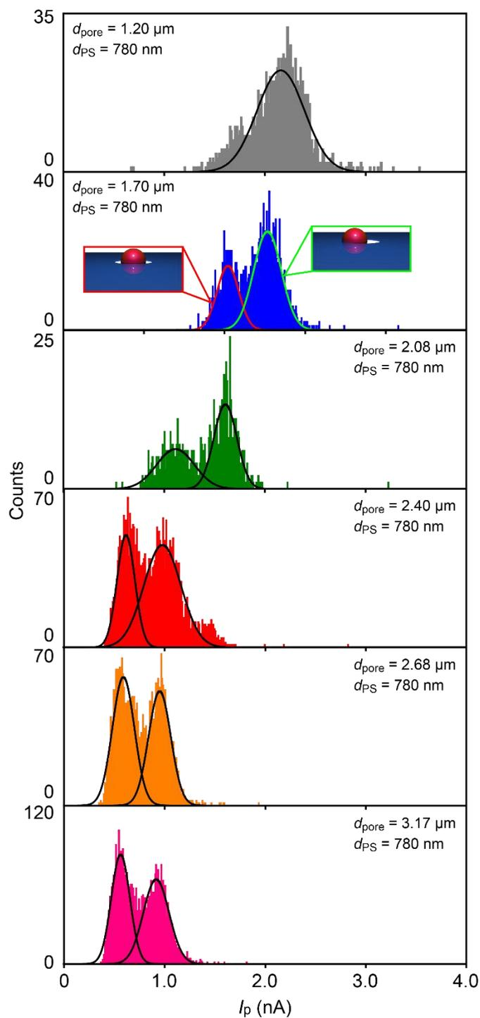
**Figure S12.** Histograms of the resistive pulse height  $I_p$  obtained for 900 nm-sized carboxylated polystyrene beads in 0.2 x PBS under 0.1 V with single pores having equivalent area to those of 1.2  $\mu\text{m}$ -sized one- (grey), two- (blue), three- (green), four- (red), five- (orange), and seven-pores (pink) in a 50 nm thick  $\text{Si}_3\text{N}_4$
