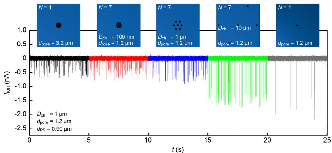
**Figure S3.** Partial ionic current ( $I_{ion}$ ) traces obtained for 900 nm-sized carboxylated polystyrene beads in 0.2 x PBS with seven-pores of various inter-channel distance  $D_{ch}$ . As the inter-channel distance  $D_{ch}$  becomes shorter, the pulse height tends to be weaker and become comparable to those observed in the equivalent-size single-pore (black).
