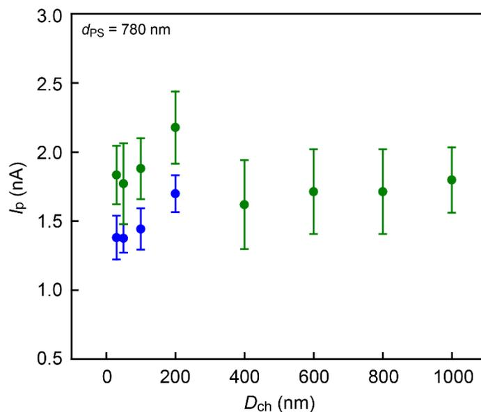
**Figure S9.** Dependence of the resistive pulse height  $I_p$  of 780 nm-sized polystyrene beads in 0.2 x PBS under 0.1 V on the number of 1.2  $\mu$ m-sized double pores of variable inter-channel distance  $D_{ch}$ . Error bars denote the full width at half maximum of Gaussian distributions fit to the  $I_p$  histograms.
