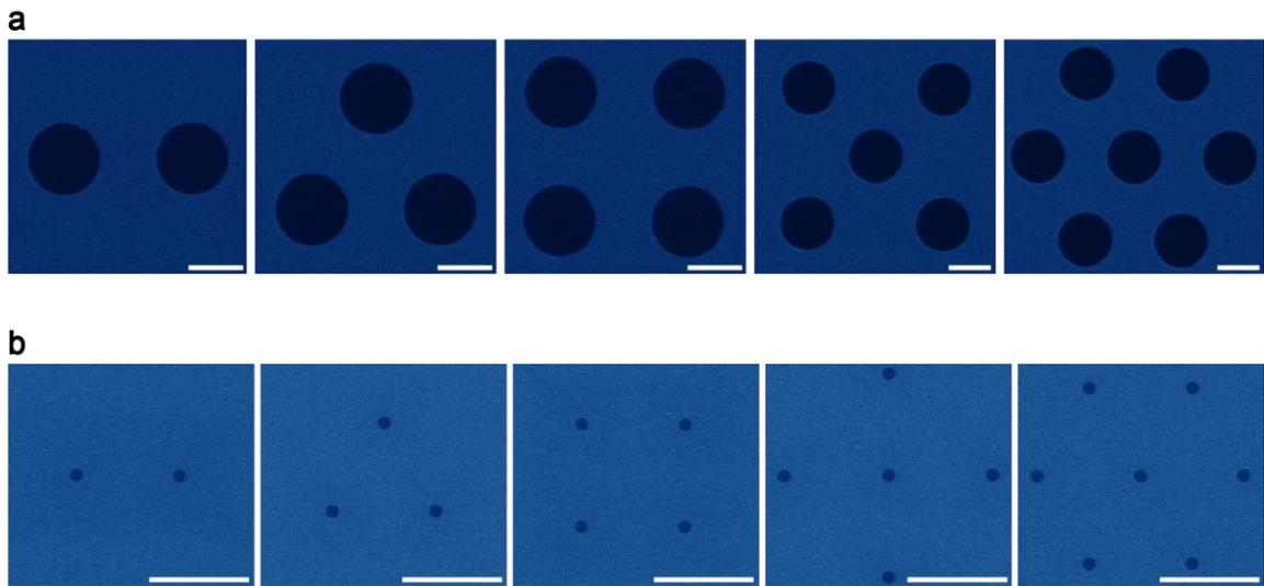
**Figure S1.** **a-b**, False-colored scanning electron microscopy images of multipores with inter-pore distance  $D_{ch}$  of 1  $\mu\text{m}$  (a) and 10  $\mu\text{m}$  (b). Bars denote 1  $\mu\text{m}$  and 10  $\mu\text{m}$ , respectively, in (a) and (b).
