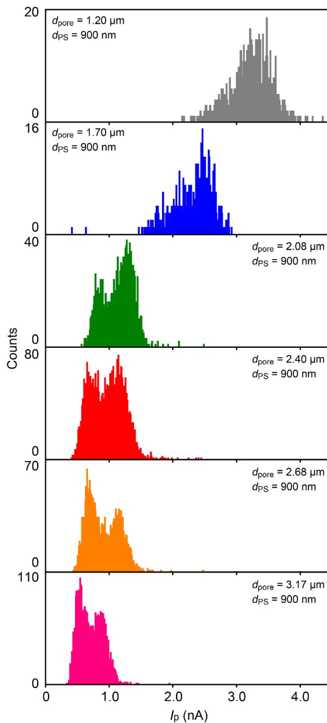
**Figure S11.** Histograms of the resistive pulse height  $I_p$  obtained for 780 nm-sized carboxylated polystyrene beads in 0.2 x PBS under 0.1 V with single pores having equivalent area to those of 1.2  $\mu\text{m}$ -sized one- (grey), two- (blue), three- (green), four- (red), five- (orange), and seven-pores (pink) in a 50 nm thick  $\text{Si}_3\text{N}_4$  membrane. Note that the distributions start to show additional peak at lower  $I_p$
