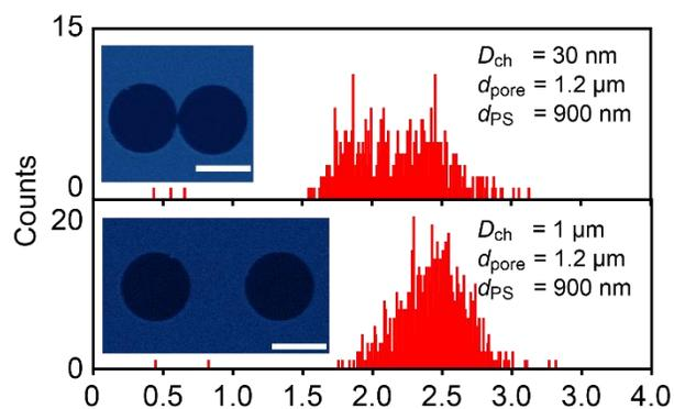
**Figure S8.** Resistive pulse height ( $I_p$ ) histograms obtained for carboxylated polystyrene nanoparticles of diameter  $d_{PS} = 900$  nm in 0.2 x PBS with 1.2  $\mu$ m-sized double-pores of inter-channel distance  $D_{ch} = 30$  nm (top) and 1000 nm (bottom). A bimodal distribution was obtained with  $D_{ch} = 30$  nm while that with  $D_{ch} = 1$   $\mu$ m demonstrates a single-peak profile. Bin size is 0.01 nA.
