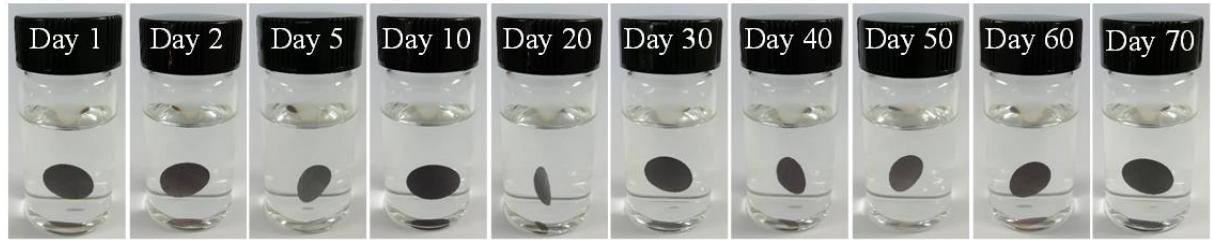
**Fig. S9.** The photographs for the long-term durability and stability of the  $\text{Ti}_3\text{C}_2\text{T}_x$  foam in electrolyte.
