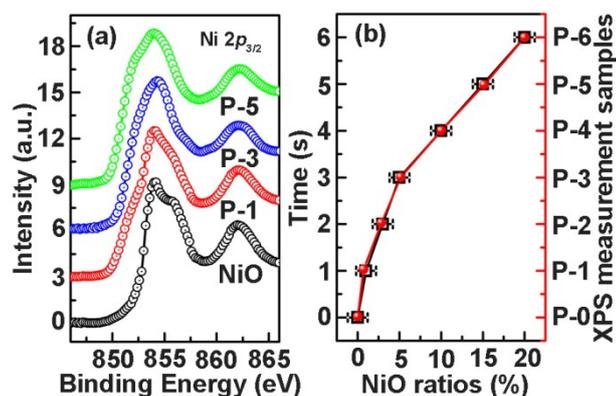
**Figure S1.** (a) Ni  $2p_{3/2}$  spectra for the pure NiO films, P-1, P-3, P-5 nanocolumnar composites. (b) NiO composite ratio versus the deposition time and the XPS data.
