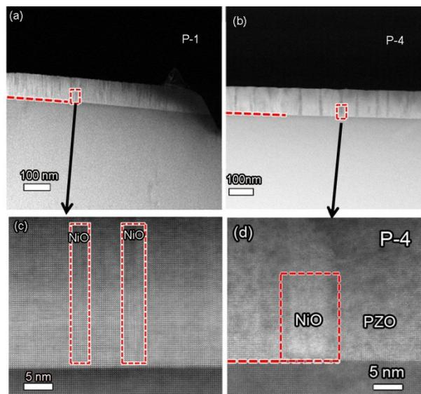
**Figure S2.** (a)-(c) The Low-magnification HAADF images of the P-1 and P-4 nanocolumnars, respectively. (d) High-resolution image of a single NiO nanocolumnar within the PZO matrix for the corresponding nanocolumnar composites.
