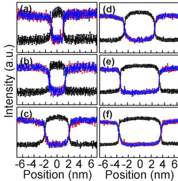
**Figure S3.** (a)-(f) STEM-EDS line scans for Pb, Zr and Ni atom in the interfacial region around the NiO nanocolumnar (the black, red and blue dot represents Ni atom, Pb atom and Zr atom, respectively.) for the P-1, P-2, P-3, P-4, P-5 and P-6 PZO:NiO nanocolumn composites, respectively.
