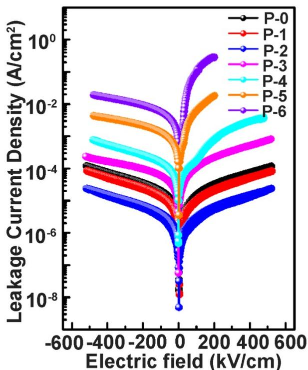
**Figure S4.** (a) The leakage current density of the PZO:NiO nanocomposites with various NiO ratios.
