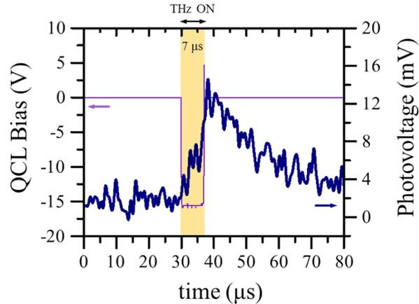
**Figure S2:** sample C, photodetection response time. Time traces of the QCL bias (left vertical axis) and of the photoresponse (right vertical axis). The photovoltage trace is recorded with an oscilloscope. The photoresponse plot represents the raw data, after a pre-amplification stage of 40 dB.
