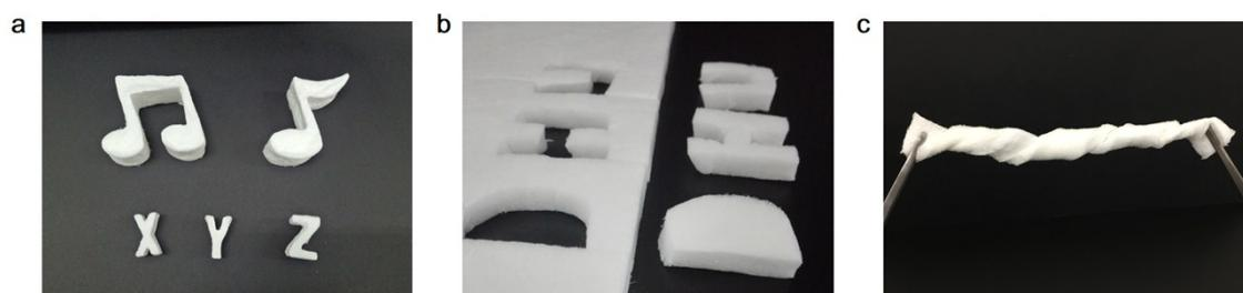
**Fig. S11** The RNFAs can be prepared with designed shape by (a) using various molds or (b) directly cutting from large RNFAs felts. (c) The RNFAs can withstand large distortion such as twist.
