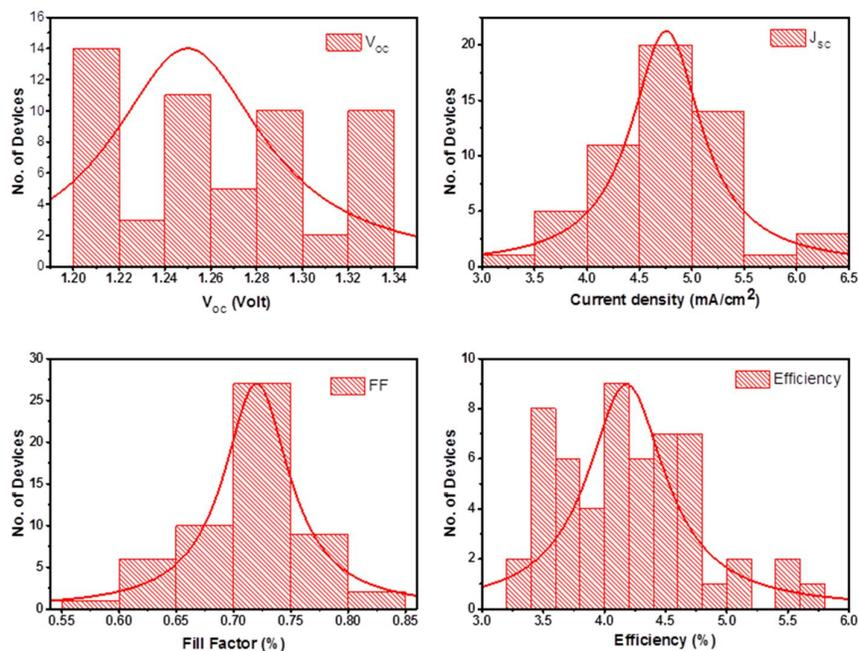
**Figure S5:** Histograms of PV parameters of FTO/d-TiO<sub>2</sub>/mp-TiO<sub>2</sub>/CsPbBr<sub>3</sub>/Hybrid MWCNT electrode.
