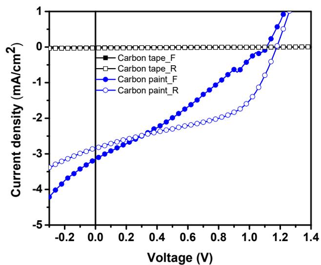
**Figure S3:** J-V characteristics of FTO/d-TiO<sub>2</sub>/mp-TiO<sub>2</sub>/CsPbBr<sub>3</sub>/carbon tape or carbon paint as electrode devices. Filled circle – forward scan and empty circle – reverse scan.
