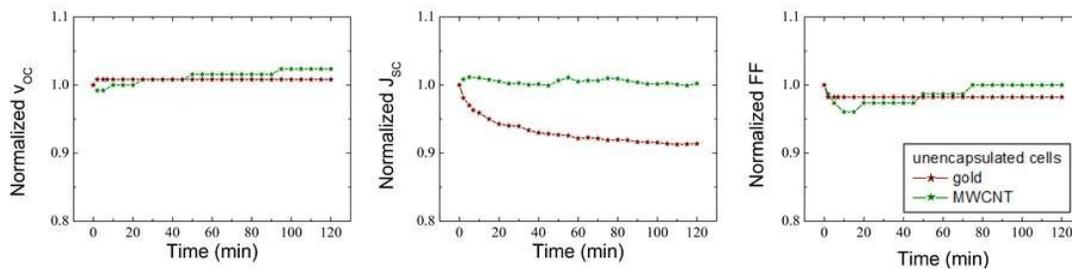
**Figure S10:** Photo-stability under continuous illumination of principal PV parameters of FTO/d-TiO<sub>2</sub>/mp-TiO<sub>2</sub>/CsPbBr<sub>3</sub>/Hybrid MWCNT and gold electrode devices.
