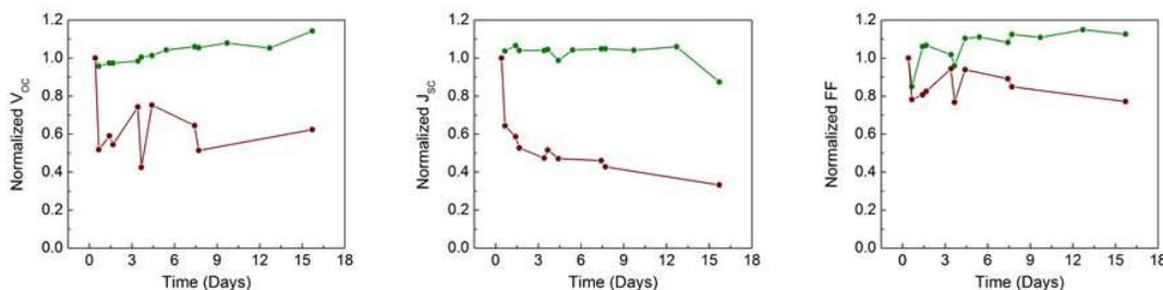
**Figure S11:** Outdoor stability of principal PV parameters of FTO/d-TiO<sub>2</sub>/mp-TiO<sub>2</sub>/CsPbBr<sub>3</sub>/Hybrid MWCNT and gold electrode devices.
