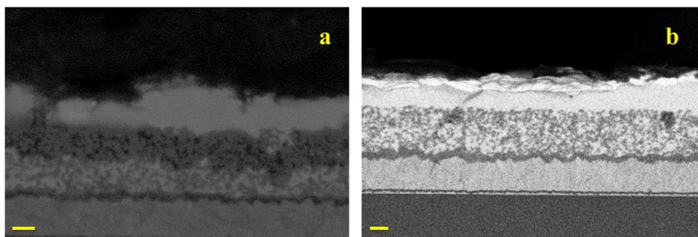
**Figure S2:** cross-sectional SEM images a) FTO/d-TiO<sub>2</sub>/mp-TiO<sub>2</sub>/CsPbBr<sub>3</sub>/Hybrid MWCNT electrode b) FTO/d-TiO<sub>2</sub>/mp-TiO<sub>2</sub>/CsPbBr<sub>3</sub>/Au electrode with Back scattered detector. Scale bar is 200 nm.
