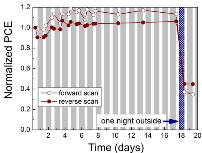
**Figure S14:** The PCE evolution of MWCNT device with day-night cycle during outdoor exposure. The gray areas correspond to nighttime, during which the cells were kept in a desiccant box in the dark. The dramatic degradation on the day 18 is a result of one night outdoor, likely, due to morning dew.
