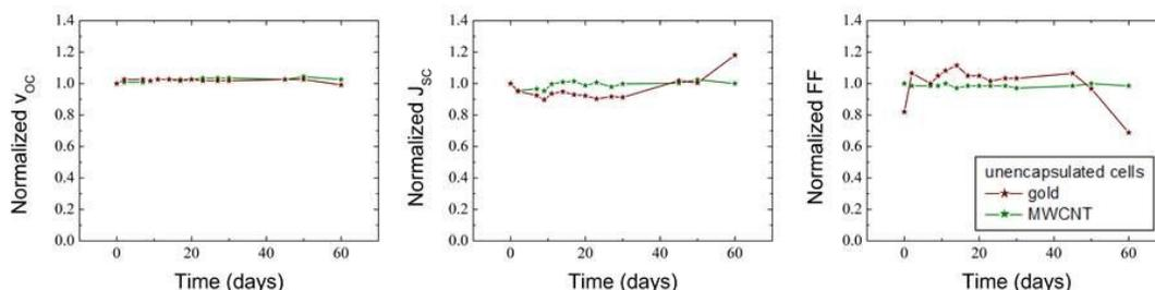
**Figure S8:** “On-shelf” stability studies of FTO/d-TiO<sub>2</sub>/mp-TiO<sub>2</sub>/CsPbBr<sub>3</sub>/Hybrid MWCNT electrode devices.
