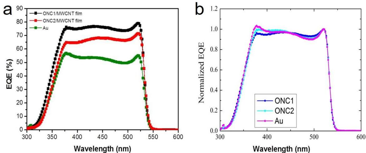
**Figure S4.** (a) EQE spectra measured with FTO/d-TiO<sub>2</sub>/mp-TiO<sub>2</sub>/CsPbBr<sub>3</sub>/back electrode, where the back electrode was ONC1•MWCNT, ONC2•MWCNT or Au. (b) The same normalized to the value at 450 nm.
