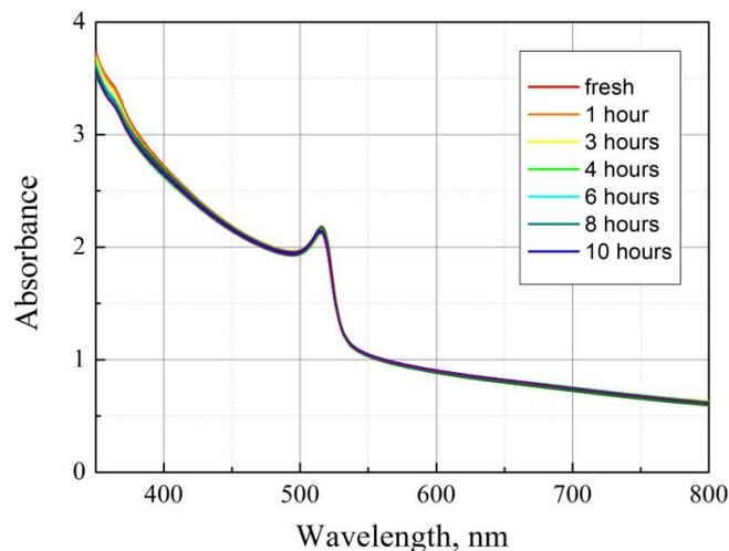
**Figure S7:** Absorption spectra of CsPbBr<sub>3</sub> film after exposure to concentrated sunlight with intensity of 100 suns.
