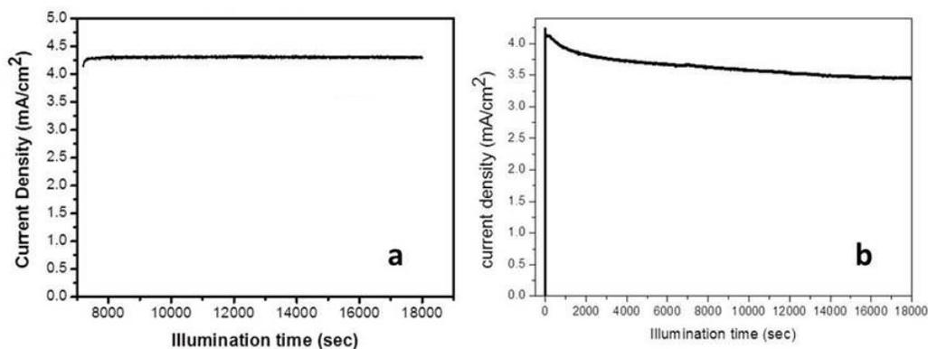
**Figure S12.** Current density evolution upon MPP tracking of (a) FTO/d-TiO<sub>2</sub>/mp-TiO<sub>2</sub>/CsPbBr<sub>3</sub>/Hybrid MWCNT and (b) gold electrode devices.
