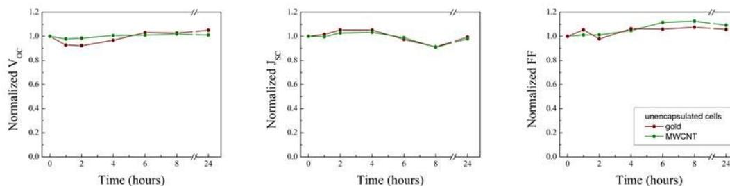
**Figure S9:** Thermal stability of principal PV parameters of FTO/d-TiO<sub>2</sub>/mp-TiO<sub>2</sub>/CsPbBr<sub>3</sub>/Hybrid MWCNT and gold electrode devices.
