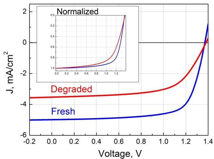
**Figure S15:** The J-V curves of the PSC before and after outdoor aging experiment shown in Figure. 6. The inset shows the same curves normalized to the J<sub>sc</sub> value.
