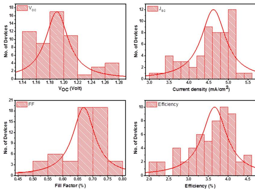
**Figure S6:** Histogram of PV parameters of FTO/d-TiO<sub>2</sub>/mp-TiO<sub>2</sub>/CsPbBr<sub>3</sub>/Au electrode.
