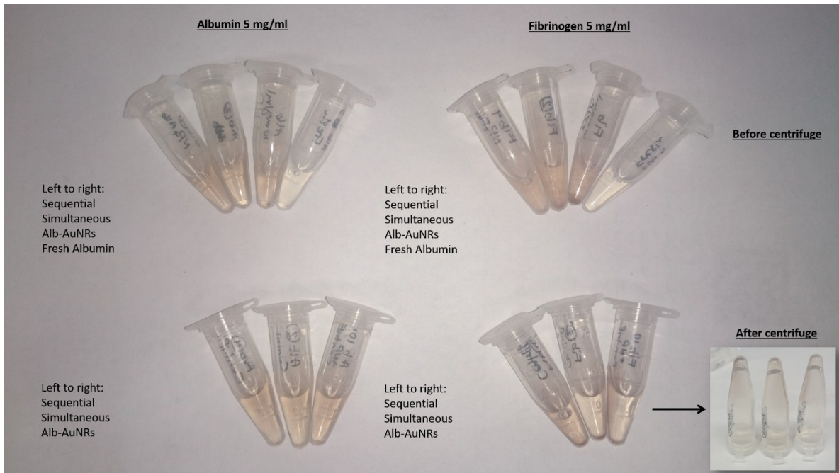
SI-Figure 3. Aggregation seen in some fibrinogen samples which resulted in adsorption of AuNRs onto microtube wall (observable in the inset in bottom right corner).
