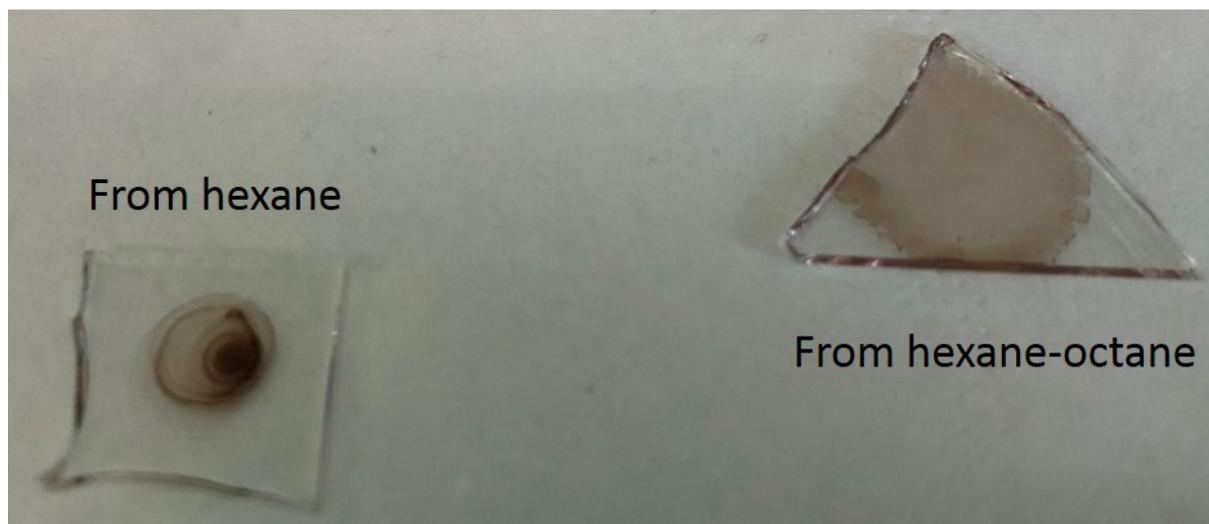
*Figure S 4 Image of dropcasted solution of HgTe/CdS from hexane solvent and from hexane:octane mixture.*
