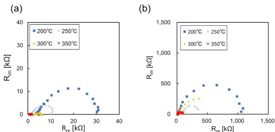
**Fig. S10** Nyquist plots (the relationship between real part  $R_{re}$  and imaginary part  $R_{im}$  of the frequency response) for films consisting of SDC10 (a) and SDC20 (b).
