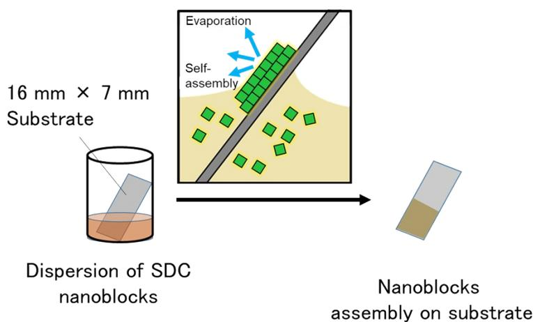
**Fig. S1** A schematic illustration of the fabrication system for thin films consisting of nanoblocks through evaporation-driven self-assembly using dispersion
