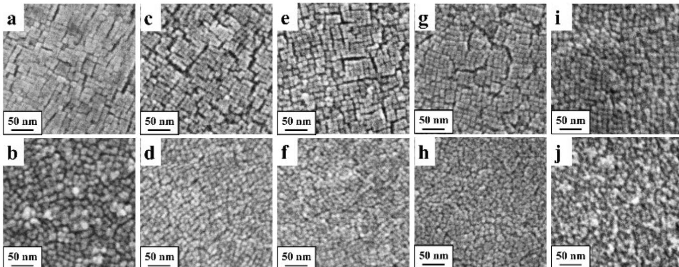
**Fig. S9** SEM images of thin films consisting of REDC nanoblocks prepared in the mother solution at  $[\text{Ce}^{3+}] : [\text{RE}^{3+}] = 9 : 1$  (upper row) and  $8 : 2$  (lower row). Dopant cations were (a, b)  $\text{La}^{3+}$ , (c, d)  $\text{Nd}^{3+}$ , (e, f)  $\text{Gd}^{3+}$ , (g, h)  $\text{Y}^{3+}$ , and (i, j)  $\text{Yb}^{3+}$ .
