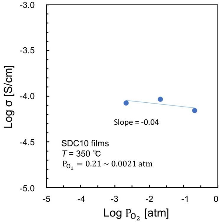
**Fig. S12** Dependence of electrical conductivity of SDC10 film on oxygen partial pressure.
