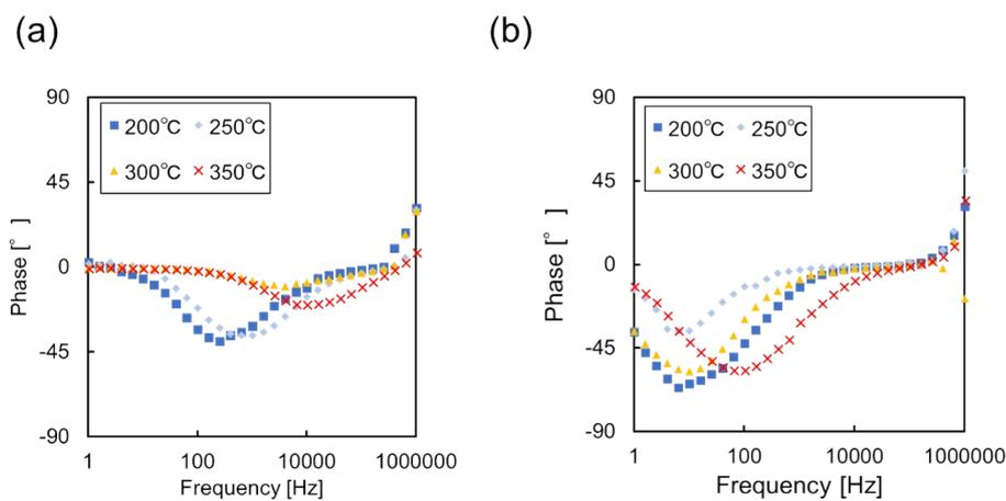
**Fig. S11** Bode plots (the phase shift as a function of frequency) for films consisting of SDC10 (a) and SDC20 (b).
