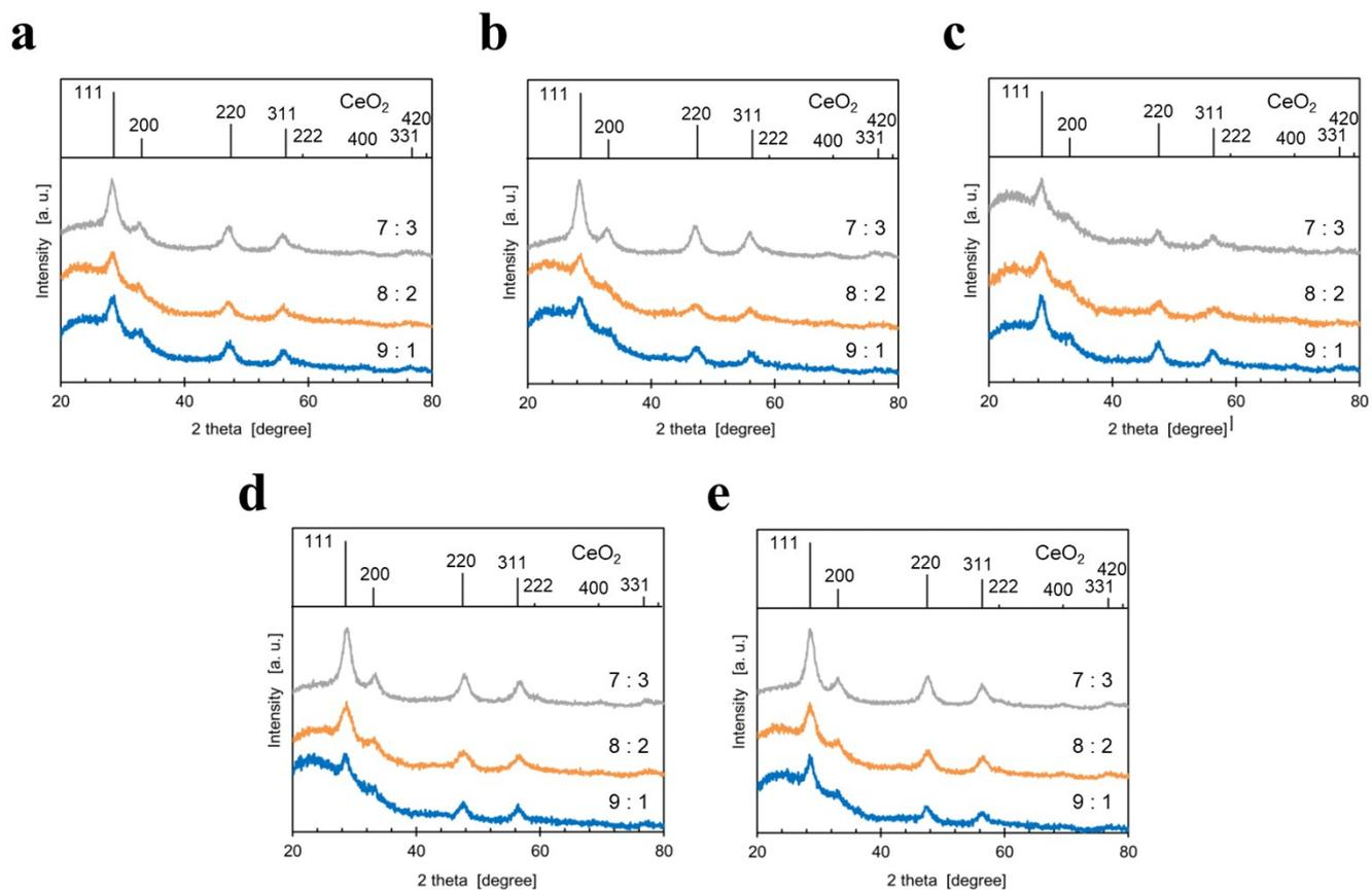
**Fig. S3** XRD profiles of REDC nanoblocks. Dopant cations were (a) La<sup>3+</sup>, (b) Nd<sup>3+</sup>, (c) Gd<sup>3+</sup>, (d) Y<sup>3+</sup>, and (e) Yb<sup>3+</sup>. The numbers represent the initial molar ratio of the dopant cations.
