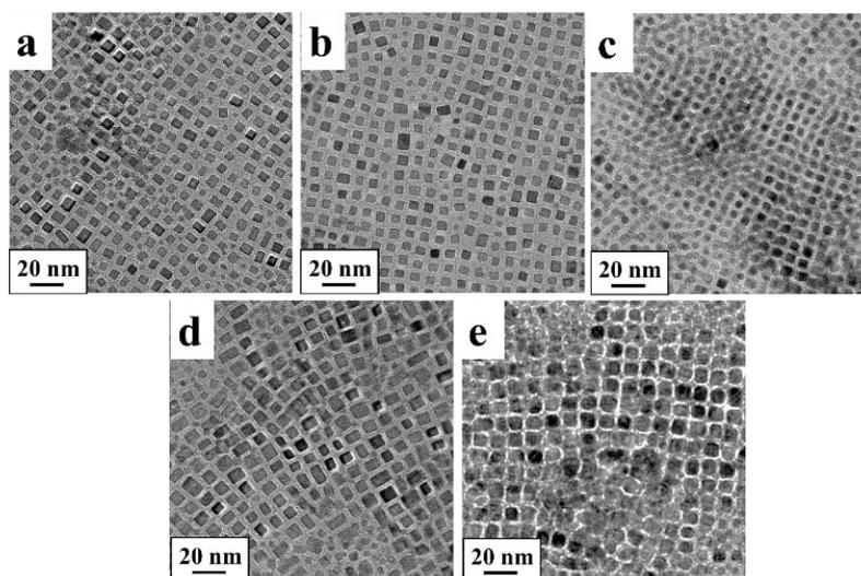
**Fig. S8** TEM images of REDC nanocubes prepared in the mother solution at  $[\text{Ce}^{3+}] : [\text{RE}^{3+}] = 9 : 1$ . Dopant cations were (a)  $\text{La}^{3+}$ , (b)  $\text{Nd}^{3+}$ , (c)  $\text{Gd}^{3+}$ , (d)  $\text{Y}^{3+}$ , and (e)  $\text{Yb}^{3+}$ .
