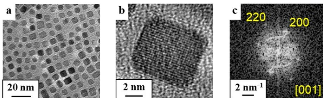
**Fig. S4** HRTEM images of CeO<sub>2</sub> nanocubes (a, b) and its FFT image (c) synthesized by the two phase solvothermal method.
