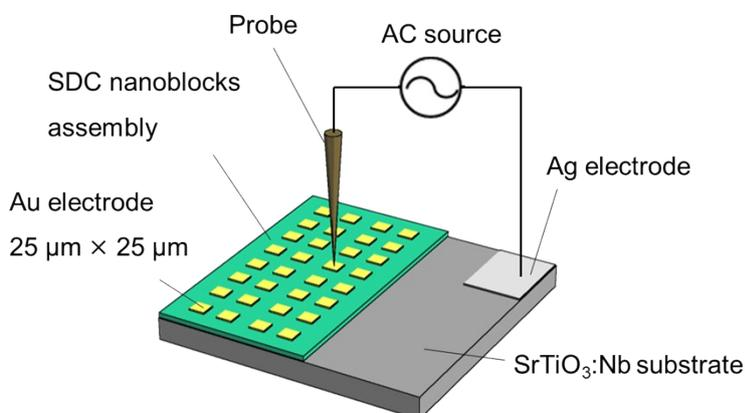
**Fig. S2** A schematic illustration of the measurement system for alternating current impedance of thin films. Film thickness of SDC10, SDC20, and SDC30 was 175, 231, and 86 nm respectively.
