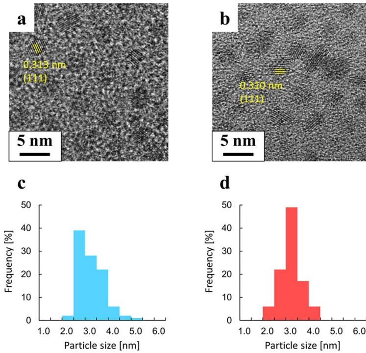
**Fig. S5** TEM images (a, b) and size distribution (c, d) of SDC nanoparticles in initial stage of reaction. (a, c) SDC10 and (b, d) SDC30.
