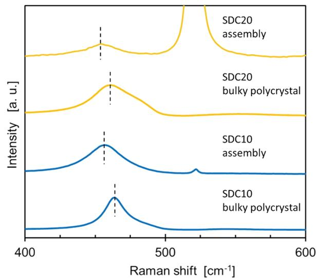
**Fig. S6** Raman scattering spectra of SDC nanoblocks assembly. The  $465\text{ cm}^{-1}$  peaks of the  $F_{2g}$  mode from the nanoblocks assembly were located at a wavenumber lower than those from bulky samples. The  $520\text{ cm}^{-1}$  peaks were attributed to the vibration of an Si substrate. Bulky polycrystals were obtained by calcination of pellets of the nanoblocks at  $1400^\circ\text{C}$ .
