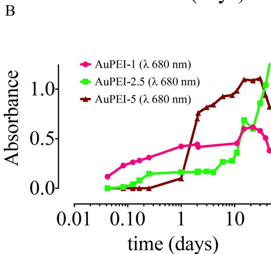
**Figure S2.** UV-visible light absorbance profile at different time points for H<sub>2</sub>AuCl<sub>4</sub> and PEI mixtures at [PEI]: [Au] ratios of 0.5 (A) and 10 (B). (C) Time evolution of primary LSPR for AuPEI-0.5 and AuPEI-10 nanocomposites.
