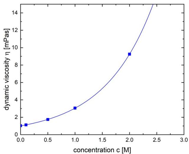
**Fig. S4** Evolution of viscosity of the MAPbBr<sub>3</sub> precursor fluid with increasing concentration.
